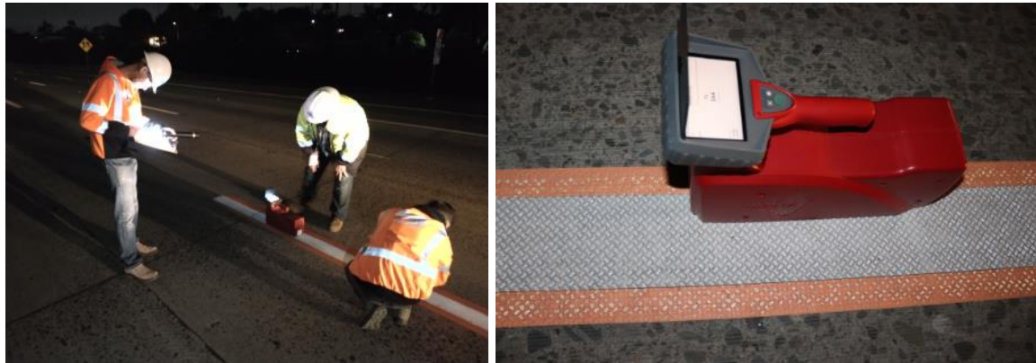
Figure 4.2: Left: Striping quality measurements performed by AHMCT researcher and Caltrans staff days after orange striping installation; Right: Retroreflectivity and nighttime color measurements on tape striping on I-5, northbound traffic, south of Las Flores Overcrossing
