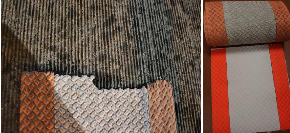
Figure 4.17: Tape on freeway concrete surface with grinding grooves (left); Orange tape striping worn (at 5 months) and new
