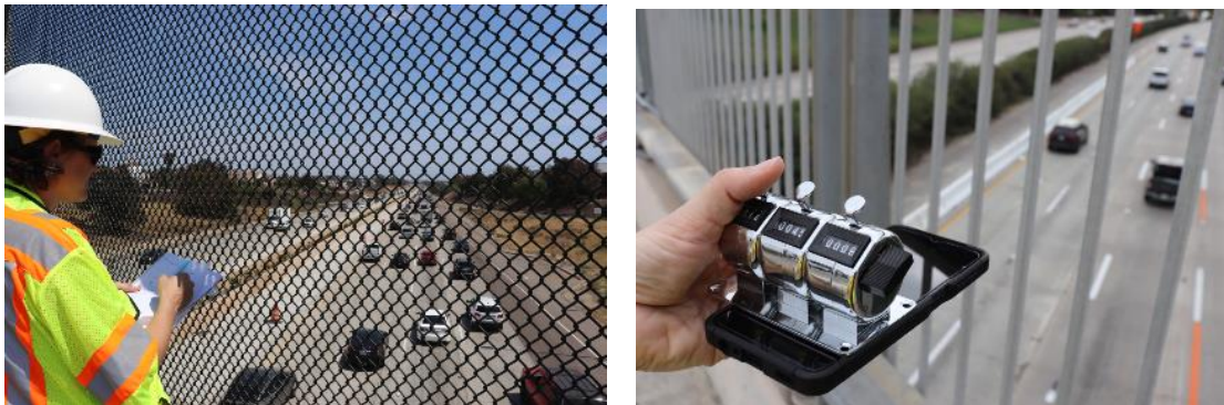
Figure 2.1: Left: Visual observation of driver lane keeping on Palomar Airport Rd Overcrossing over I-5, south view on SB traffic. Right: Using the three-part clicker for recording and smartphone as timer on Las Flores Overcrossing over I-5, south view on SB traffic.
