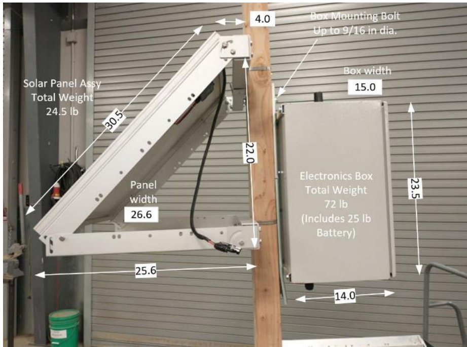
Figure A1.4: Solar panel and electronics box installation
