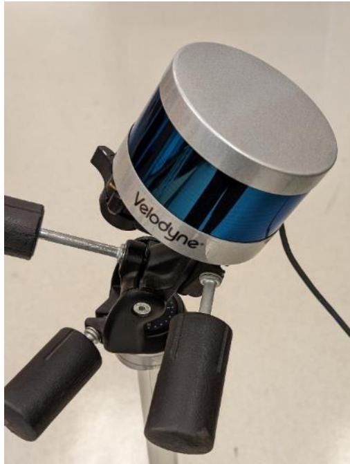
Figure A2.1: Velodyne VLP16 LiDAR sensor with a 30 degree tilt from horizontal
