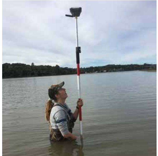
Image 1: Determining precise elevation of pressure sensors deployed.
