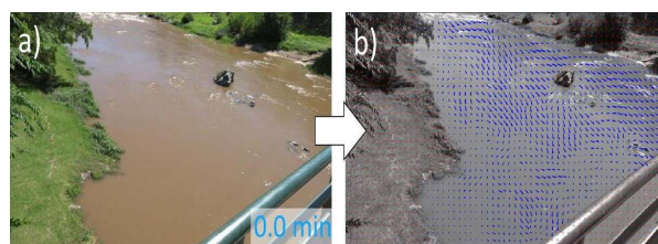
Figure 3: Results of LSPIV analysis process for a flash-flood event on a river.
