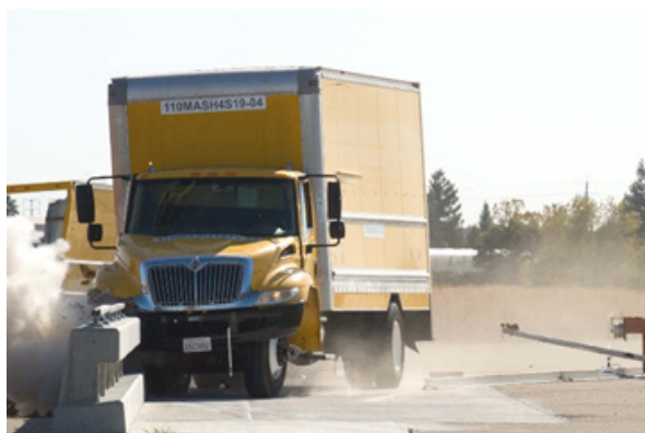
Image 5: Type 85 Bridge Rail: Van Body Impact
