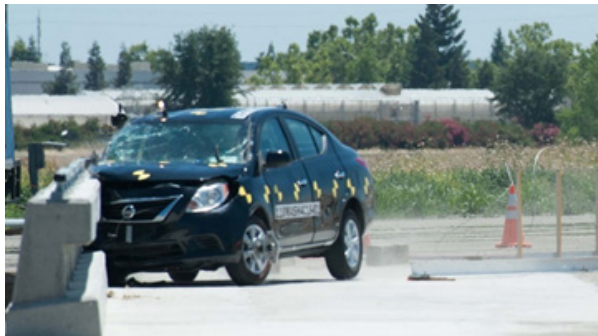
Image 3: Type 85 Bridge Rail: Small Car Impact
