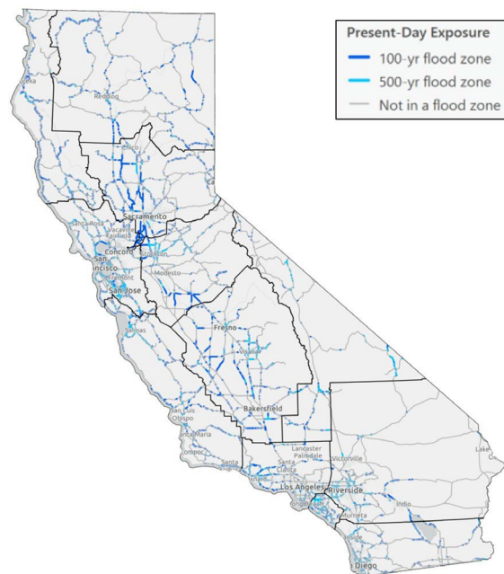
Figure 6 Exposure of the SHS to present-day riverine flooding.
