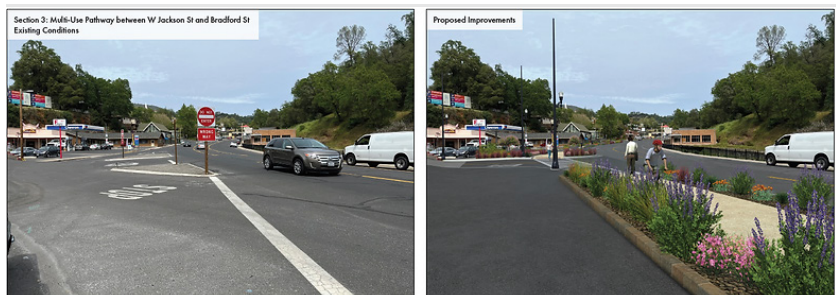
Existing conditions of an intersection on this project corridor and the proposed path concept design.
