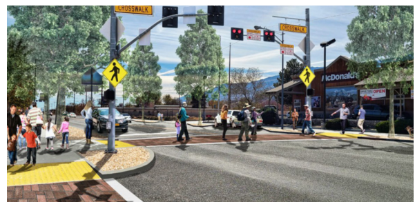
Conceptual design of the crosswalk enhancements, bulbouts, and RRFB
