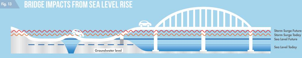
Climate change can impact infrastructure in multiple ways. Bridges in the Delta, for example, can be directly impacted by rising sea levels and storm surge effects. Today's bridges were designed and built for current tidal and surge conditions, so increasing water levels may increase the risk for these facilities in the future.
