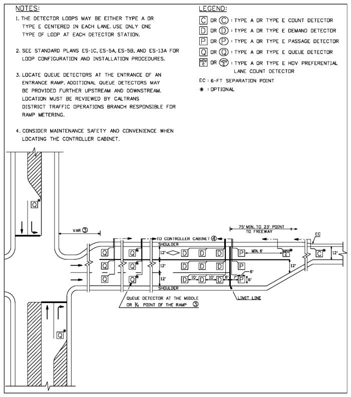
Figure 2-10 Typical Detector Layout for an Exit Ramp
