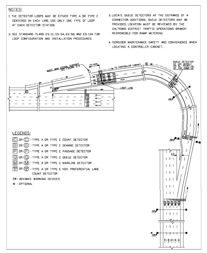
Figure 2-12 Typical Advance Warning Devices
