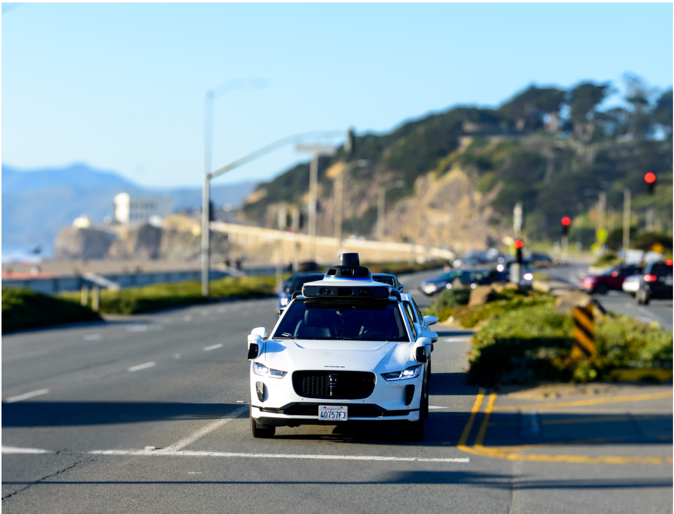
Photo 1: Driverless car equipped with LiDAR sensors and cameras. Editorial credit: Michael Vi / Shutterstock.com.
