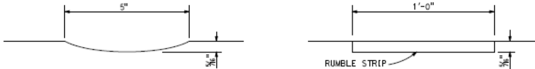
Figure 2: Detail of standard rumble strip
