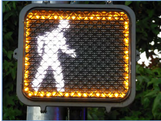
Figure 2 – Final prototype module with 1-inch LED spacing.
