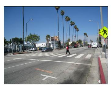
The Santa Monica Boulevard/Princeton Street test consists of marked а crosswalk on Santa Monica Boulevard the across uncontrolled eastern leg of the intersection. Santa Monica Boulevard is a Principal Arterial. Stop controls are provided on Princeton Street, the minor side street approaches to Santa Boulevard. Monica The Final Report
