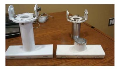
The modified mounts are affixed to a standard terminal block, and allow the RRFB housings to be angled towards or away from the roadway, and rotated from top to bottom.
