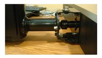
Below is an image of the finished modification, with the terminal block holding two RRFB housings, to face each direction of oncoming traffic.
