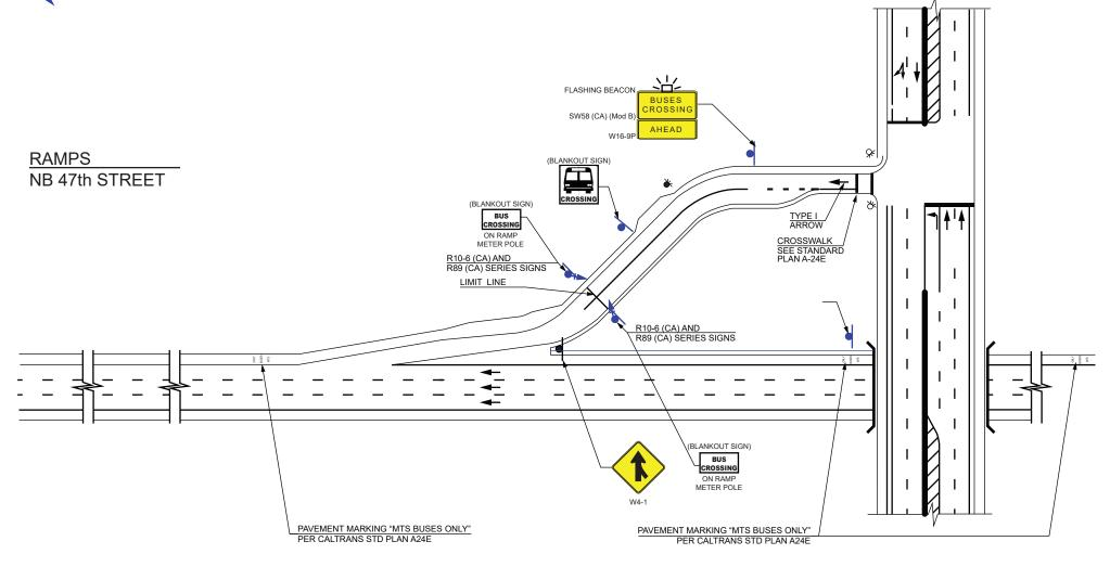
PROPOSED TYPICAL SIGNING AND PAVEMENT MARKING BASED ON FIGURE 3-2 OF CALTRANS RAMP METER DESIGN MANUAL
