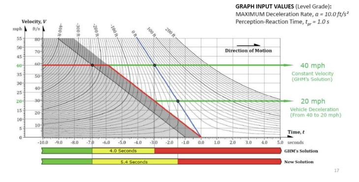
Assuming the variables above, the minimum yellow interval would be 5.4 sec. The current yellow interval is 3.0 sec., 2.4 seconds too short. Drivers routinely encounter a dilemma zone. The pattern of violations at this intersection shows the problem.
