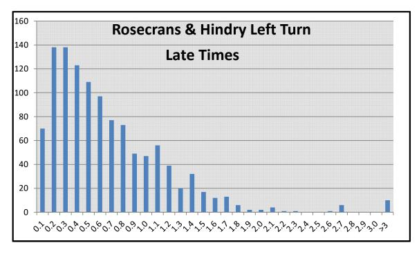
Note that almost all violations at this intersection occur in the 2.4 second range, exactly the time difference between the current yellow interval of 3.0 sec, and the calculated minimum yellow interval of 5.4 sec. arrived at using the extended solution.
