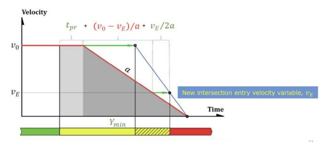
To calculate the time to cross the critical distance, add the perception-reaction time to the time to slow down to the entry speed, plus the time to continue at that speed into the intersection.
