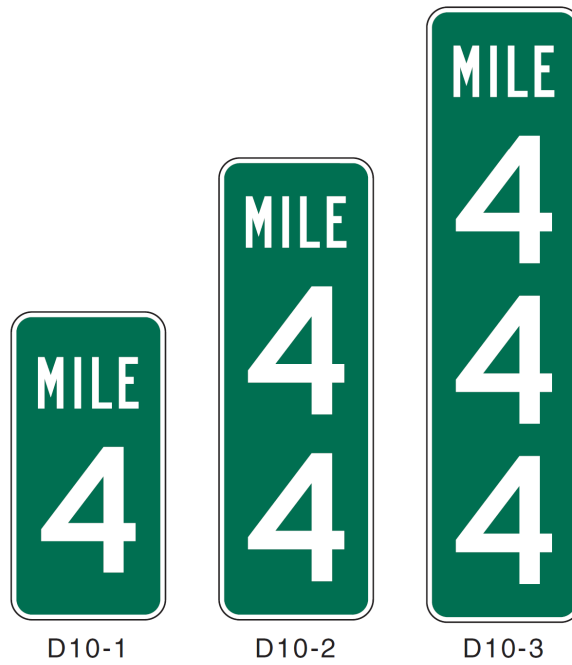
Figure 2H-2. Reference Location Signs
