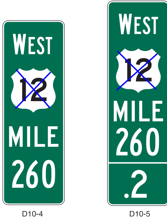
Figure 2H-4. Enhanced Reference Location Signs
