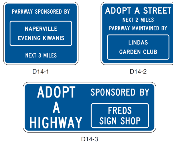
Figure 2H-5. Examples of Acknowledgment Sign Designs
