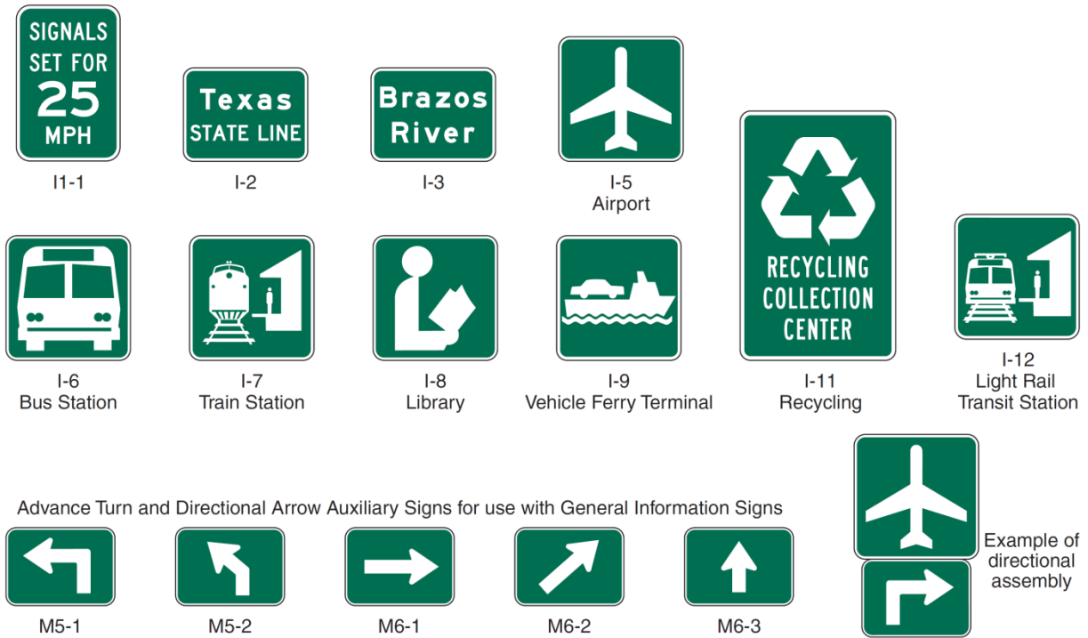
Figure 2H-1. General Information and Miscellaneous Information Signs
