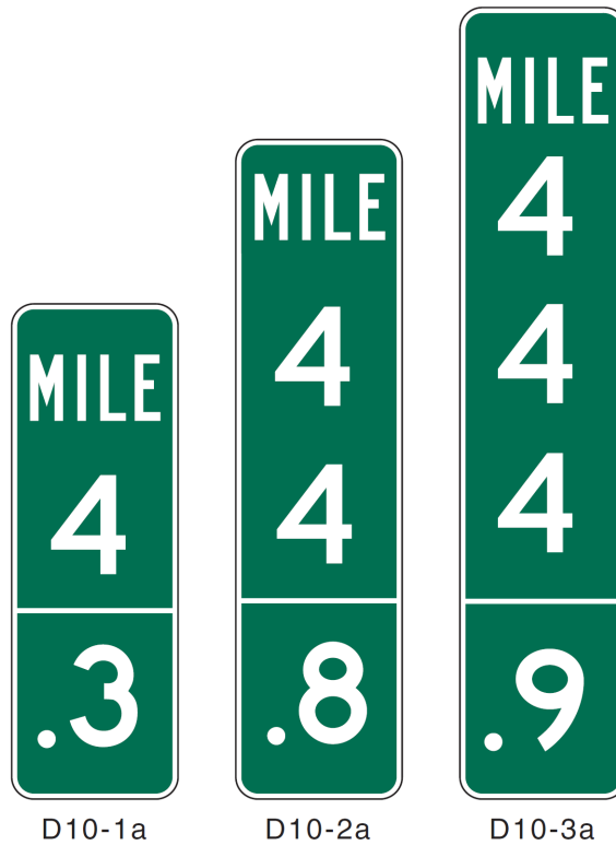
Figure 2H-3. Intermediate Reference Location Signs
