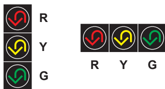
Figure 4E-1. Typical Arrangements of U-Turn Signal Faces
