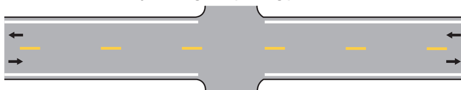
Figure 3B-1. Yellow Center Lines for Two-Lane, Two-Way Applications
