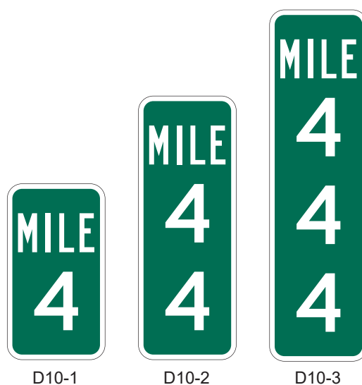
Figure 2H-5. Reference Location Signs
