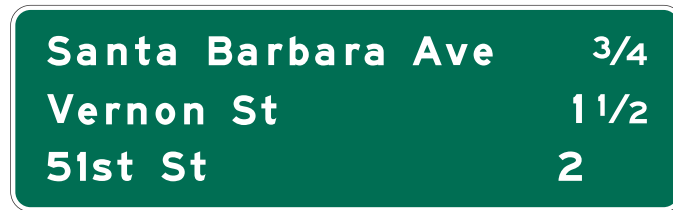
Figure 2E-10. Example of an Interchange Sequence Sign
