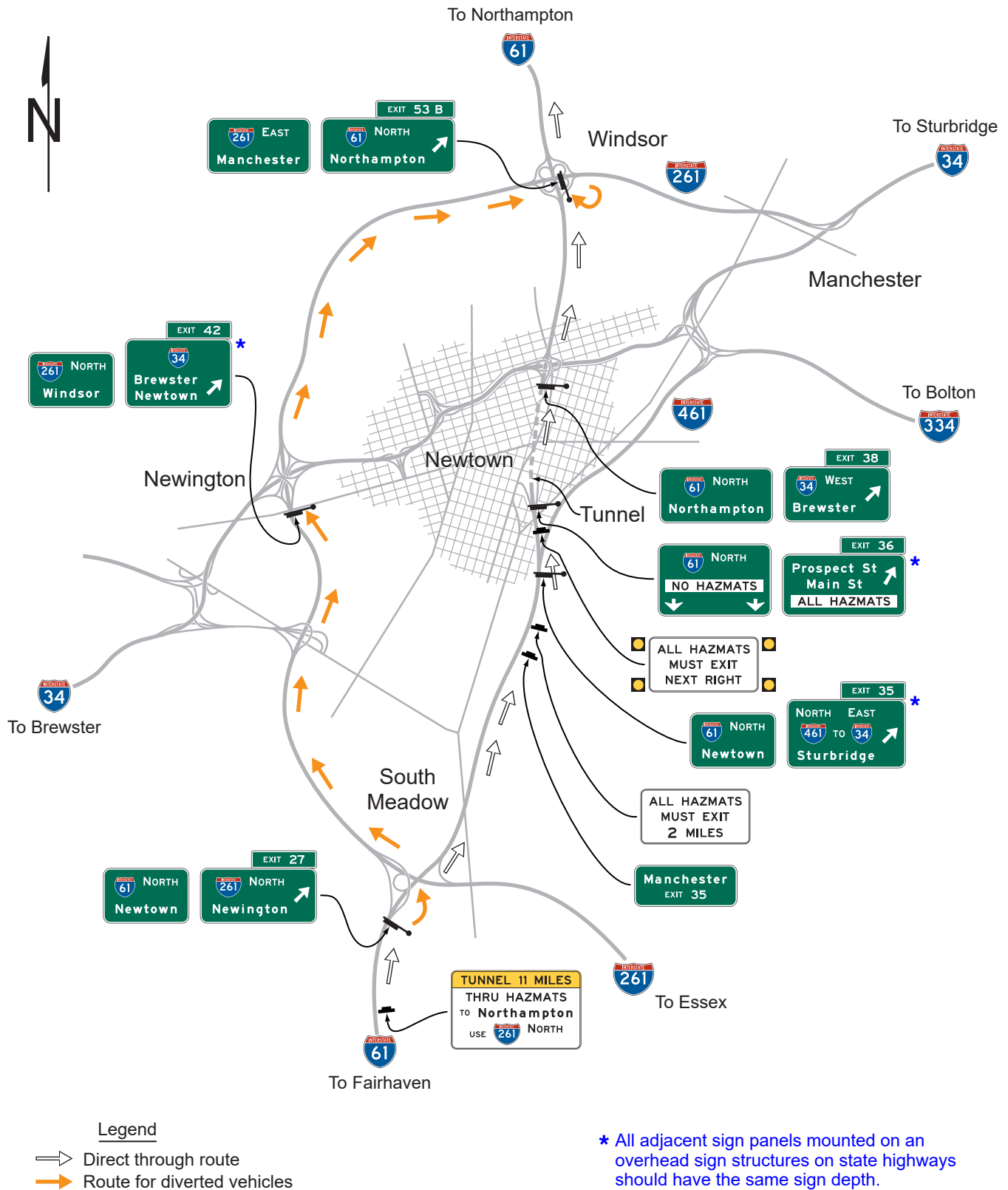
Figure 2E-62. Example of Signing for Route Diversion by Vehicle Class
