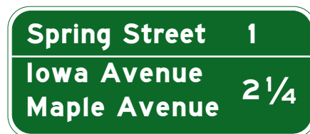
Figure 2E-10(CA). California Example of an Interchange Sequence Sign
