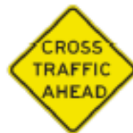
Figure 2C-9 (CA). Intersection Warning Signs and Plaques
