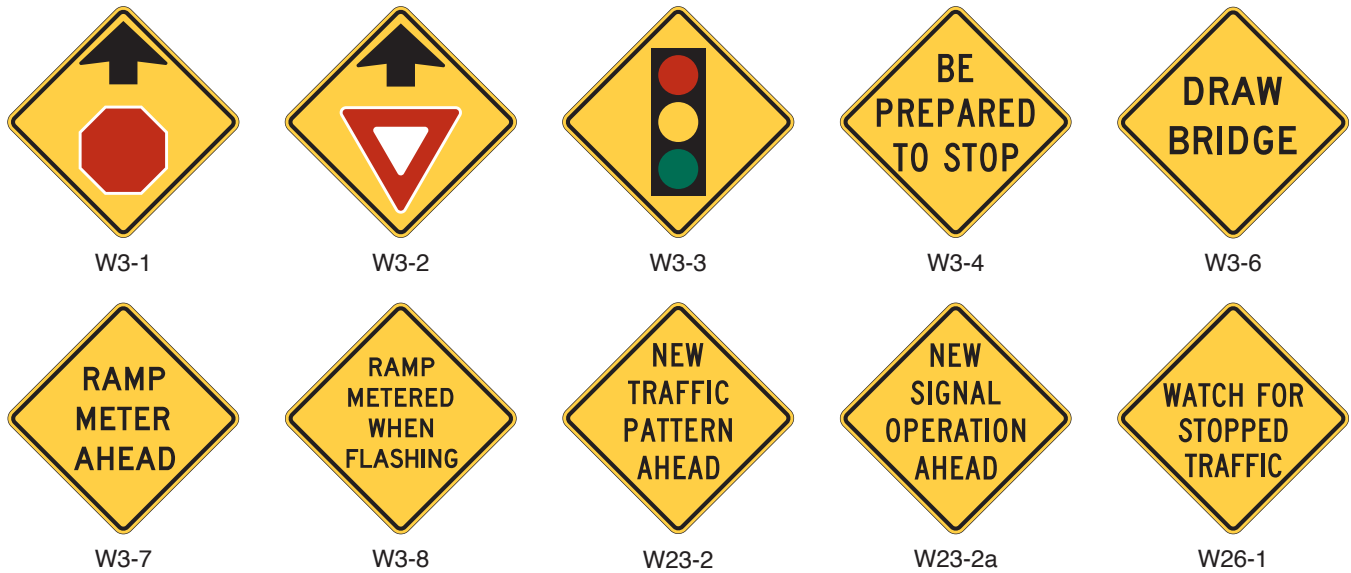
Figure 2C-8. Advance Traffic Control Signs
