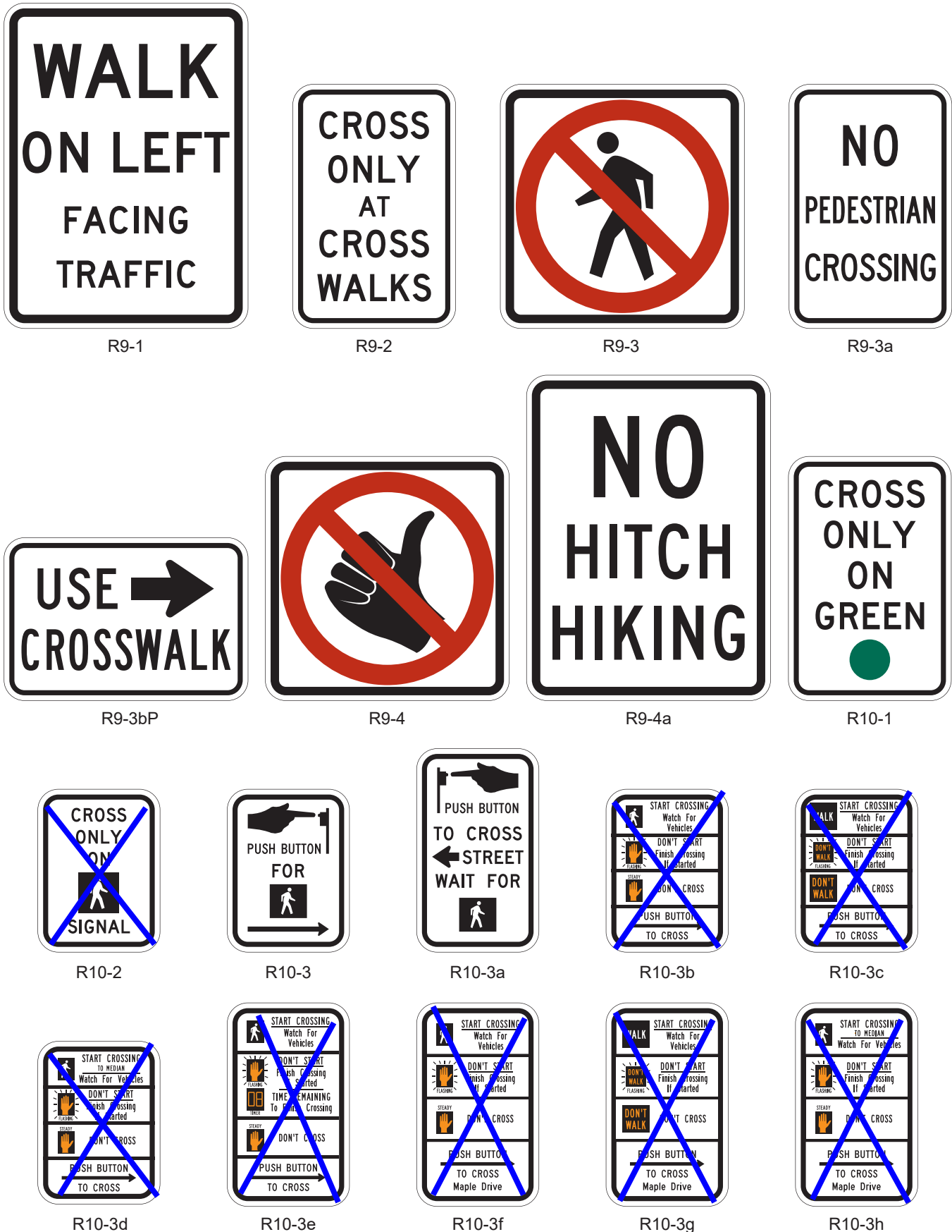
Figure 2B-27. Pedestrian Signs and Plaques (Sheet 1 of 2)
