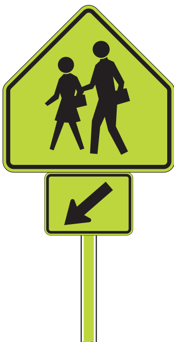
C) RMS-3(CA) Fluorescent Yellow-Green vertical retroreflective strip on pedestrian, bicycle, and school zone sign supports
