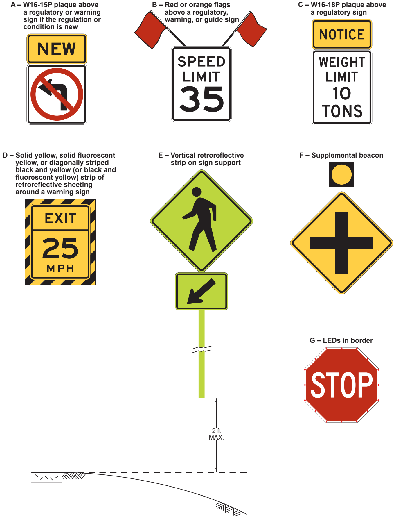
Figure 2A-1. Examples of Enhanced Conspicuity for Signs
