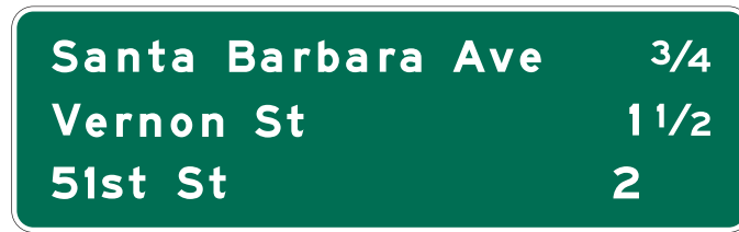
Figure 2E-10. Example of an Interchange Sequence Sign
