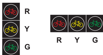
Figure 4H-1. Typical Arrangements of Bicycle Signal Faces
