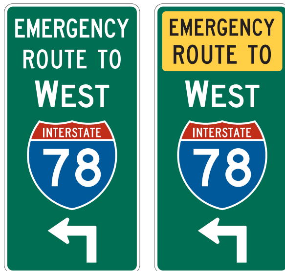
Examples of guide signs for rerouting
