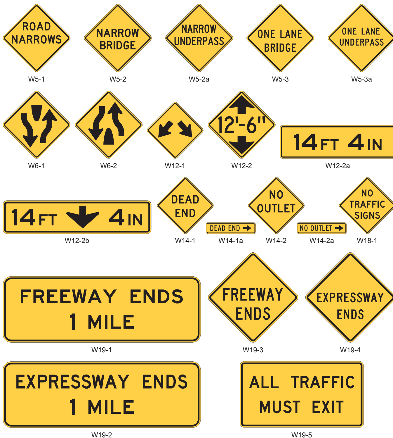
Figure 2C-6. Miscellaneous Warning Signs
