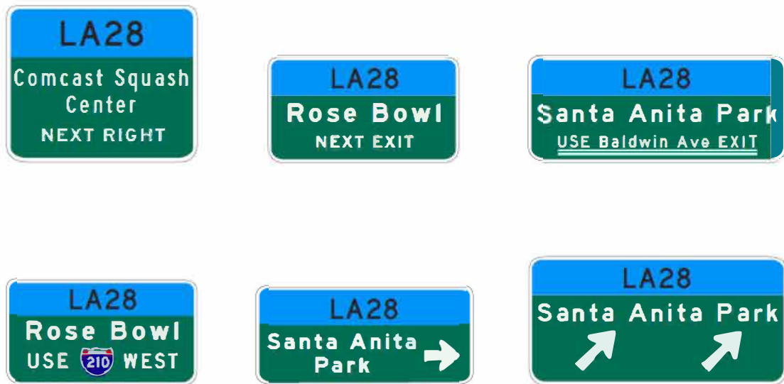
Figure 2D-9(CA)(LA28). LA28 Sign Panel on Destination Signs
