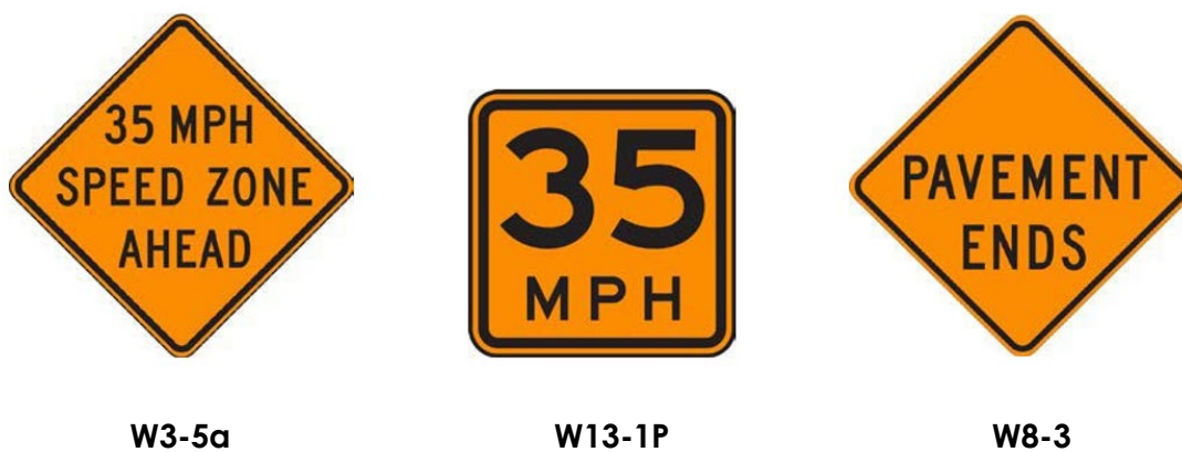
Figure 2-6 Temporary Traffic Control Advisory Signs
