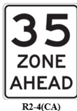
Figure 4-2 Reduced Speed Zone Ahead
