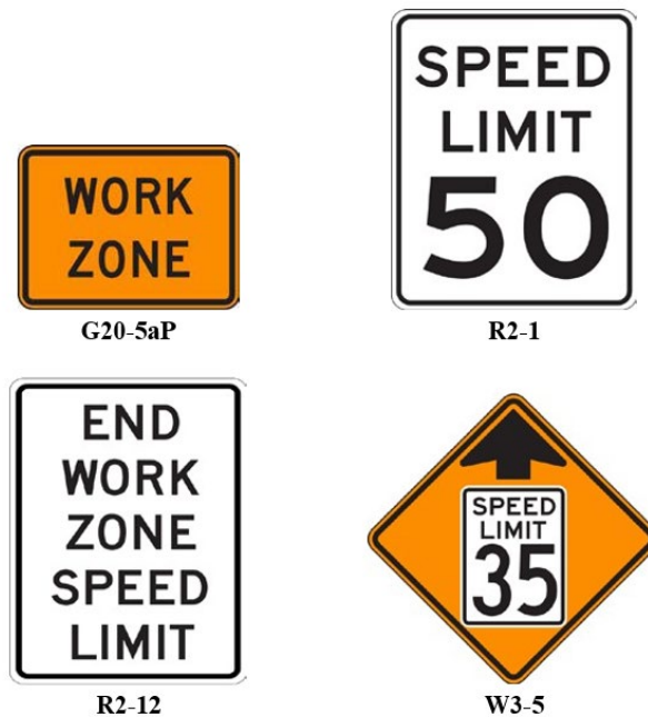
Figure 2-7 Temporary Traffic Control Regulatory Signs
