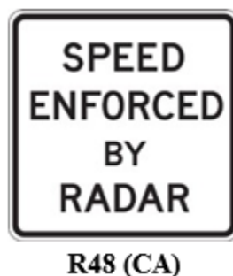
Figure 4-5 Speed Enforced by Radar
