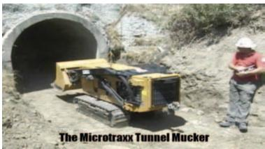
The Microtraxx Tunnel Mucker is a radio remote-controlled front end loader. The Mucker allows safe and easy access to box culverts and ditches for cleaning purposes. These areas can otherwise be hazardous or difficult to access.
