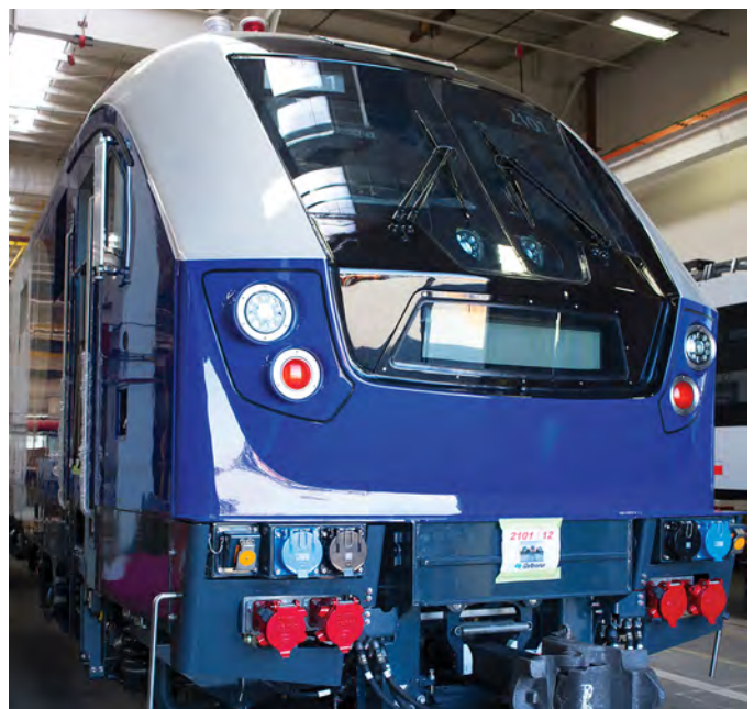
The front of this locomotive is closer to completion as lights and electrical hookups are added.
