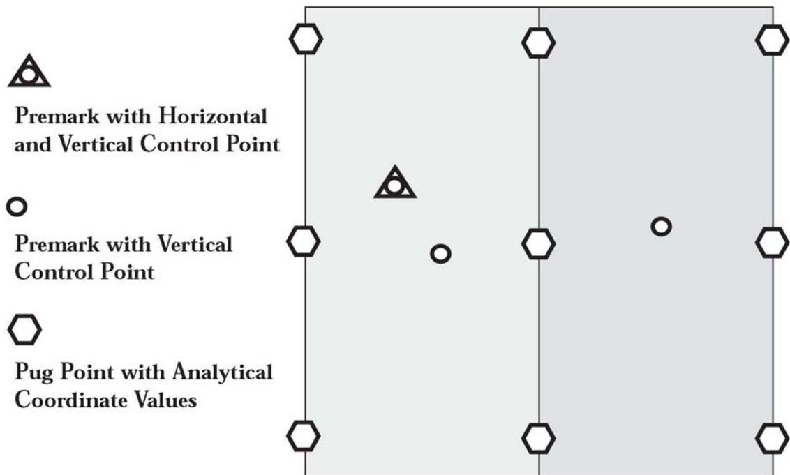
These points can be either traditional pre-marked targets or analytic points produced by the aerotriangulation process.
