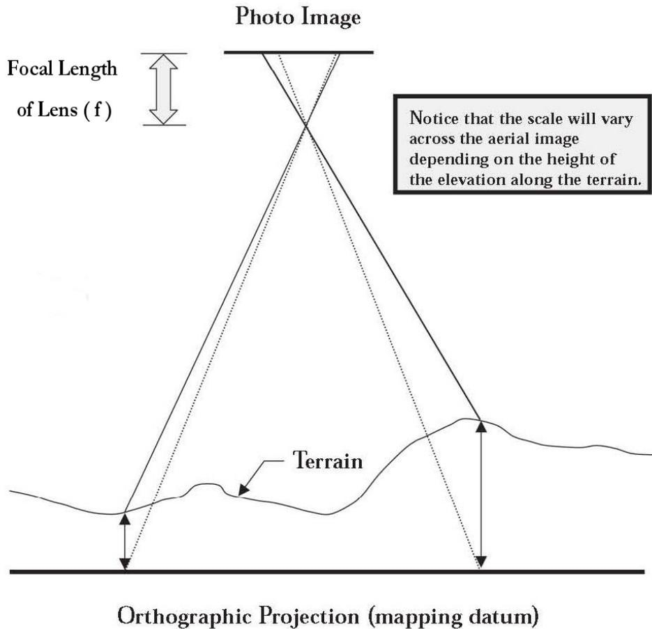
As you see, the shorter the distance between the ground and the camera the larger the scale of the photograph at that point. The result is greater ground resolution and the potential for increased accuracy, however the coverage is reduced, increasing the number of photographs and ground control required for
