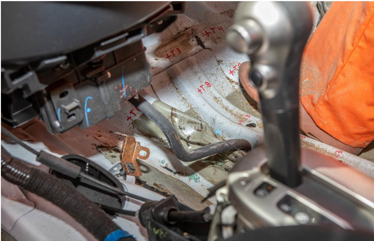
Figure 5-21 Test 4-10 Floorboard Deformation
