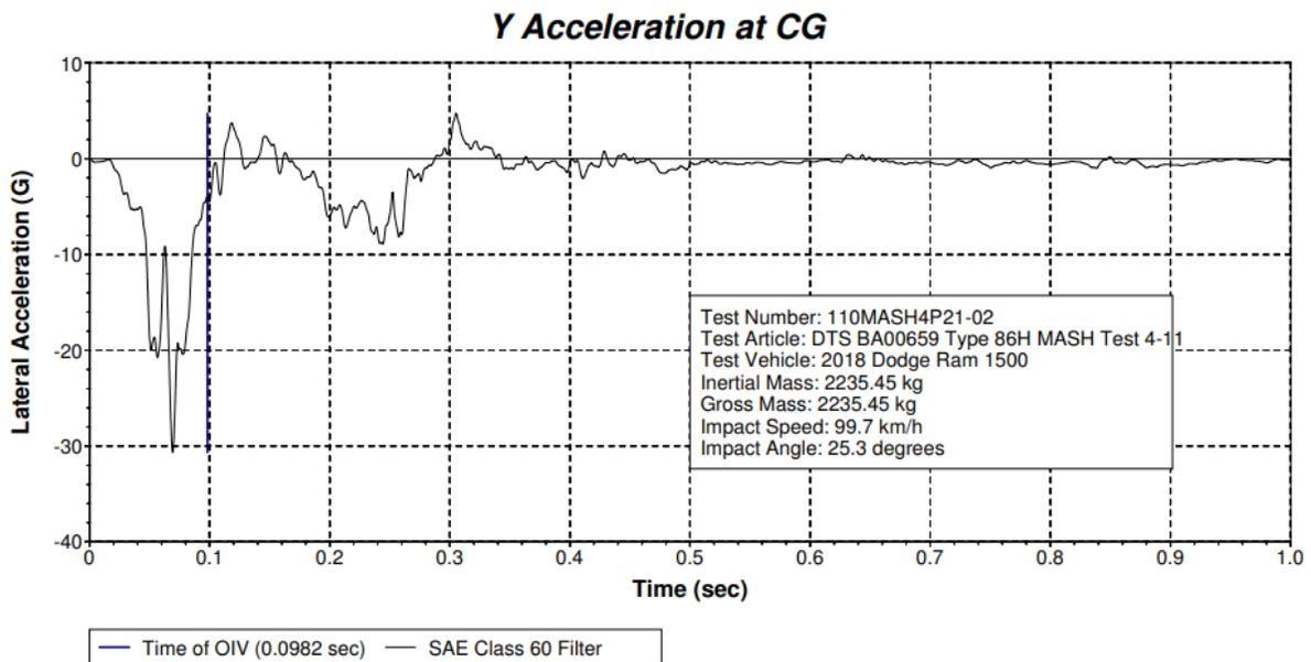
Figure 10-39 Test 4-11 Lateral Acceleration (DTS SLICE Micro TRAP BA00659)
