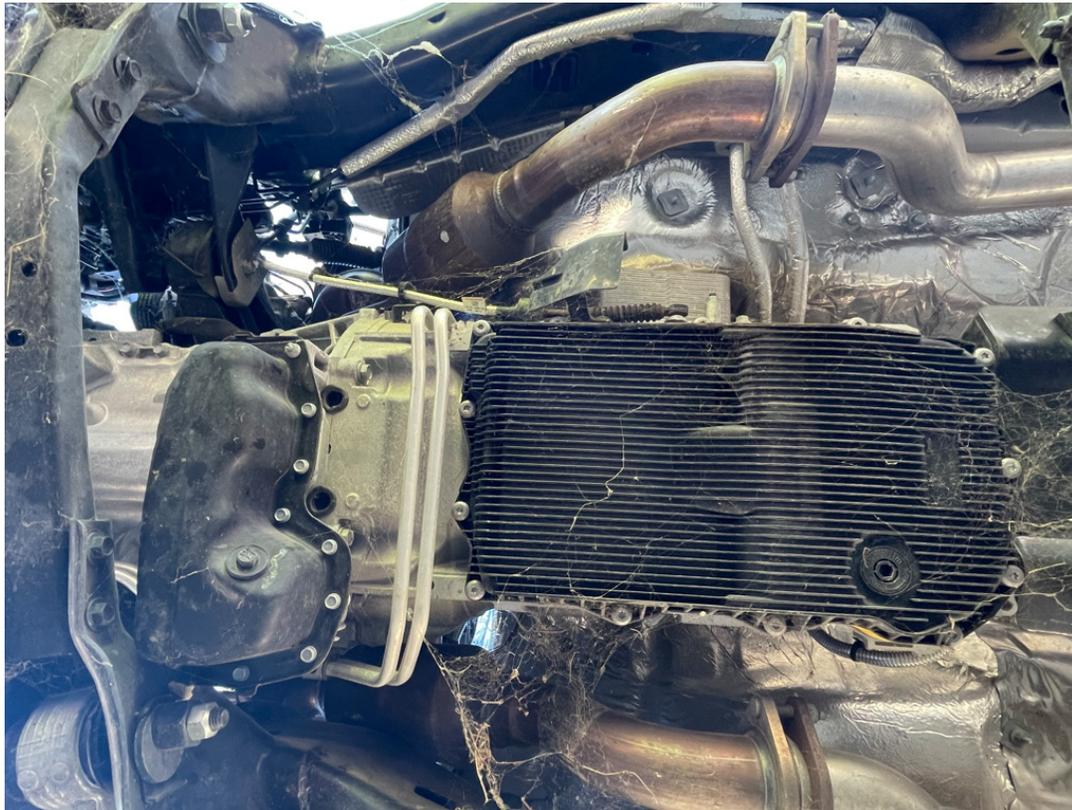
**Figure 13-4 Undamaged Oil Pan for the 2270P Pick Up Truck**
