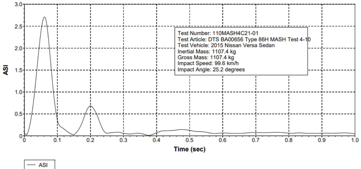
Figure 10-36 Test 4-10 Acceleration Severity Index (DTS SLICE Micro TRAP BA00656)
