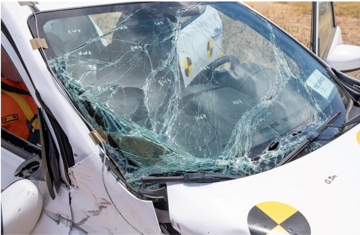
Figure 5-17 Test 4-10 Test Vehicle Damage Windshield / Exterior
