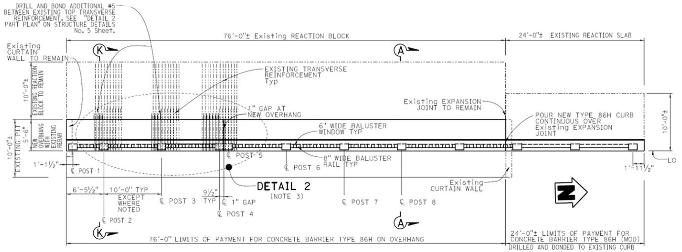
Figure 2-4 Plan View of Type 86H Test Article
