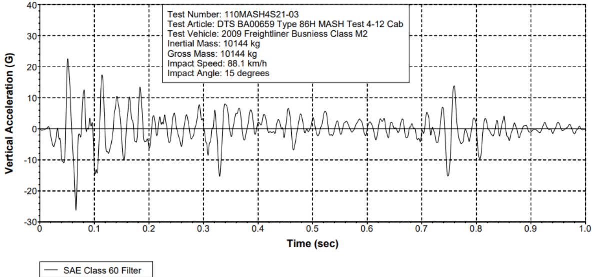
Figure 10-61 Test 4-12 Vertical Acceleration (DTS SLICE Micro TRAP BA00659)
