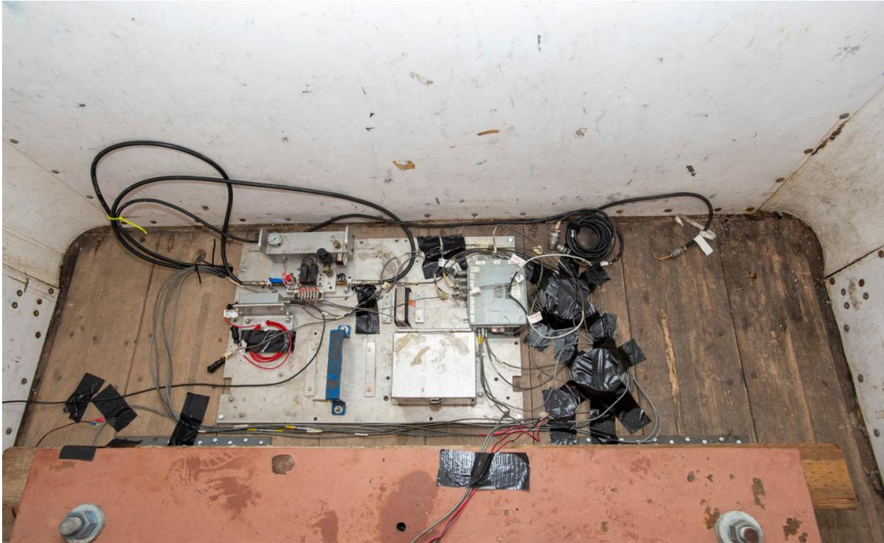
**Figure 4-22 MASH 4-12 Test Vehicle Instrumentation Equipment in Cargo Box**
