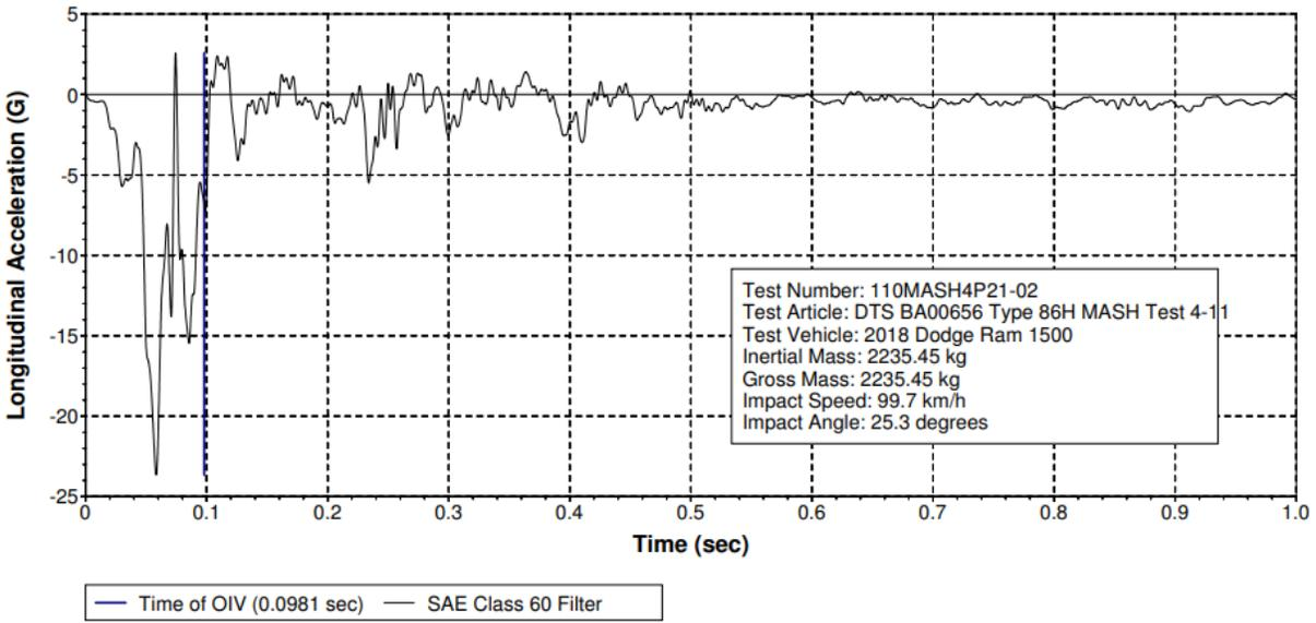
Figure 10-45 Test 4-11 Longitudinal Acceleration (DTS SLICE Micro TRAP BA00656)
