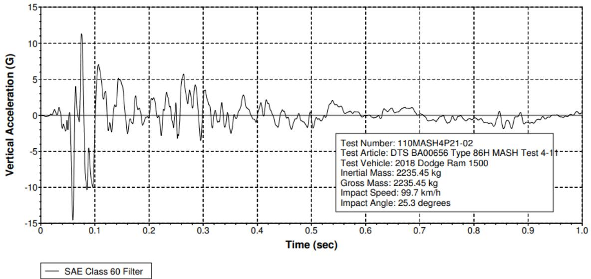
Figure 10-47 Test 4-11 Vertical Acceleration (DTS SLICE Micro TRAP BA00656)
