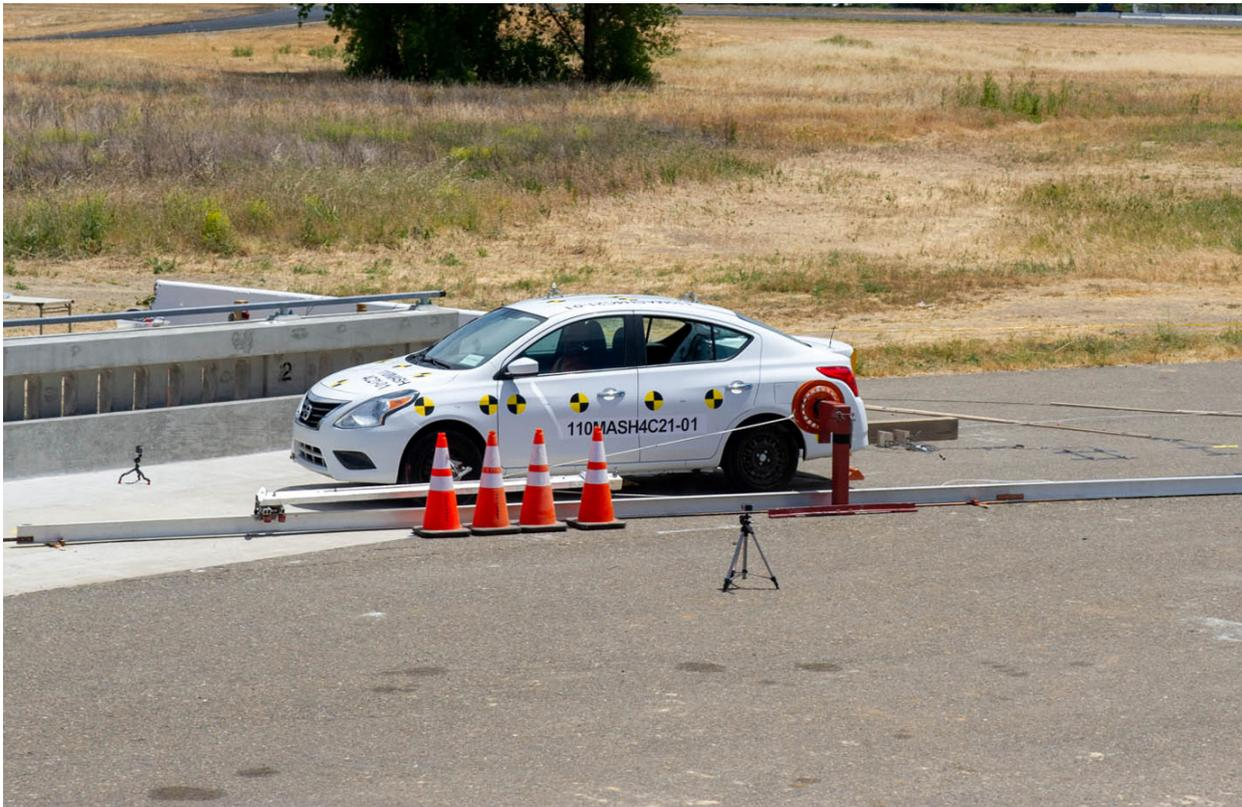
**Figure 10-10 Guide Arm Released from Vehicle**
