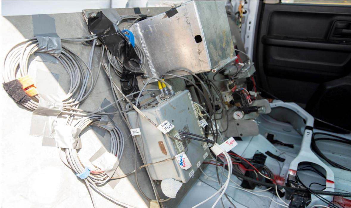
**Figure 10-3 Test 4-11 Vehicle Instrumentation**
