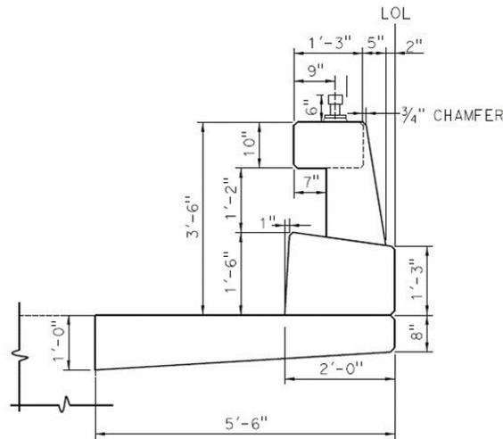
Figure 1-4 Type 86H Concrete Post and Beam Barrier Rail (MASH TL-4)
