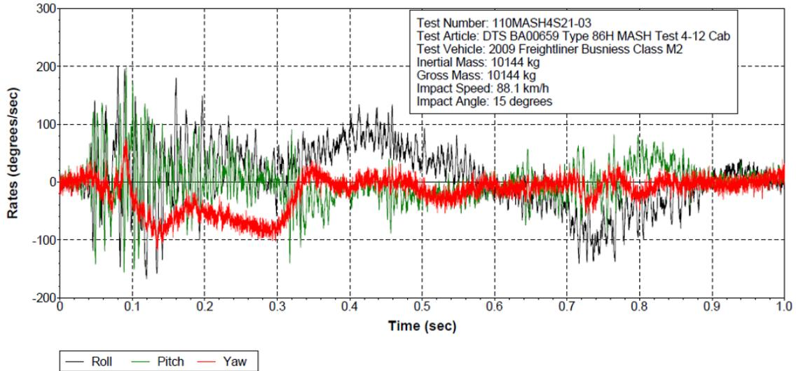
Figure 10-62 Test 4-12 Roll, Pitch, and Yaw Rates (DTS SLICE Micro TRAP BA00659)
