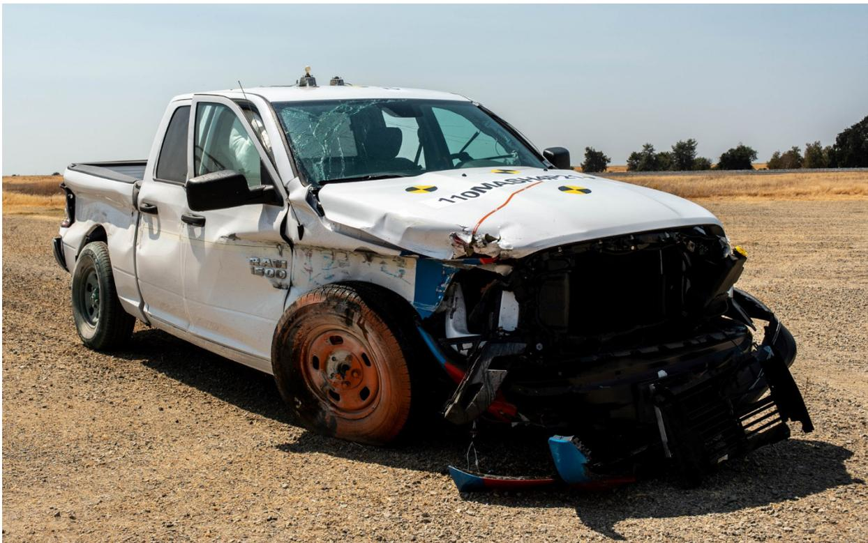
Figure 6-11 Test 4-11 Test Vehicle Damage (front right)
