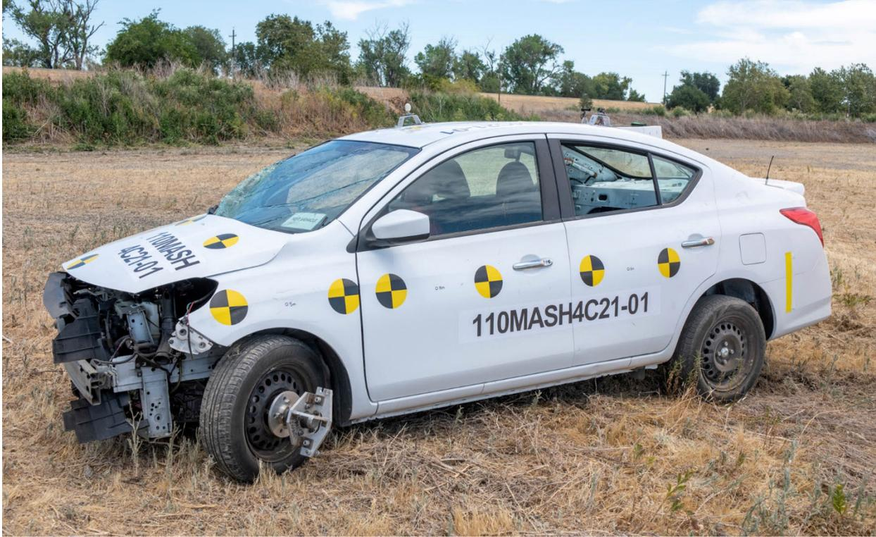
Figure 5-14 Test 4-10 Test Vehicle Damage (front left)
