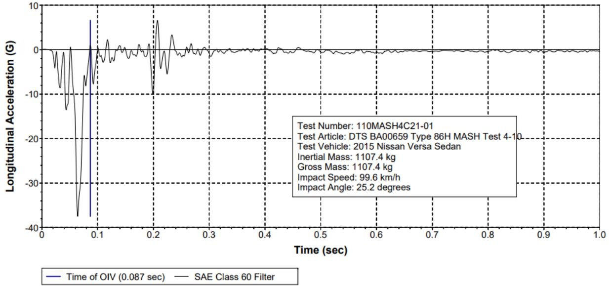
Figure 10-24 Test 4-10 Longitudinal Acceleration (DTS SLICE Micro TRAP BA00659)
