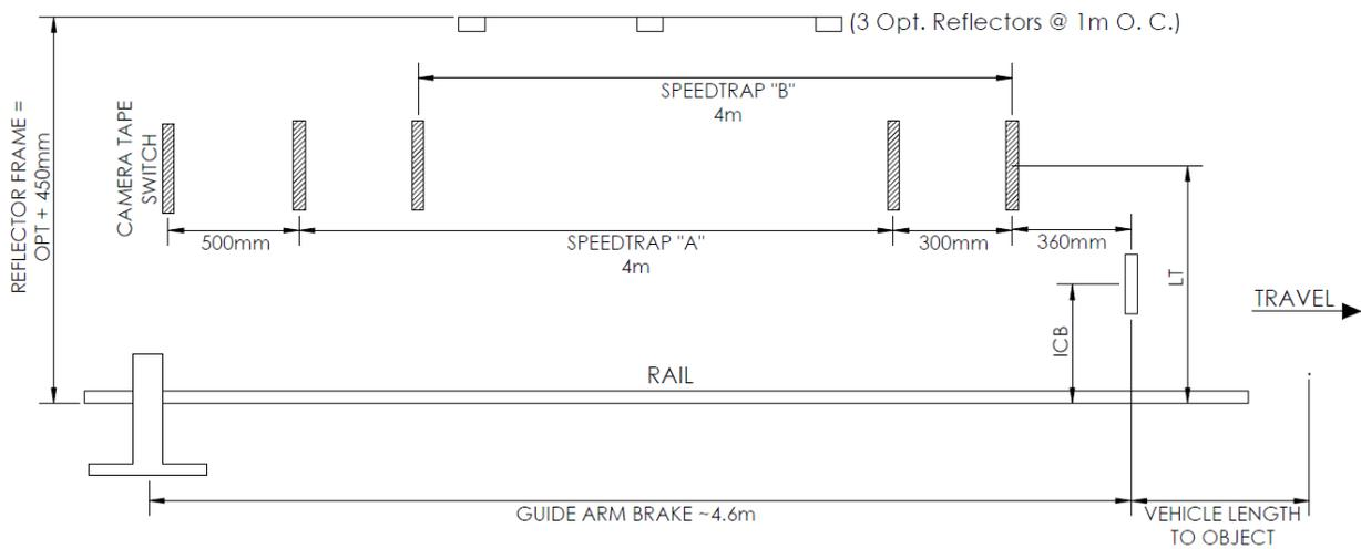
Figure 10-16 Speed Trap Tape Layout
