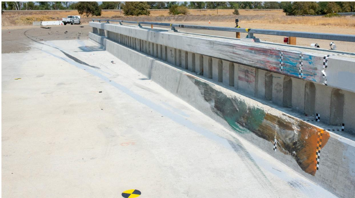
Figure 6-9 Test 4-11 Type 86H Overview of Barrier Post-Test with Tire Marks (view looking downstream)
