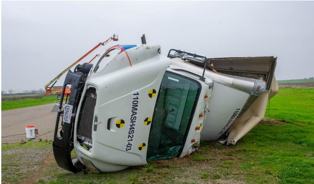
Figure 7-13 Test 4-12 Vehicle Damage (front, hood and windshield)
