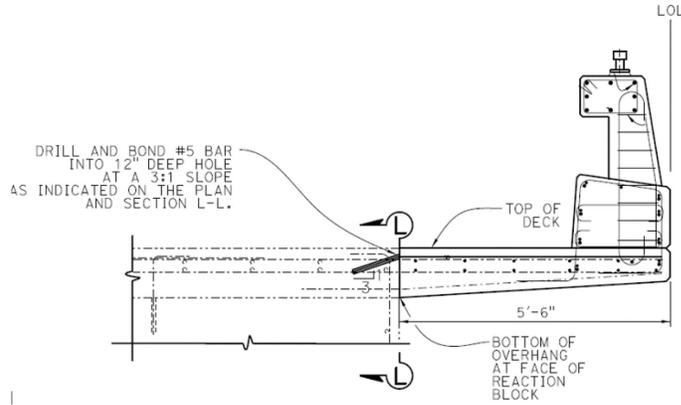
Figure 2-3 Partial Cross Section of New Overhang with the Type 86H Barrier Rail
