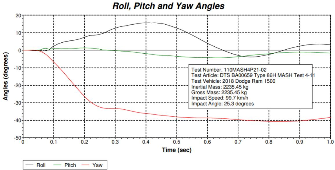
Figure 10-42 Test 4-11 Roll, Pitch, and Yaw Angles (DTS SLICE Micro TRAP BA00659)
