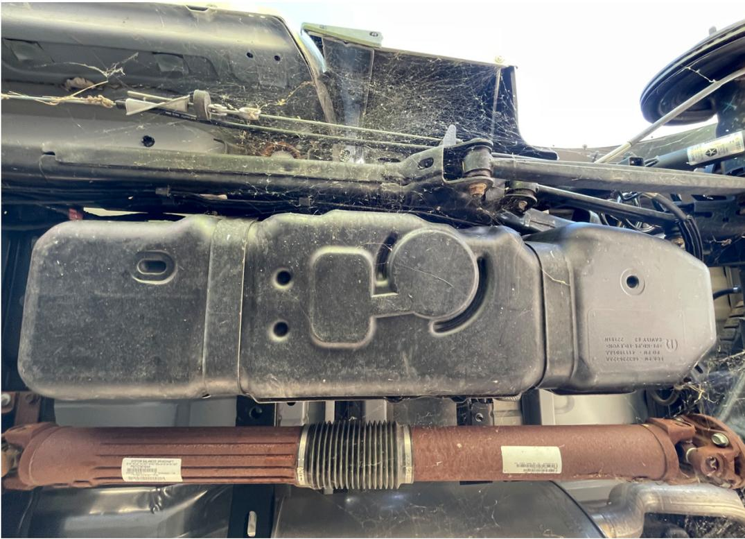
**Figure 13-3 Undamaged Gasoline Tank for the 2270P Pick Up Truck**
