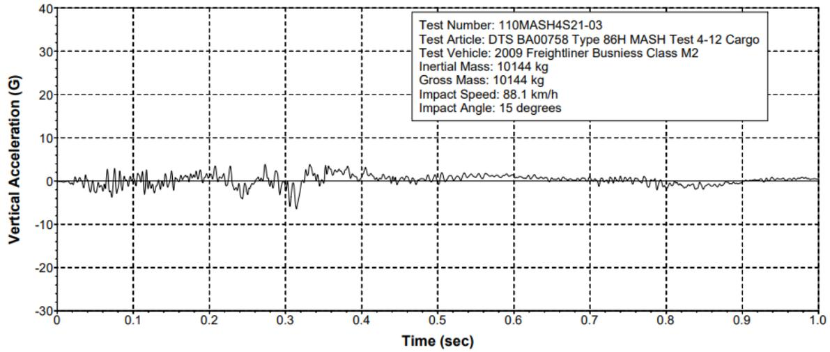
Figure 10-68 Test 4-12 Vertical Acceleration (DTS SLICE Micro TRAP BA00758)
