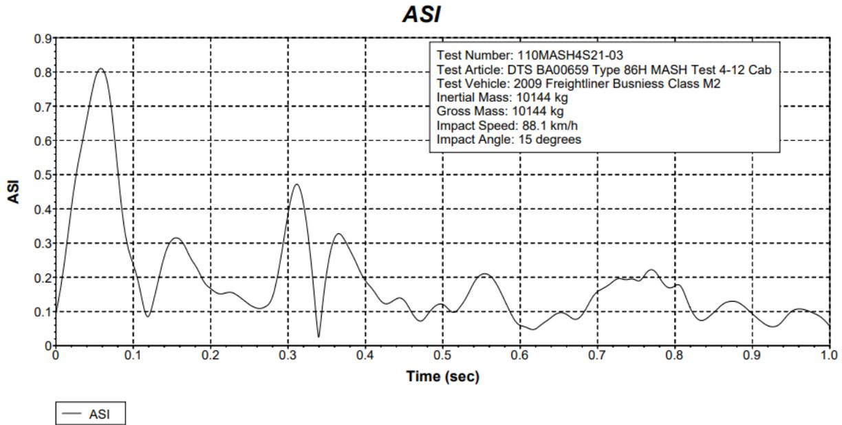
Figure 10-64 Test 4-12 Acceleration Severity Index (DTS SLICE Micro TRAP BA00659)
