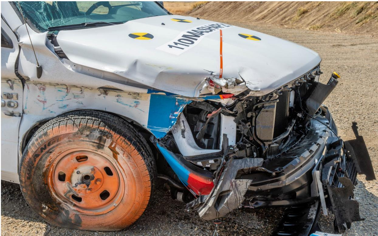
Figure 6-13 Test 4-11 Test Vehicle Damage (front right)
