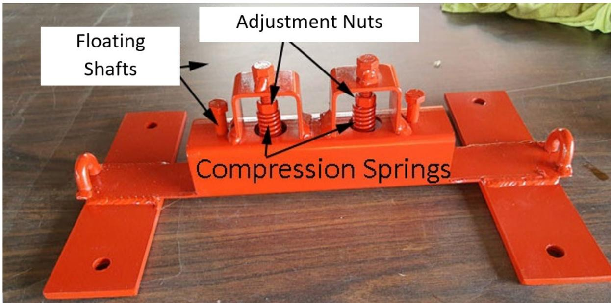
Figure 10-12 Friction Brake Close Up View
