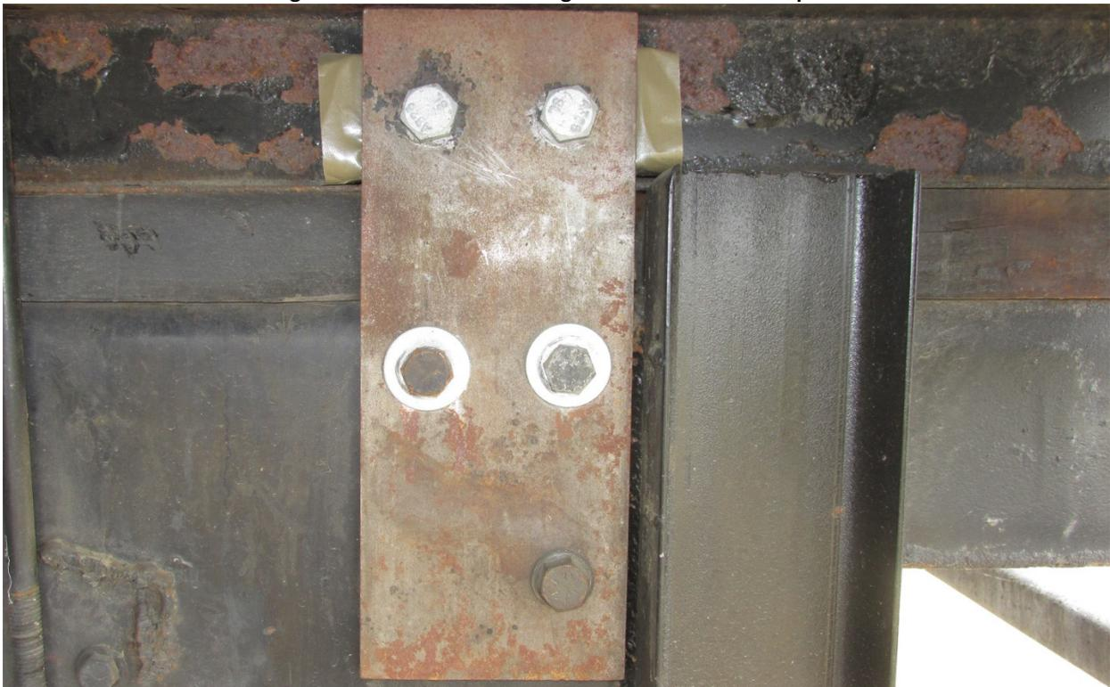
**Figure 7-23 Test 4-12 Rear Left Shear Plate After Impact**
