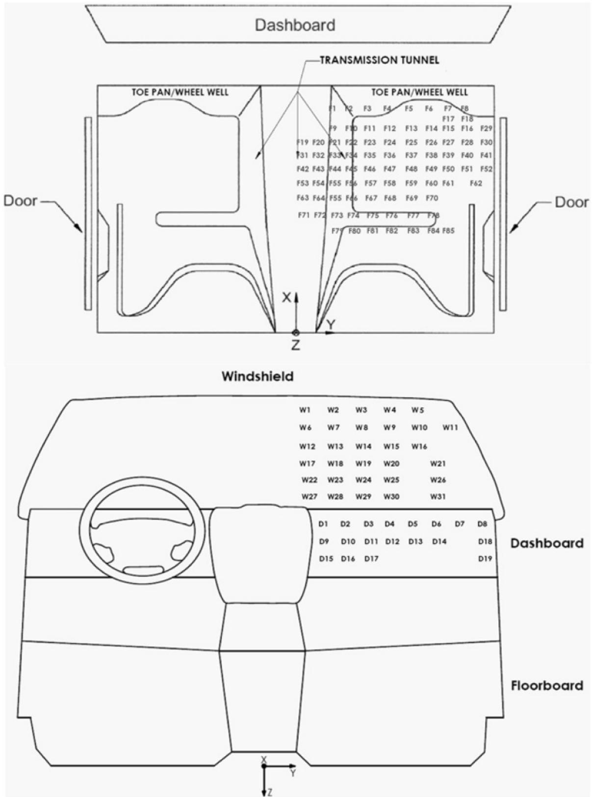
Figure 10-21 Schematic of Measured Interior Points for Floorboard, Dashboard, Windshield, Toe Pan, Wheel Well and Transmission Tunnel
