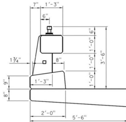
Figure 1-5 Type 85 Concrete Post and Beam Barrier Rail (MASH TL-4)
