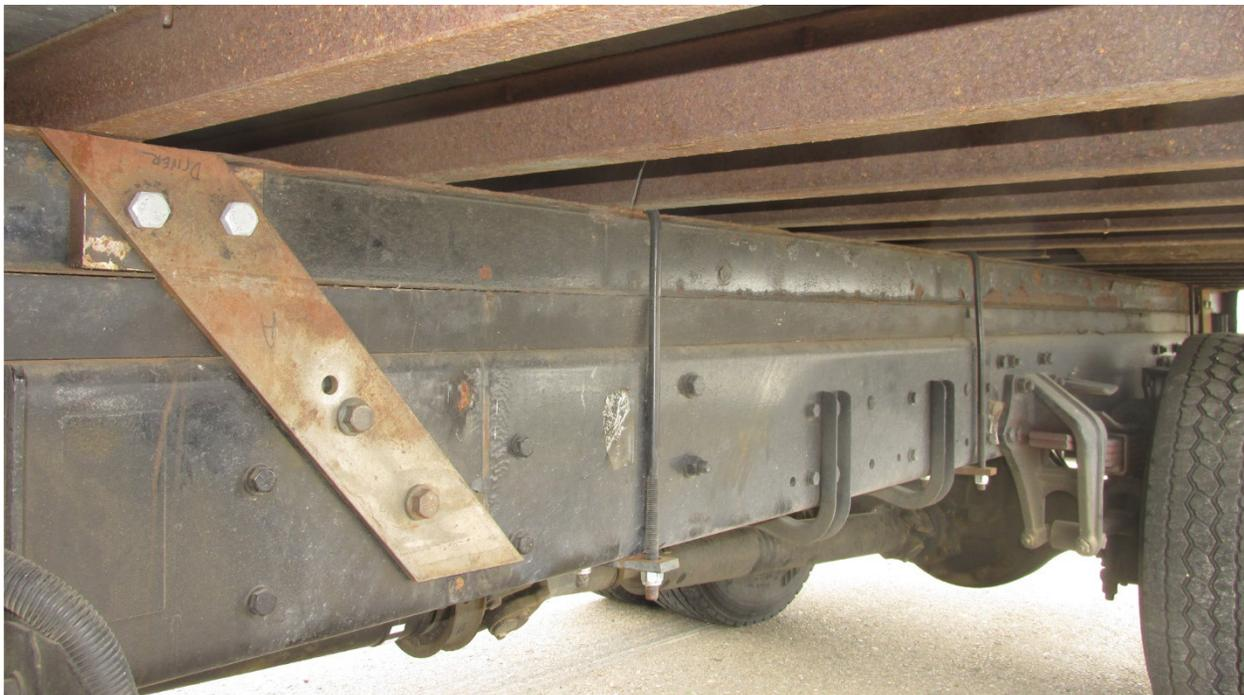
Figure 7-21 Test 4-12 Front Left Shear Plate After Impact
