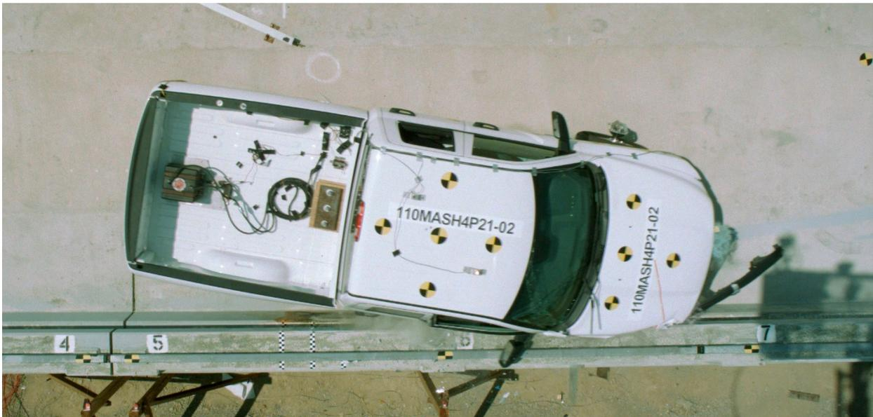
Figure 6-4 Test 4-11 Overhead Camera Impact View
