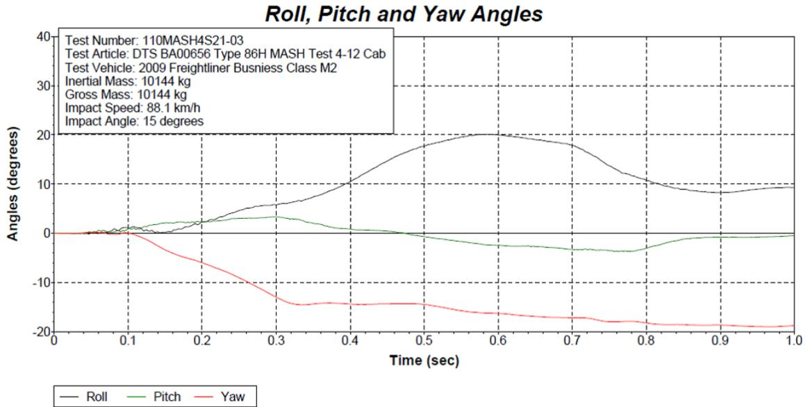
Figure 10-56 Test 4-12 Roll, Pitch, and Yaw Angles (DTS SLICE Micro TRAP BA00656)
