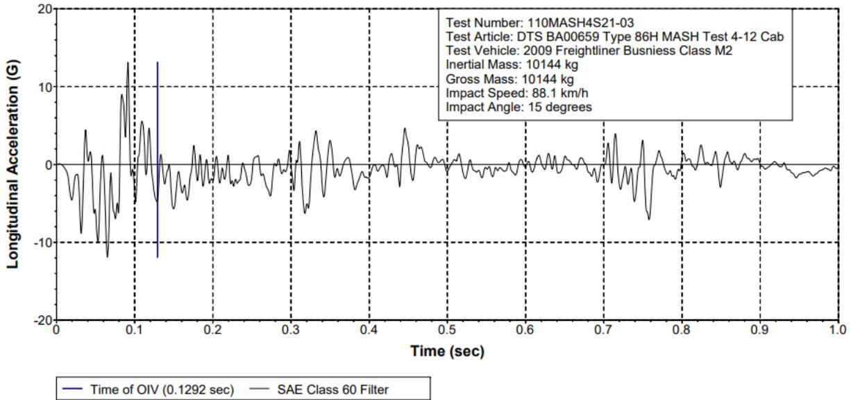
Figure 10-59 Test 4-12 Longitudinal Acceleration (DTS SLICE Micro TRAP BA00659)
