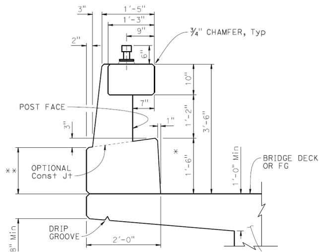
Figure 2-1 Type 86H Cross-Section
