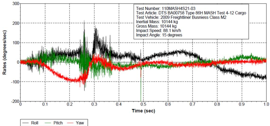
Figure 10-69 Test 4-12 Roll, Pitch, and Yaw Rates (DTS SLICE Micro TRAP BA00758)
