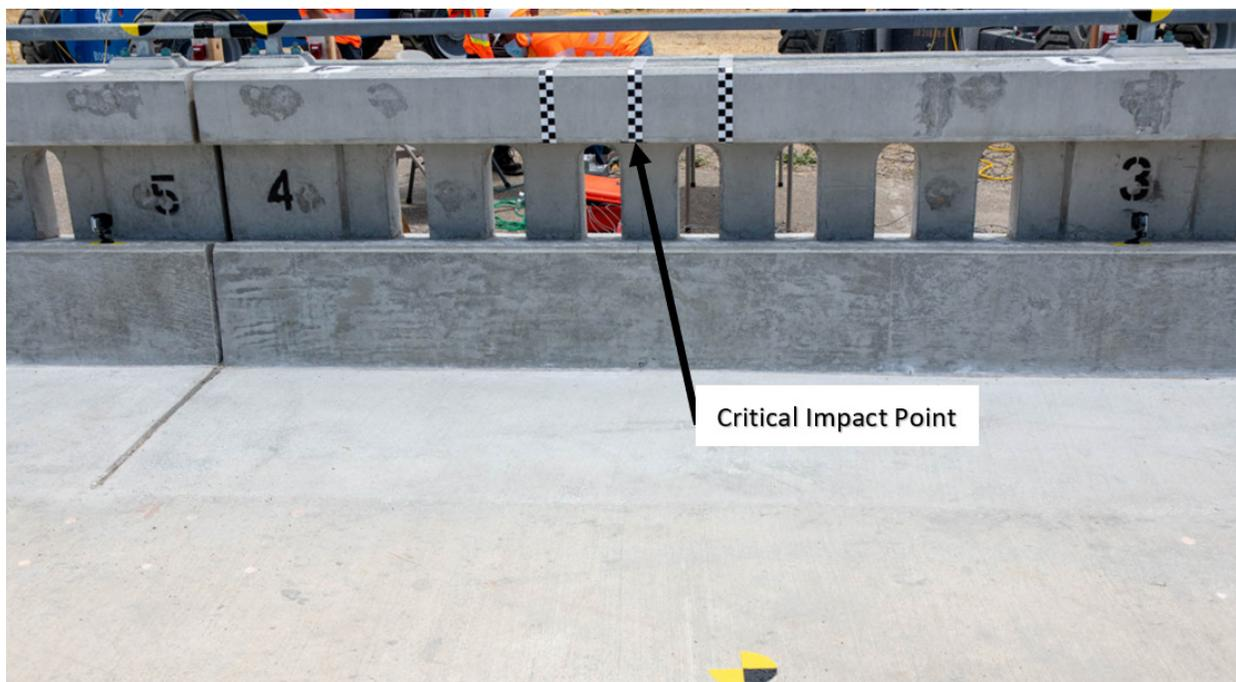
Figure 5-1 Test Article Impact Area Pre-Test 4-10
