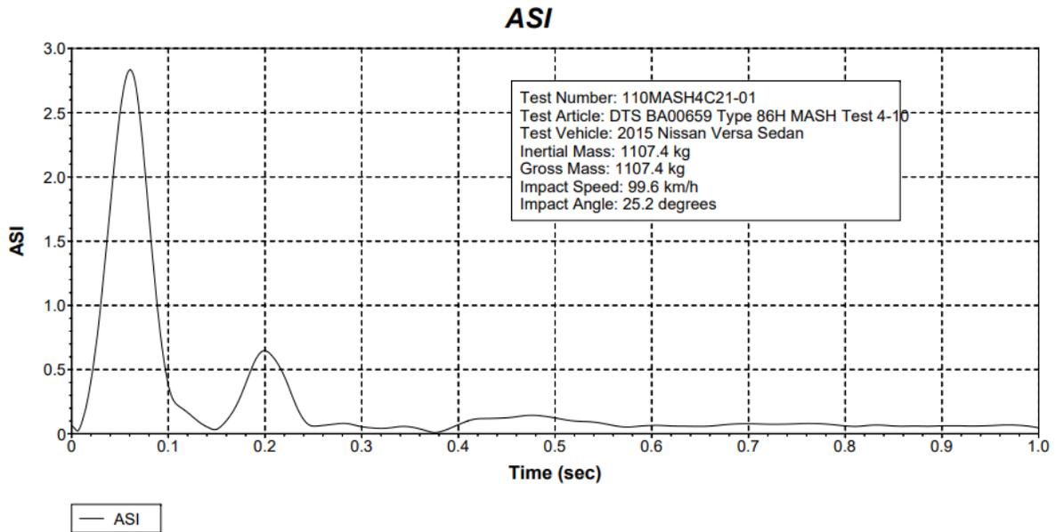
Figure 10-29 Test 4-10 Acceleration Severity Index (DTS SLICE Micro TRAP BA00659)
