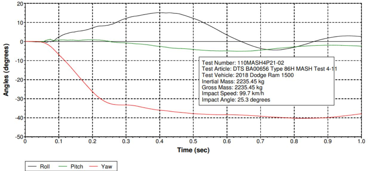
Figure 10-49 Test 4-11 Roll, Pitch, and Yaw Angles (DTS SLICE Micro TRAP BA00656)
