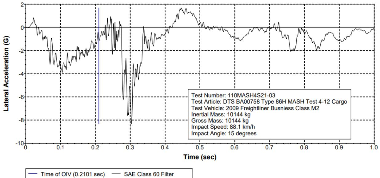
Figure 10-67 Test 4-12 Lateral Acceleration (DTS SLICE Micro TRAP BA00758)
