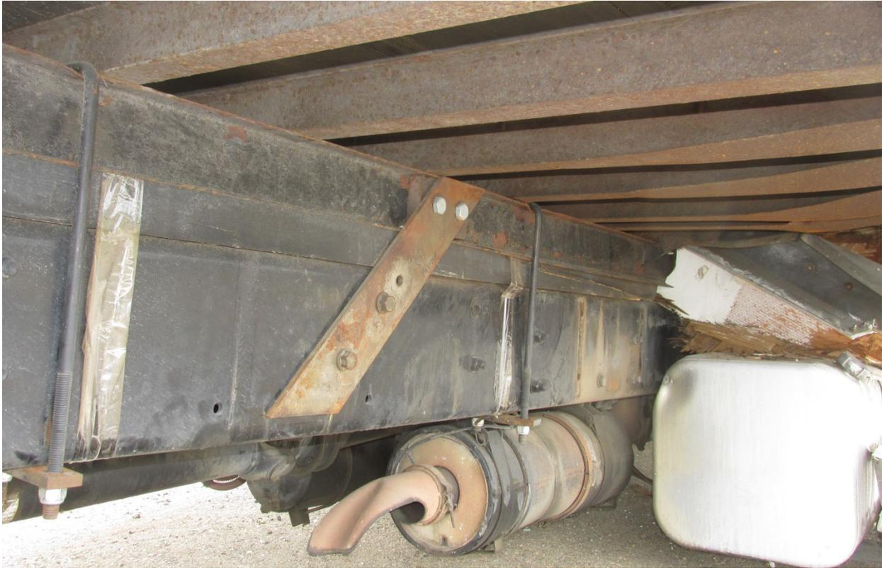
**Figure 7-22 Test 4-12 Front Right Shear Plate After Impact**
