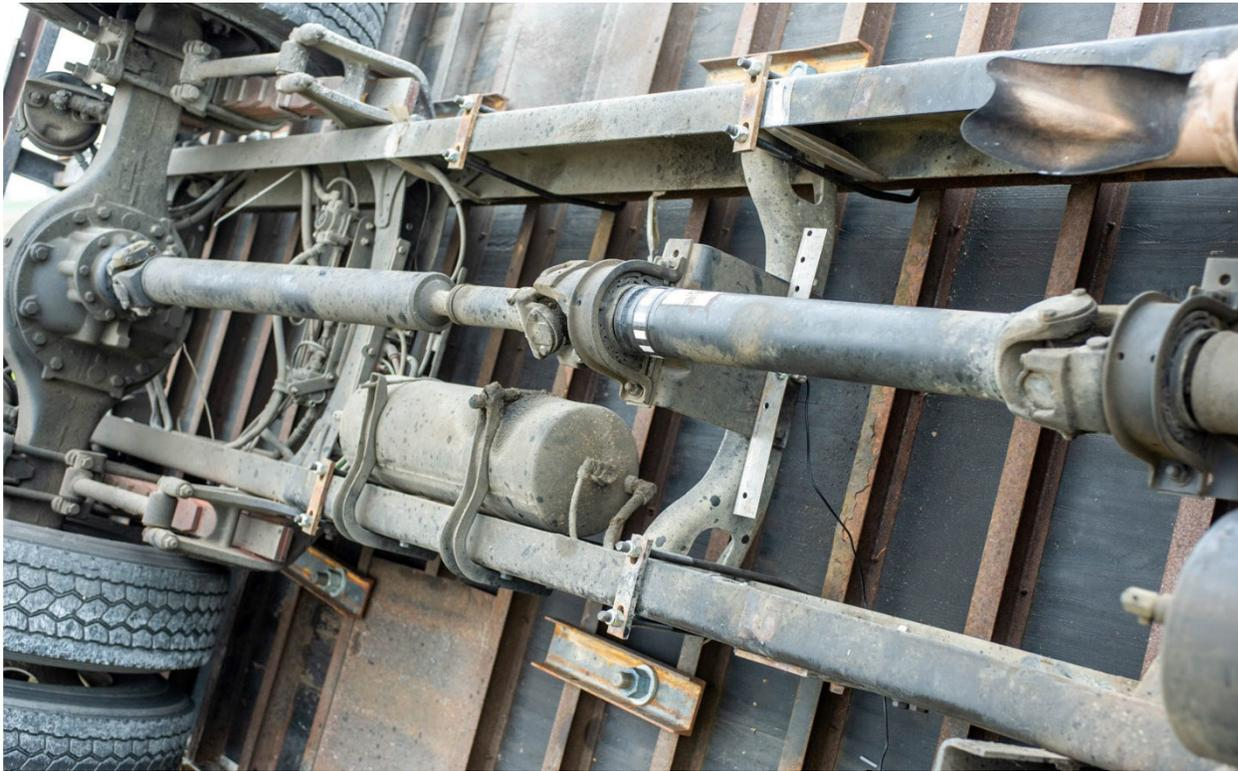
Figure 7-16 MASH 4-12 Test Vehicle Undamaged Undercarriage After Impact (rear)
