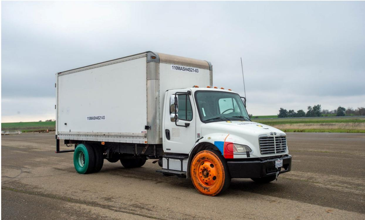
**Figure 4-14 MASH 4-12 Test Vehicle Front Right**
