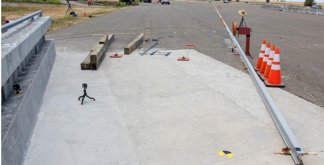
Figure 10-8 Typical Guidance System Layout
