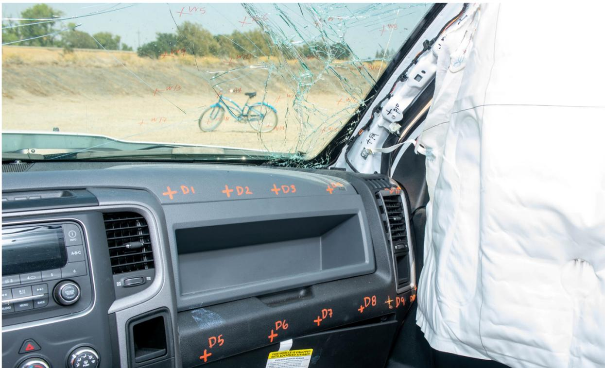
Figure 6-19 Test 4-11 Test Vehicle Damage Windshield / Interior View
