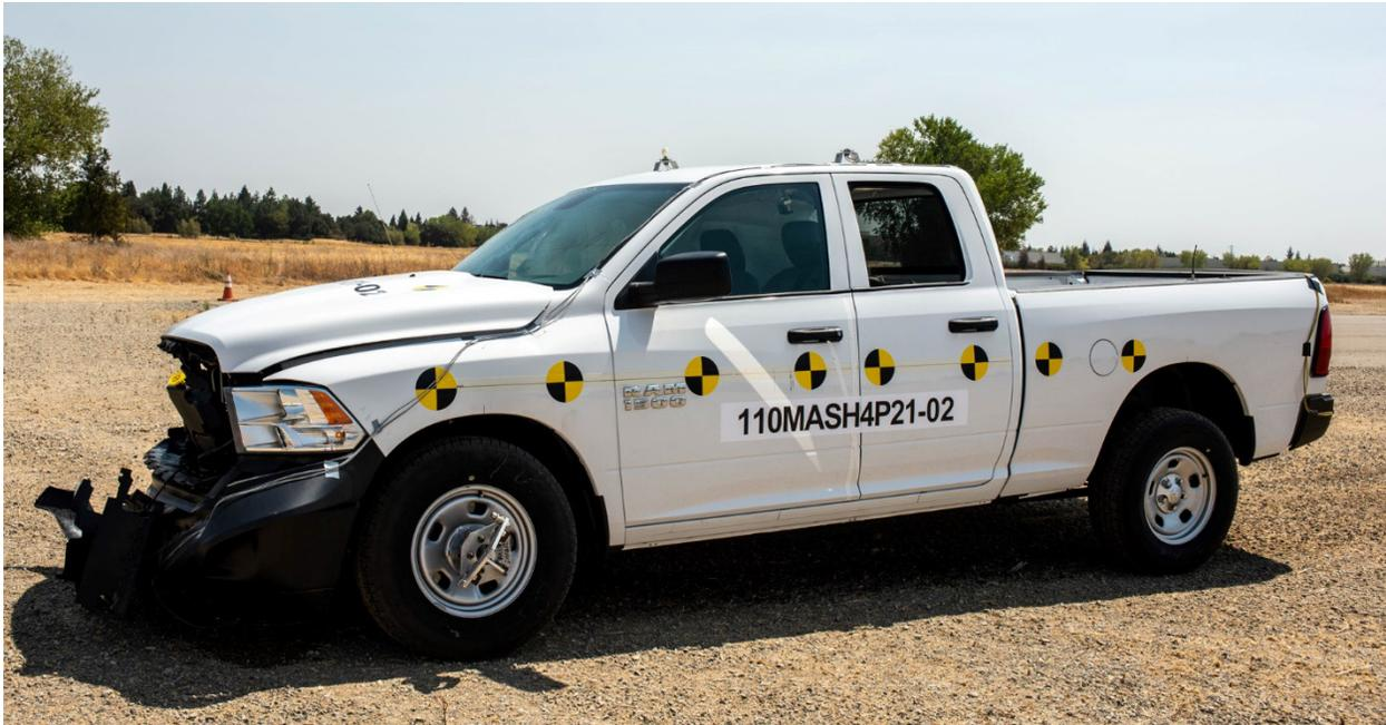
**Figure 6-16 Test 4-11 Test Vehicle Damage (left front)**
