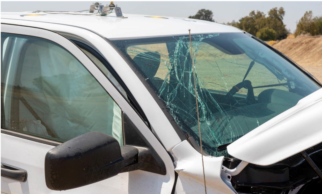
**Figure 6-17 Test 4-11 Test Vehicle Damage Windshield/Exterior**
