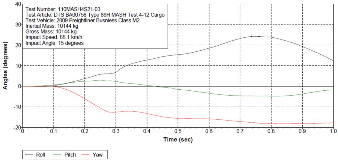
Figure 10-70 Test 4-12 Roll, Pitch, and Yaw Angles (DTS SLICE Micro TRAP BA00758)
