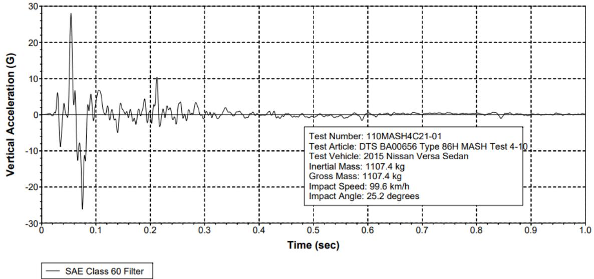
Figure 10-33 Test 4-10 Vertical Acceleration (DTS SLICE Micro TRAP BA00656)
