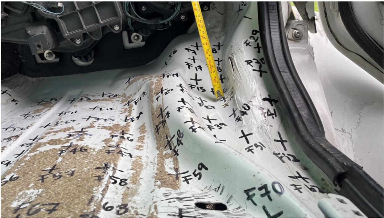
Figure 7-26 Test 4-12 Test Vehicle Passenger-Side Floorboard Deformation
