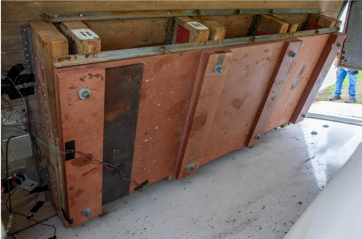
Figure 7-18 Test 4-12 Test Vehicle Ballast After Impact
