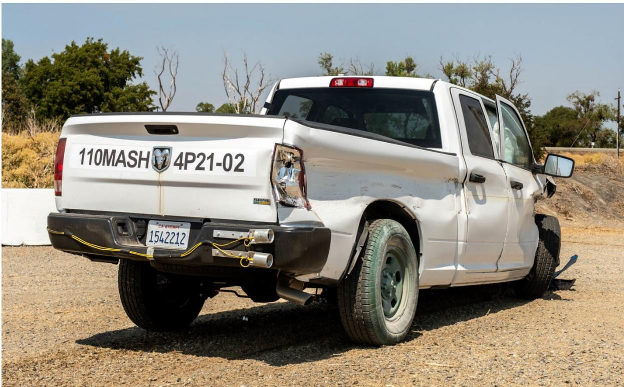
Figure 6-15 Test 4-11 Test Vehicle Damage (right rear)
