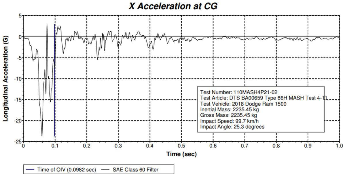
Figure 10-38 Test 4-11 Longitudinal Acceleration (DTS SLICE Micro TRAP BA00659)
