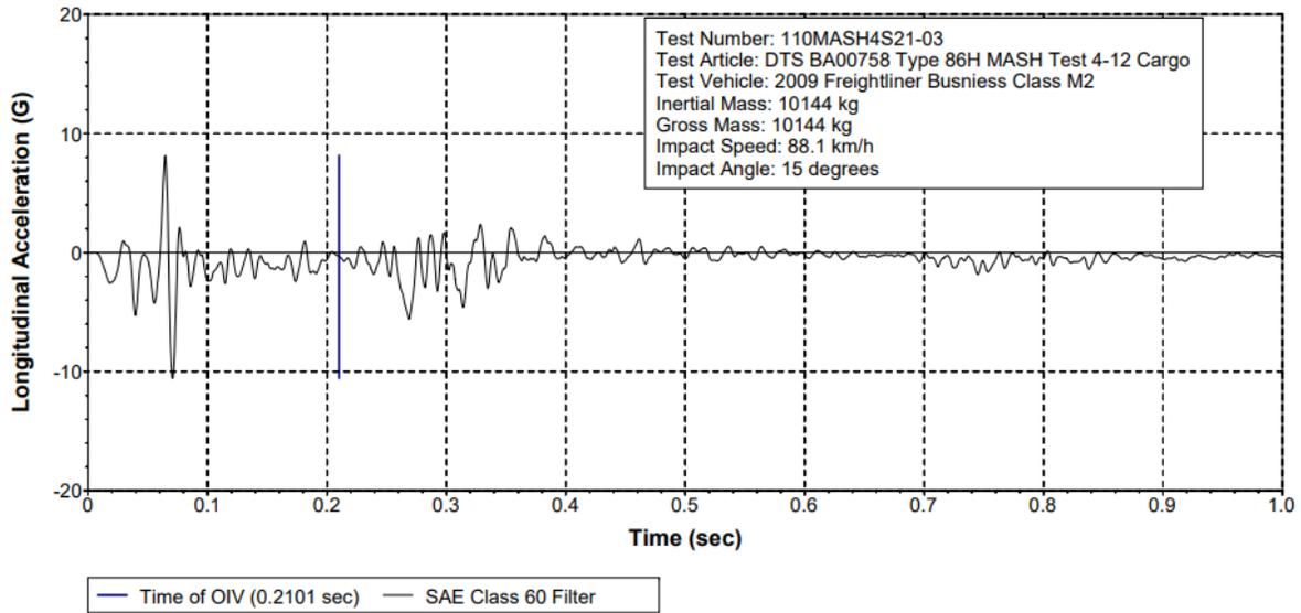
Figure 10-66 Test 4-12 Longitudinal Acceleration (DTS SLICE Micro TRAP BA00758)
