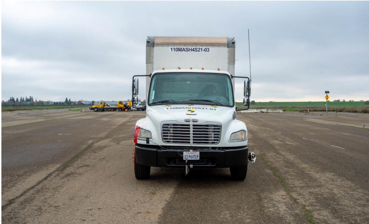
Figure 4-16 MASH 4-12 Test Vehicle Front
