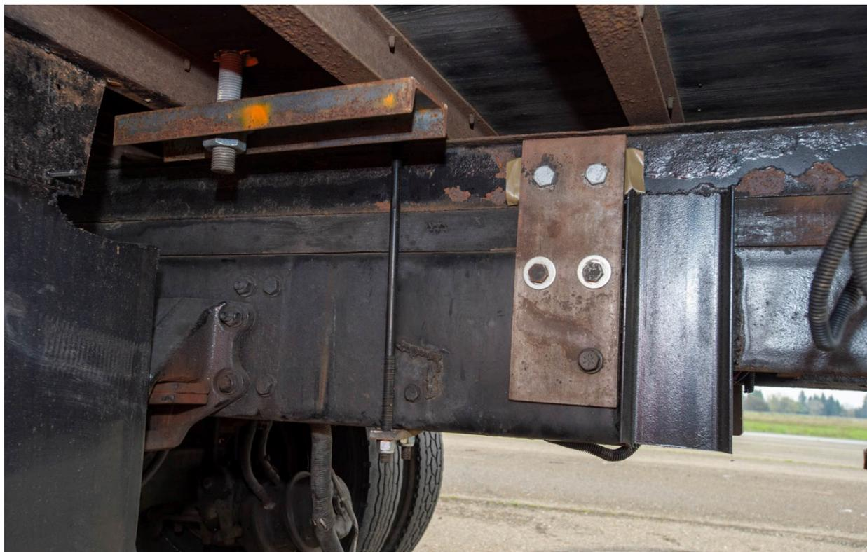
**Figure 4-24 MASH 4-12 Test Vehicle Rear Shear Plate and Ballast Mounting Plate**
