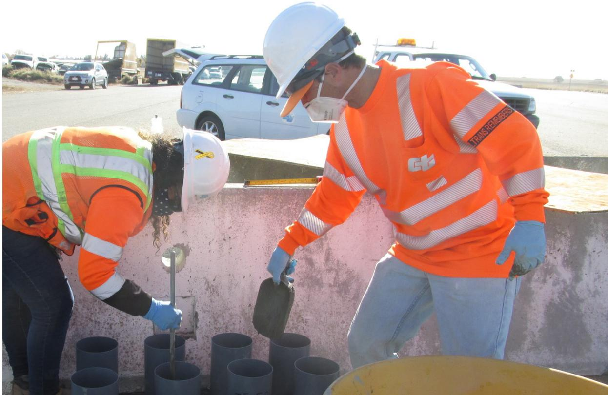
**Figure 2-25 Concrete Samples Taken During the Curb Pour by Caltrans Staff**
