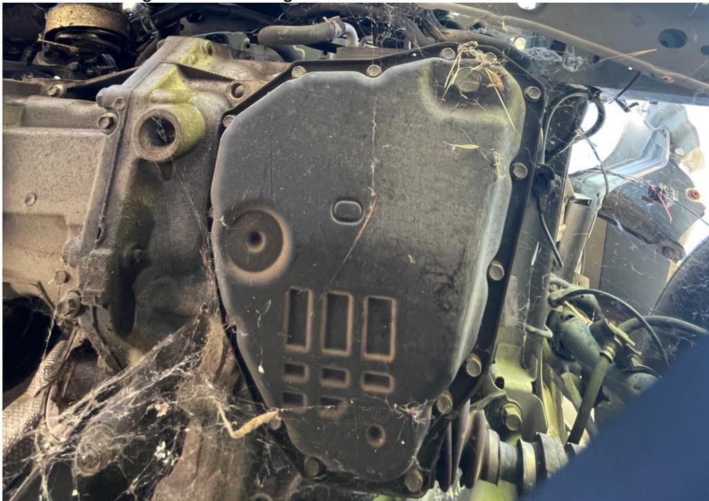
**Figure 13-2 Undamaged Oil Pan for the 1100C vehicle**
