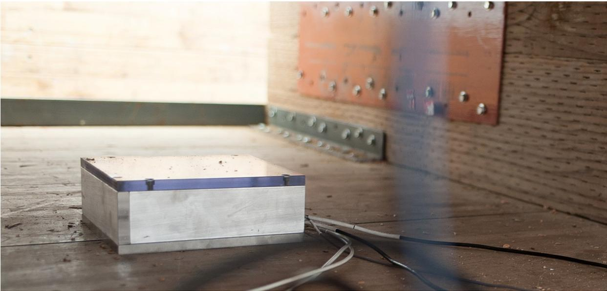
**Figure 10-6 Test 4-12 DTS SLICE Micro Mount Position in Cargo Box**
