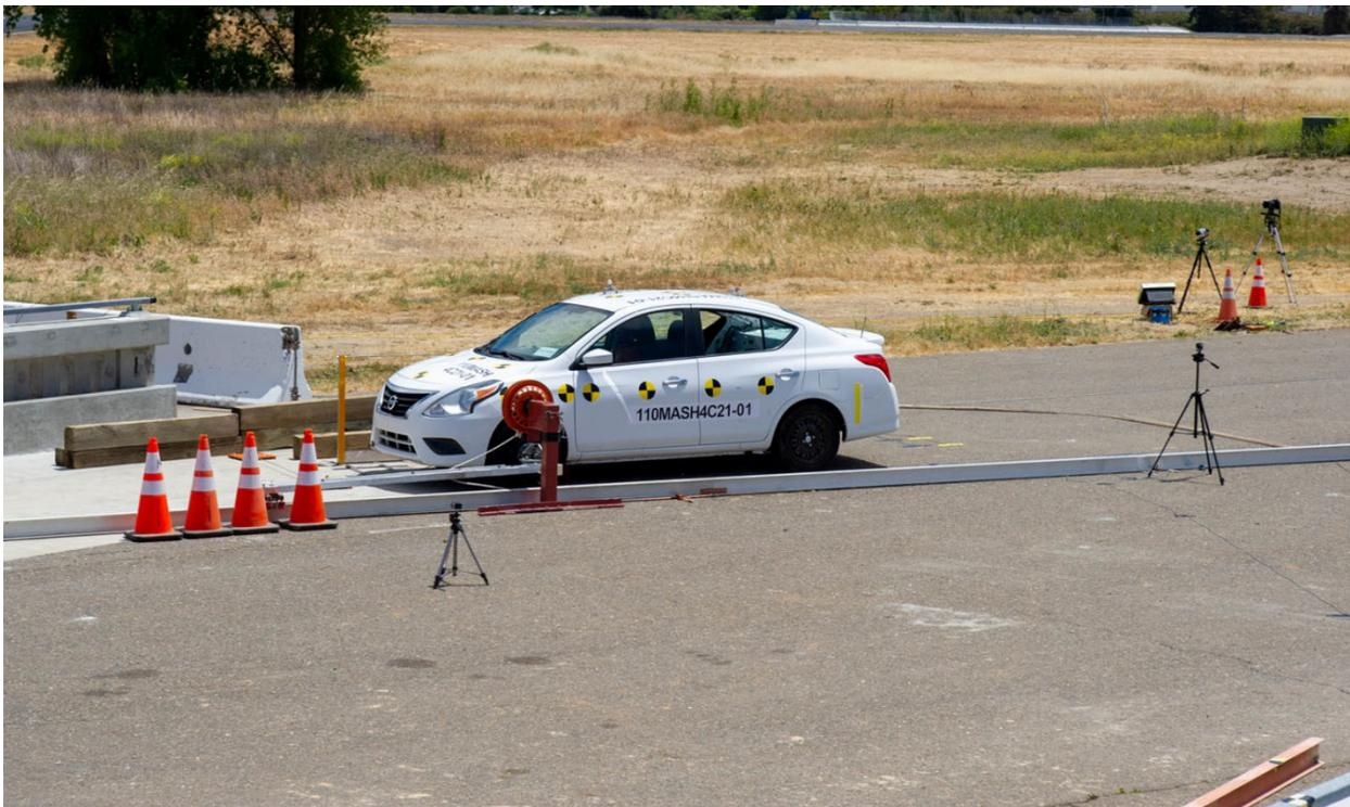
Figure 10-9 Guide Arm Releasing from Test Vehicle
