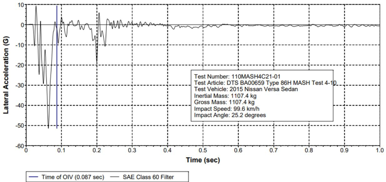
Figure 10-25 Test 4-10 Lateral Acceleration (DTS SLICE Micro TRAP BA00659)
