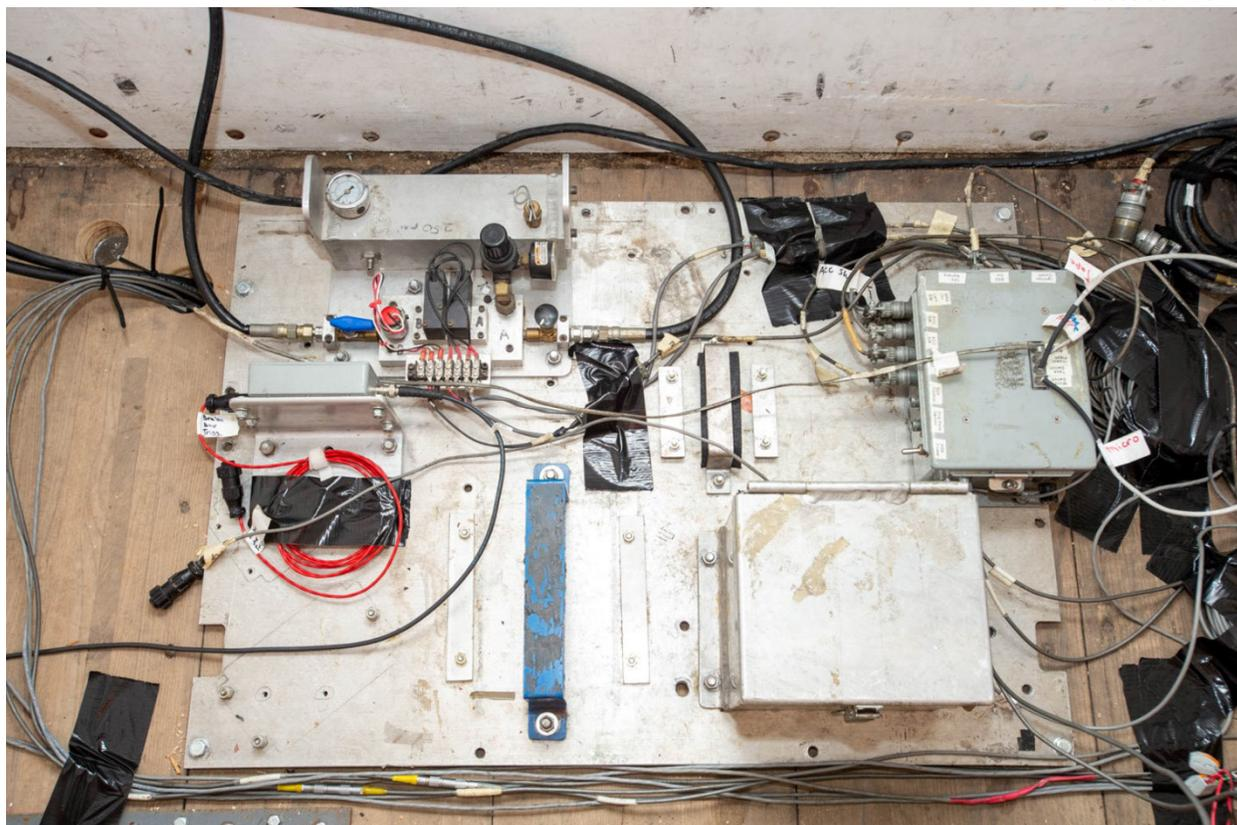
**Figure 10-7 Test 4-12 Vehicle Instrumentation Mounted in Cargo Box**
