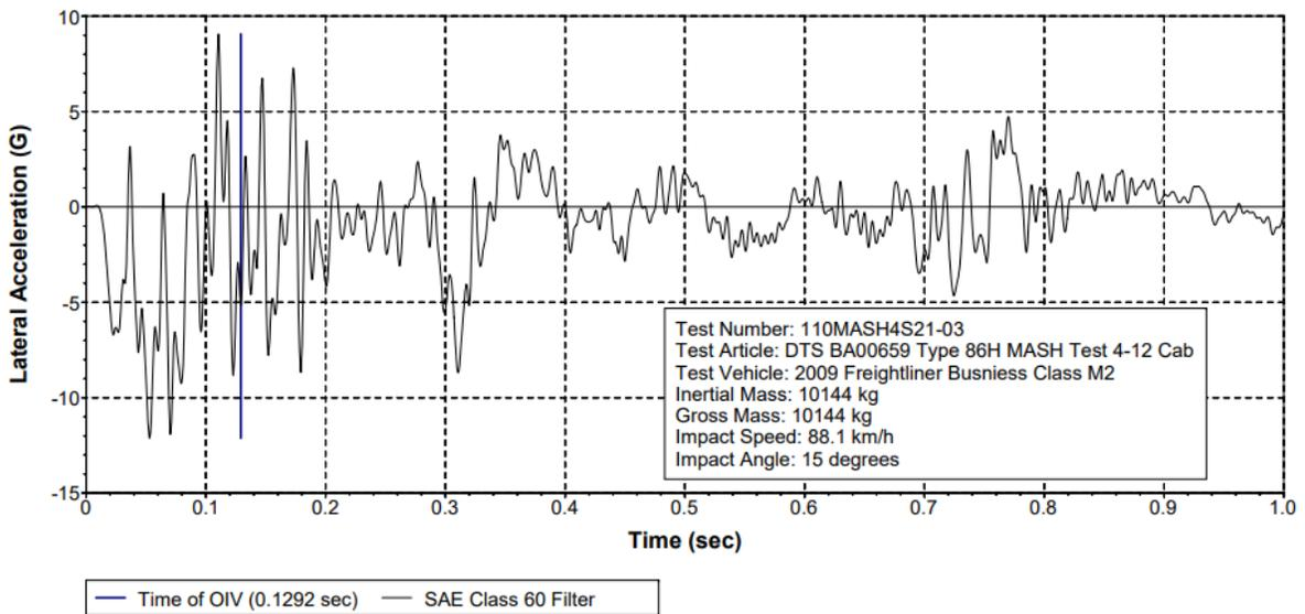
Figure 10-60 Test 4-12 Lateral Acceleration (DTS SLICE Micro TRAP BA00659)
