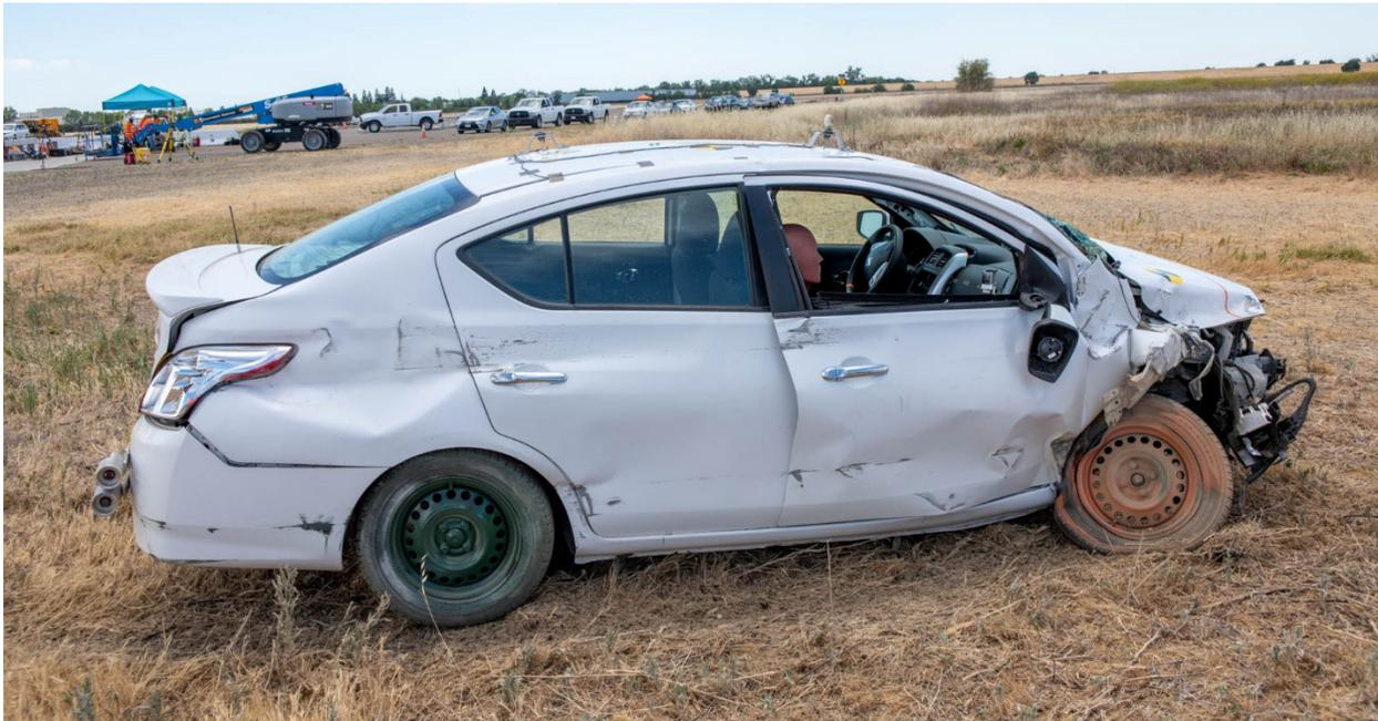
Figure 5-12 Test 4-10 Test Vehicle Damage (right)
