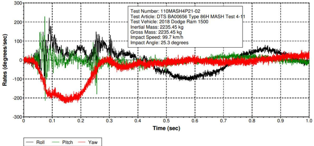
Figure 10-48 Test 4-11 Roll, Pitch, and Yaw Rates (DTS SLICE Micro TRAP BA00656)
