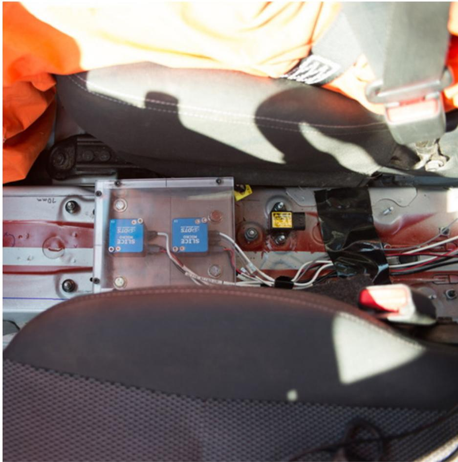
**Figure 10-2 DTS SLICE Micro Mount Position in the Vehicle Test 4-10**
