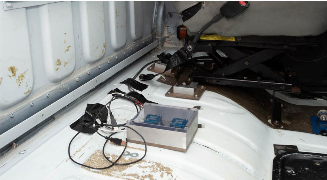
**Figure 10-5 Test 4-12 DTS SLICE Micro Mount Position in the Cab**
