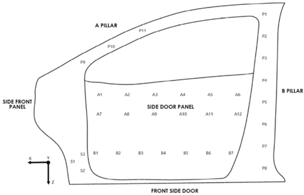
**Front Door Area Internal Measurements**
