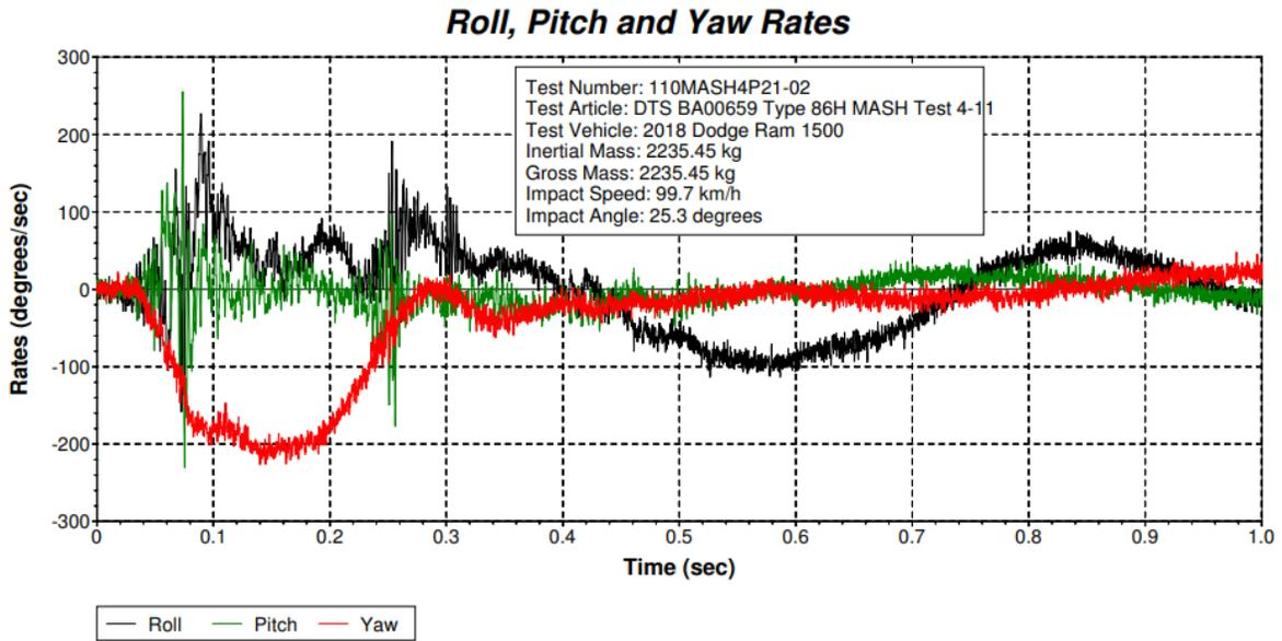
Figure 10-41 Test 4-11 Roll, Pitch, and Yaw Rates (DTS SLICE Micro TRAP BA00659)
