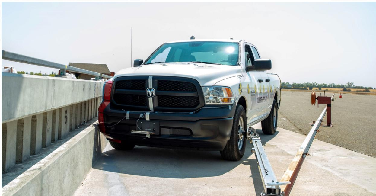
Figure 4-13 MASH 4-11 Test Vehicle at Impact Point
