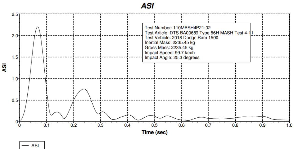
Figure 10-43 Test 4-11 Acceleration Severity Index (DTS SLICE Micro TRAP BA00659)
