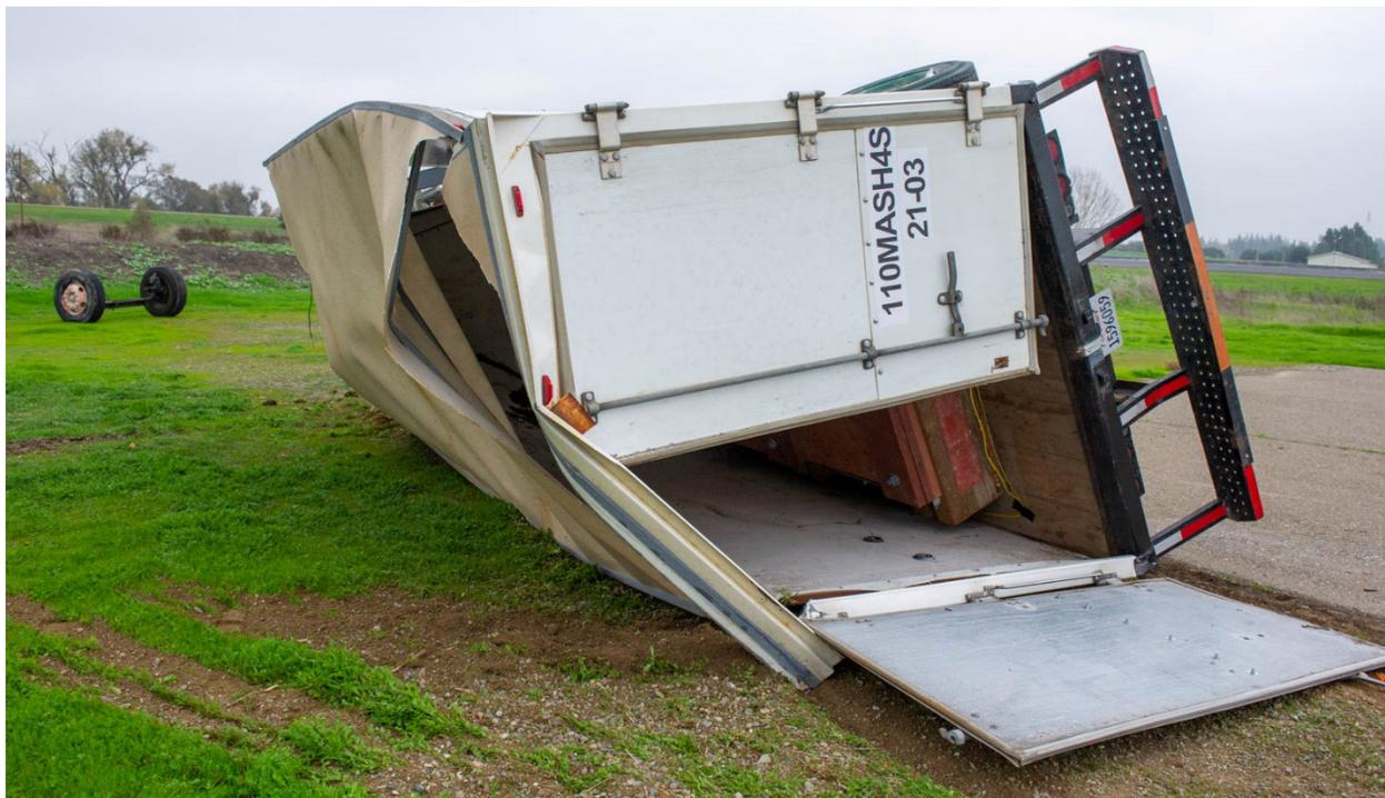
Figure 7-17 Test 4-12 Test Vehicle After Impact (Rear)
