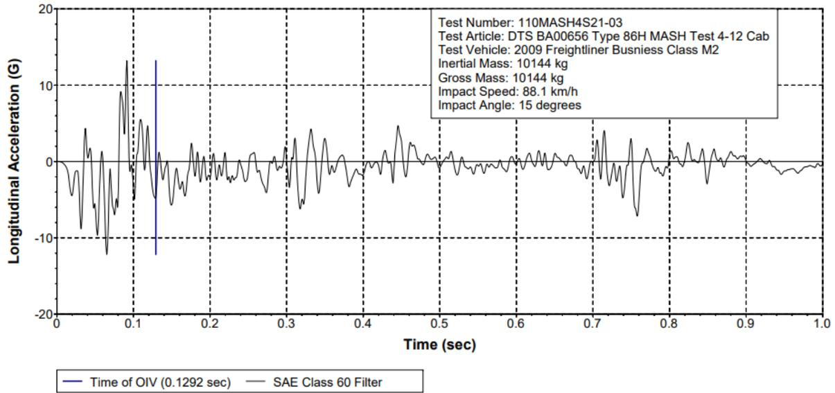
Figure 10-52 4-12 Longitudinal Acceleration (DTS SLICE Micro TRAP BA00656)
