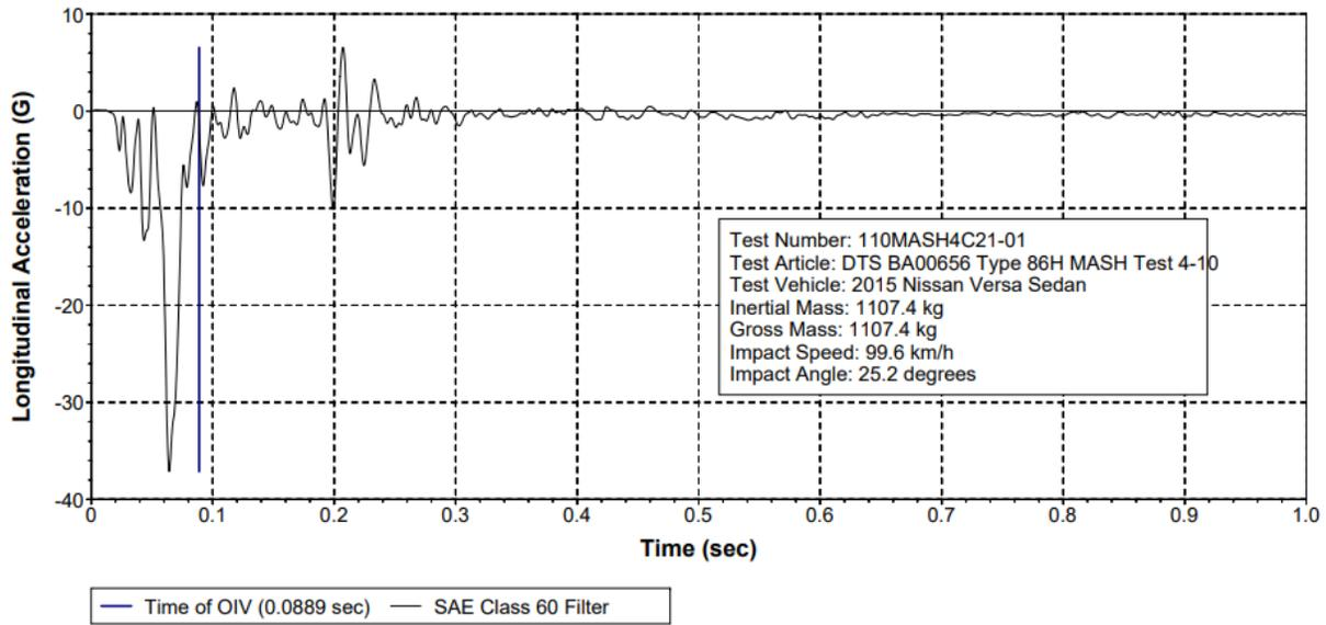
Figure 10-31 Test 4-10 Longitudinal Acceleration (DTS SLICE Micro TRAP BA00656)
