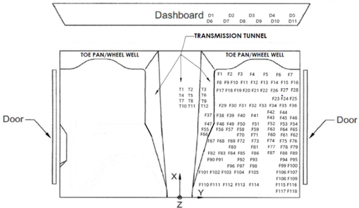
**Floorboard Area Internal Measurements**
