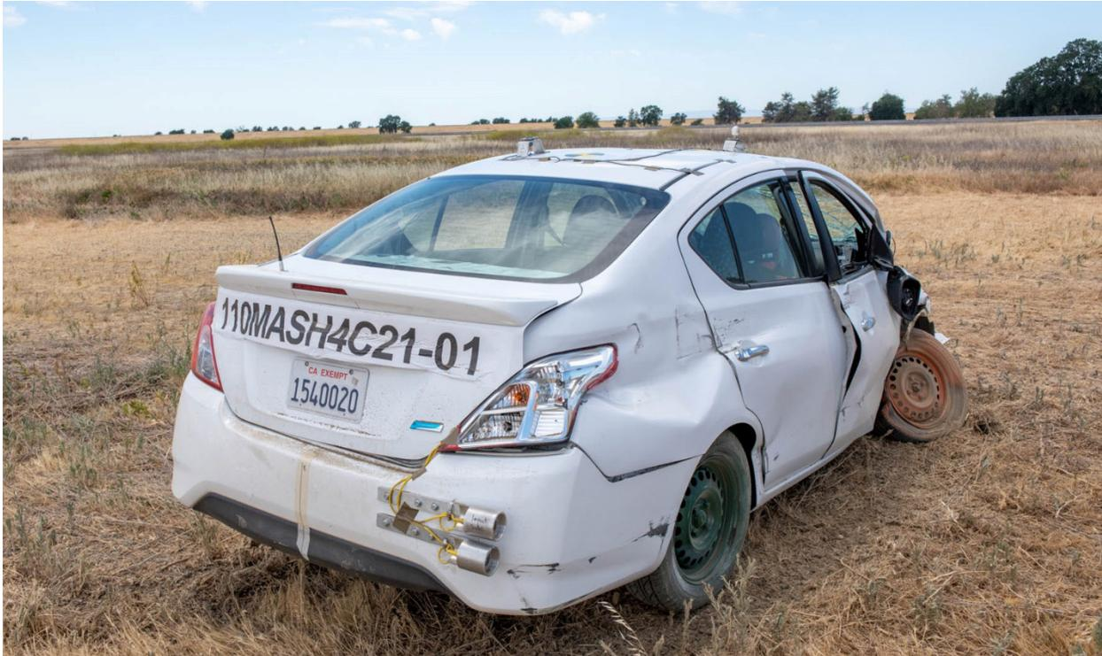
Figure 5-16 Test 4-10 Test Vehicle Damage (right rear)
