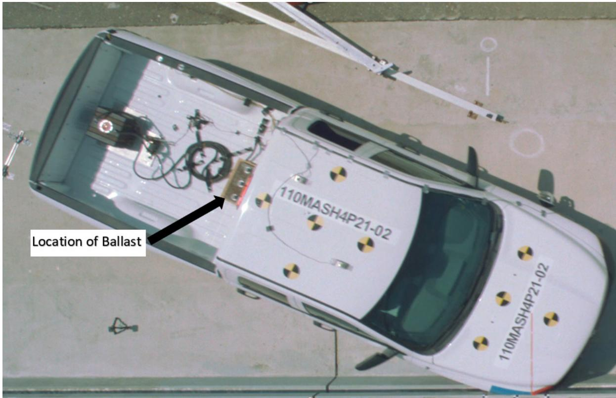
Figure 4-12 MASH 4-11 Test Vehicle Ballast
