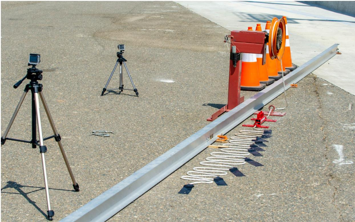
**Figure 10-13 Guide Arm Brake System with Friction Brake (Prior To Pickup Test)**
