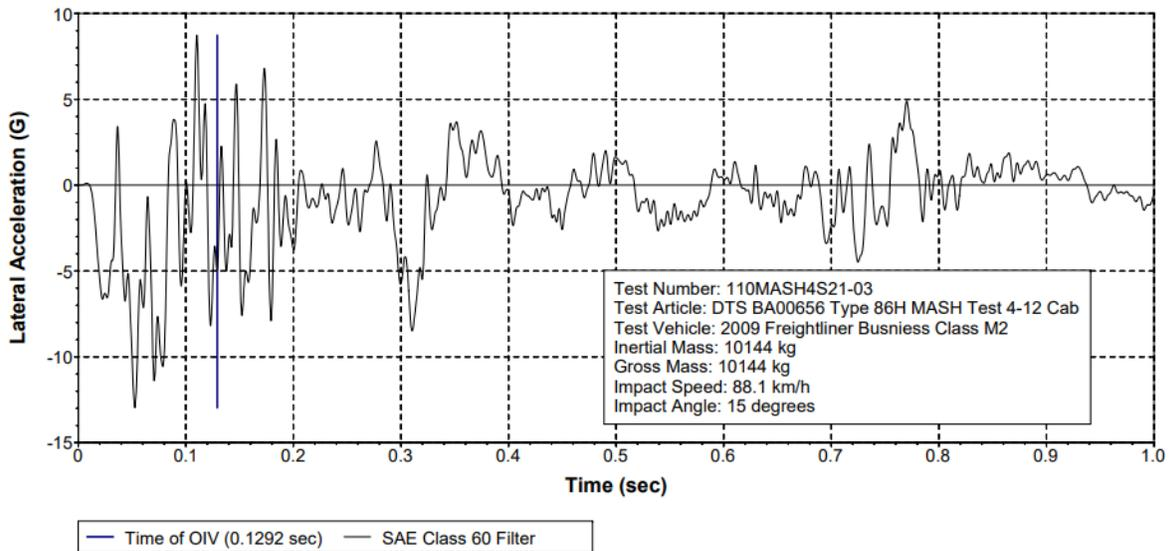
Figure 10-53 Test 4-12 Lateral Acceleration (DTS SLICE Micro TRAP BA00656)
