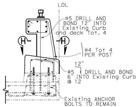
Figure 2-5 Partial Cross Section of Drilled and Bonded Type 86H (MOD) on Existing Reaction Slab
