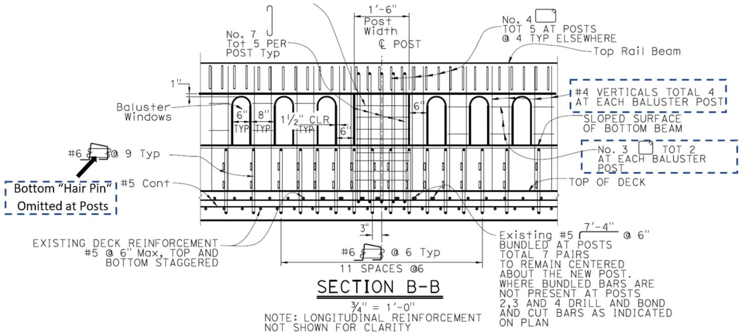
Figure 2-27 Section B-B with Concrete Reinforcement
