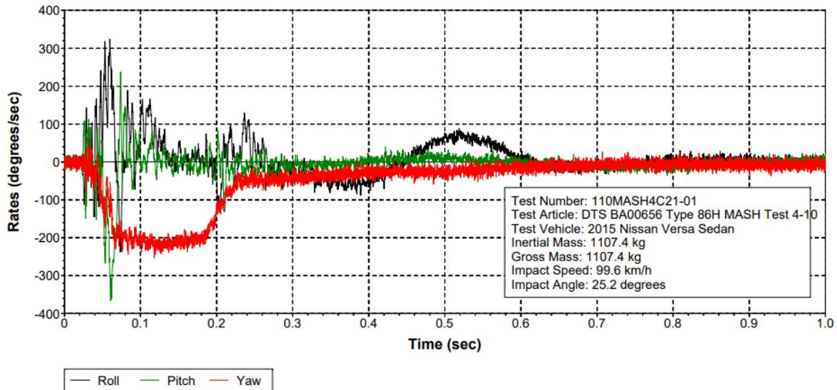
Figure 10-34 Test 4-10 Roll, Pitch, and Yaw Rates (DTS SLICE Micro TRAP BA00656)
