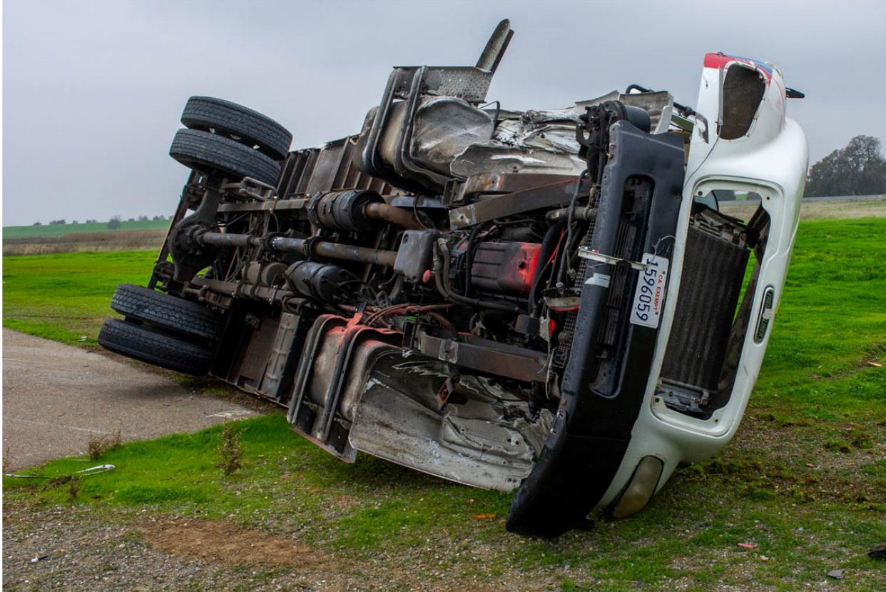
Figure 7-14 Test 4-11 Test Vehicle Damage (front right)
