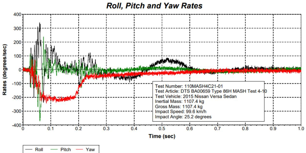
Figure 10-27 Test 4-10 Roll, Pitch, and Yaw Rates (DTS SLICE Micro TRAP BA00659)
