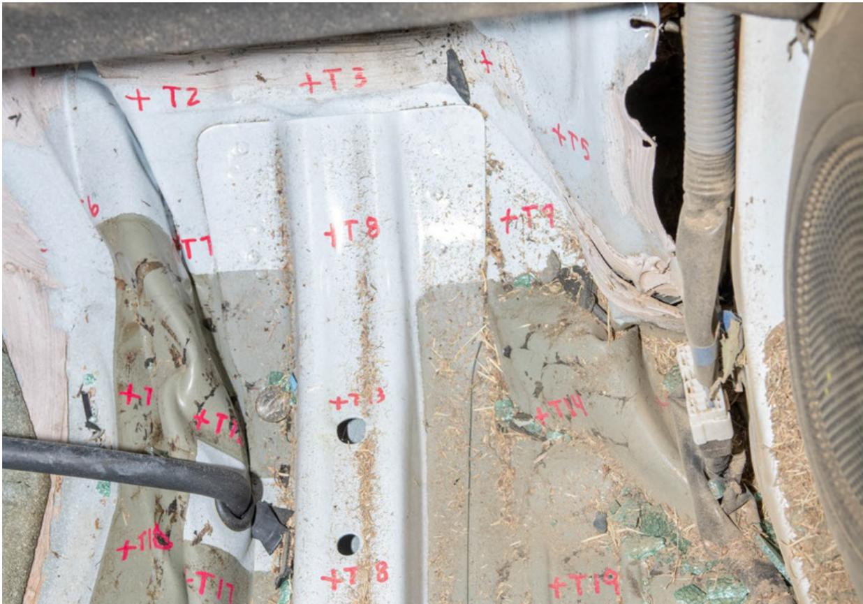
Figure 5-23 Test 4-10 Floorboard Deformation
