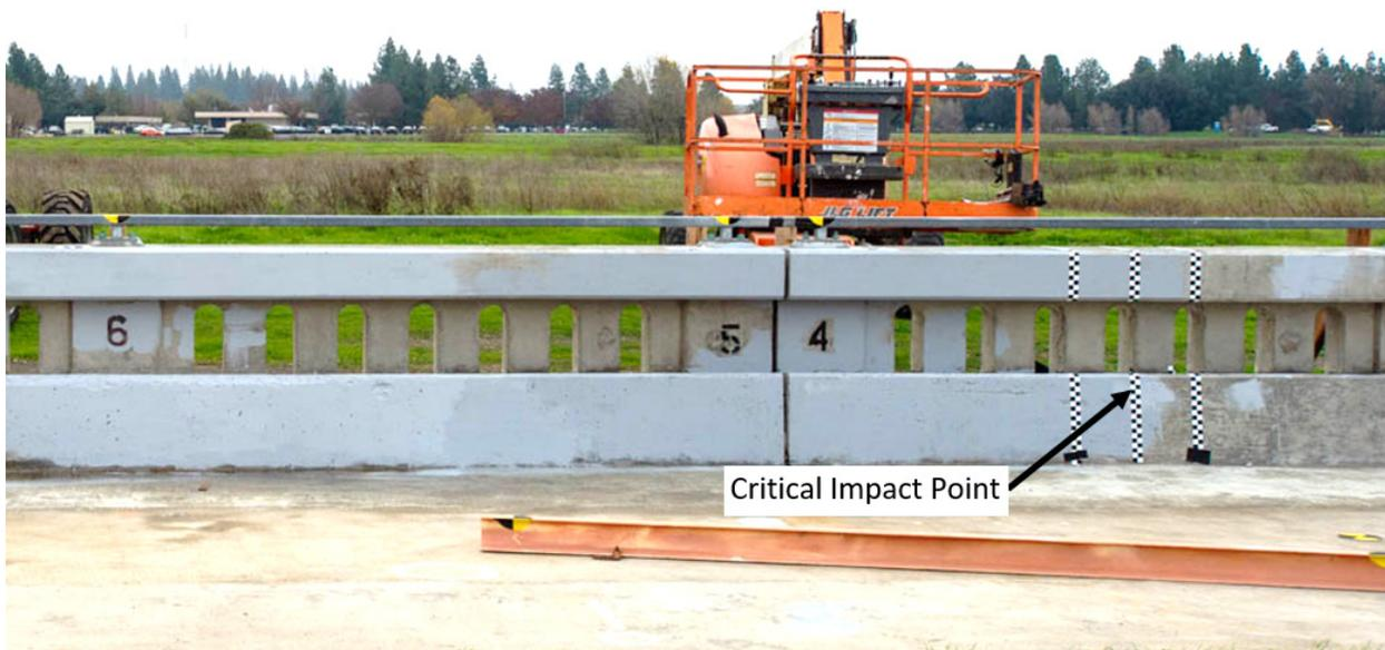
Figure 7-2 Test Article Downstream of Impact Area Pre-Test 4-12
