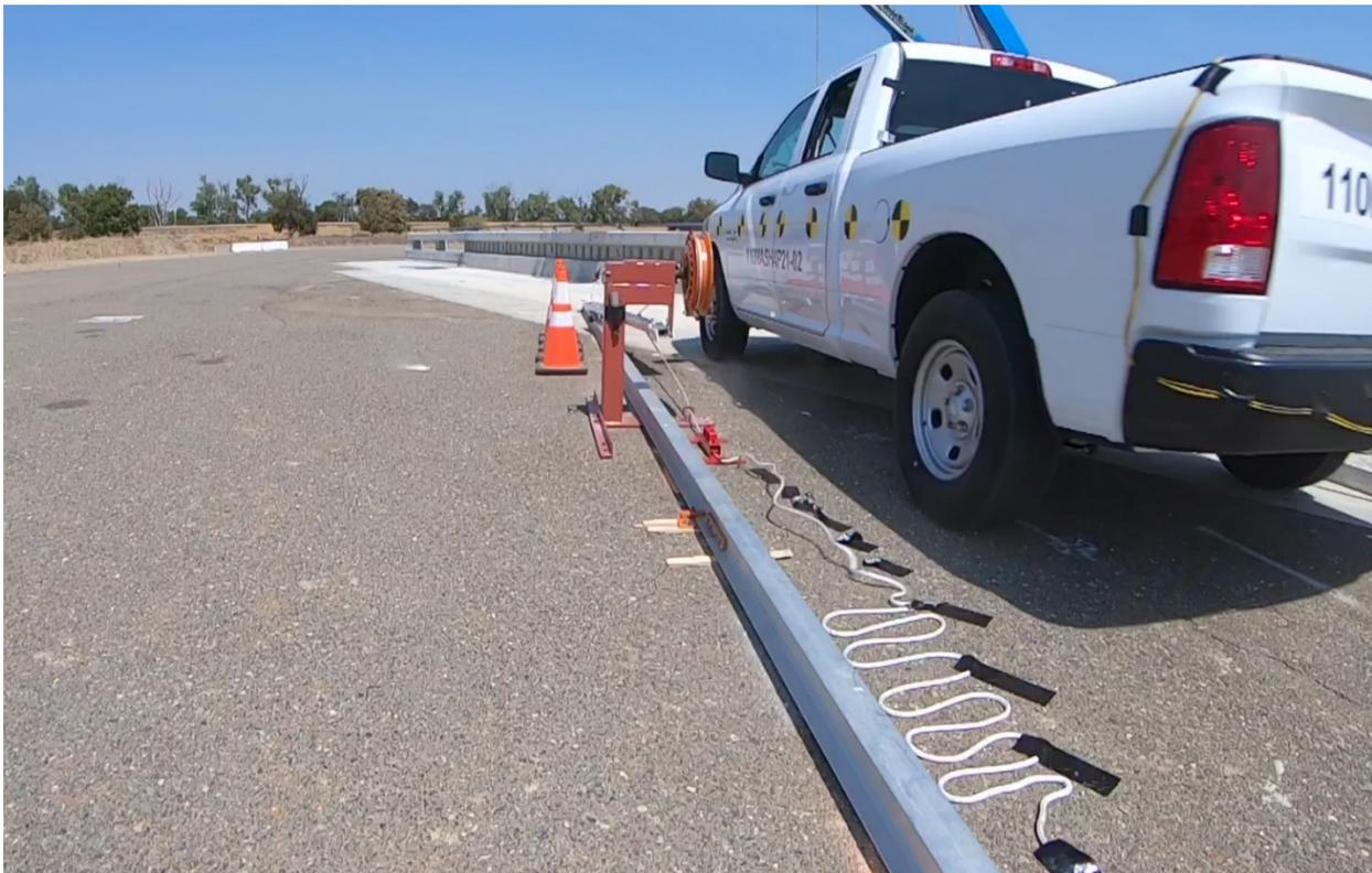
**Figure 10-14 Released Guide Arm with Engaged Friction Brake (Pickup Test Prior to Impact)**
