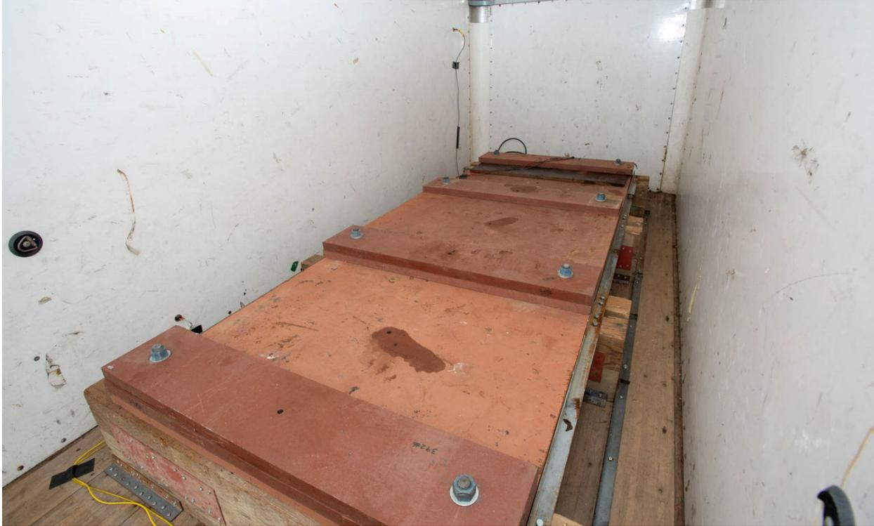
Figure 4-20 MASH 4-12 Test Vehicle Ballast in Cargo Box
