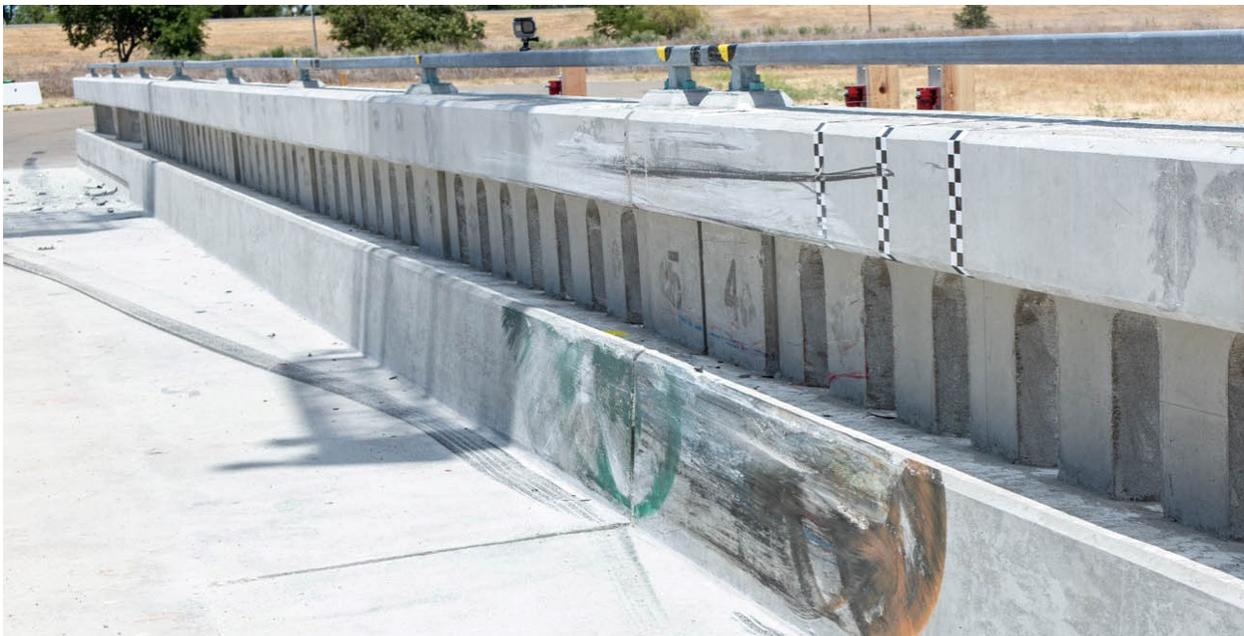
Figure 5-8 Test 4-10 Overview of Barrier Post-Test
