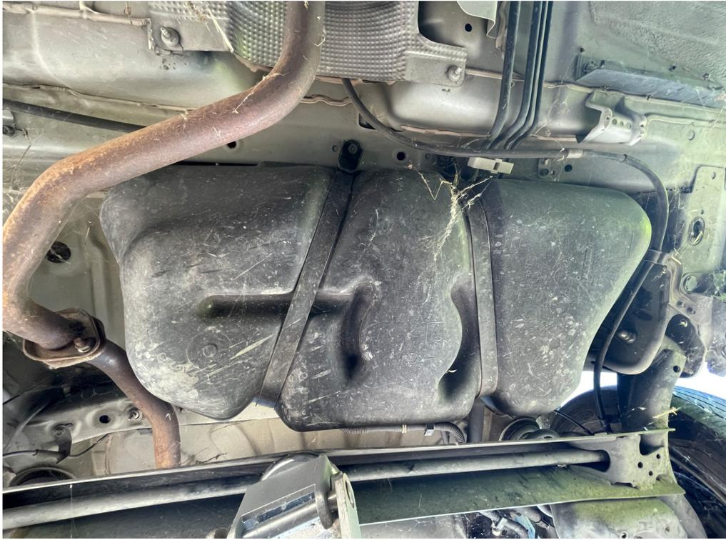
**Figure 13-1 Undamaged Gasoline Tank for the 1100C vehicle**
