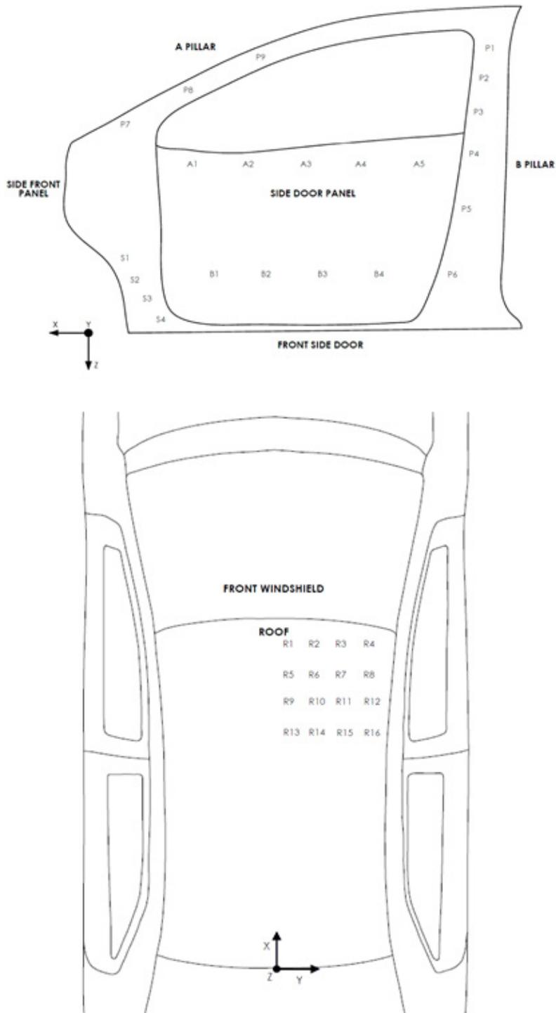
Figure 10-18 Schematic of Measured Points for the A Pillar, B Pillar, Side Front Door Panel, Side Door Panel, Front Side Door and Roof
