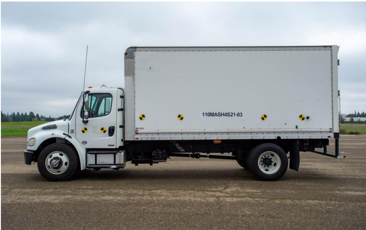
Figure 4-17 MASH 4-12 Test Vehicle Driver Side
