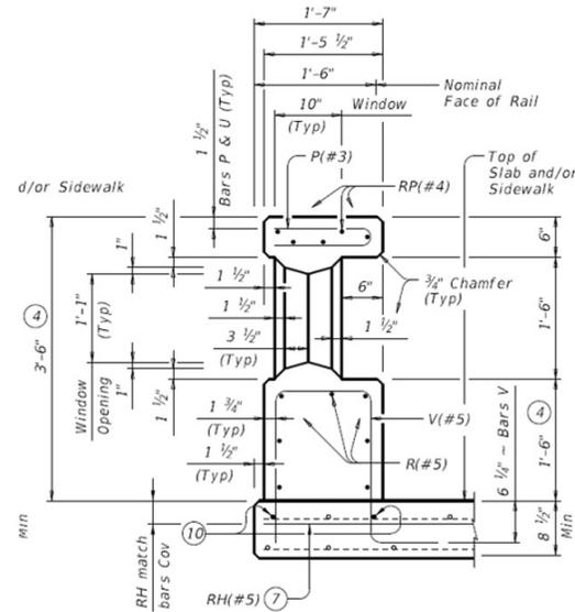
**Figure 1-7 Texas C412 Concrete Baluster Bridge Rail (MASH TL-5)**
