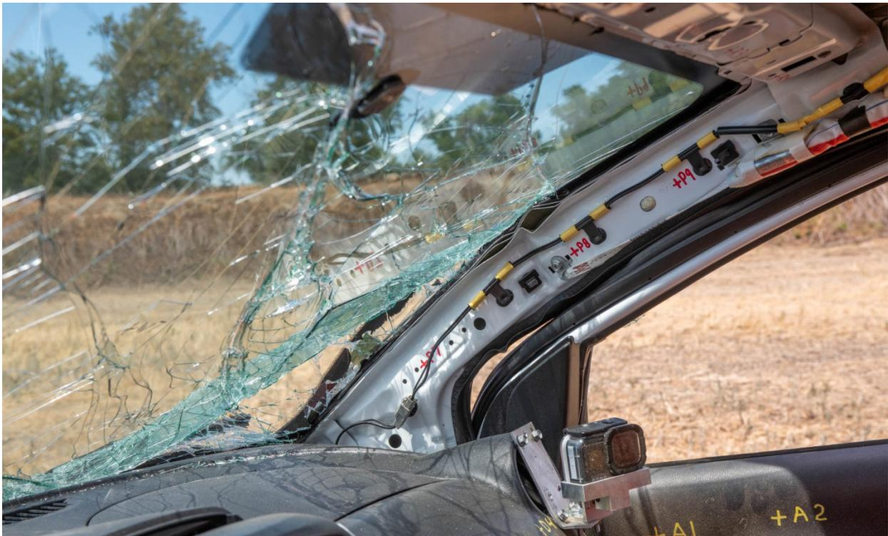
Figure 5-19 Test 4-10 Test Vehicle Damage Windshield / Interior View
