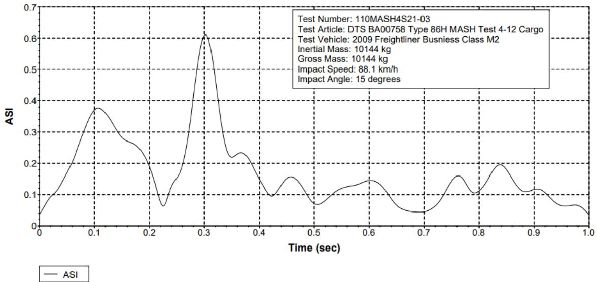
Figure 10-71 Test 4-12 Acceleration Severity Index (DTS SLICE Micro TRAP BA00758)
