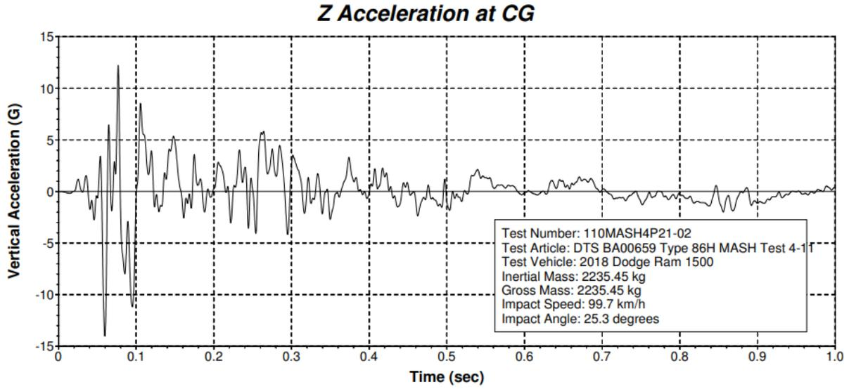
Figure 10-40 Test 4-11 Vertical Acceleration (DTS SLICE Micro TRAP BA00659)
