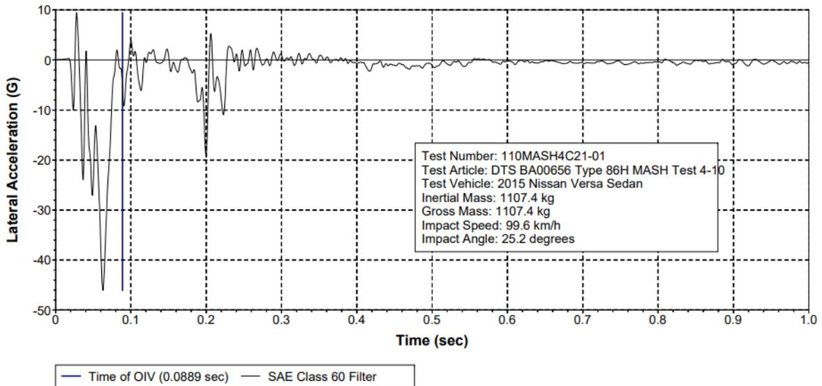
Figure 10-32 Test 4-10 Lateral Acceleration (DTS SLICE Micro TRAP BA00656)
