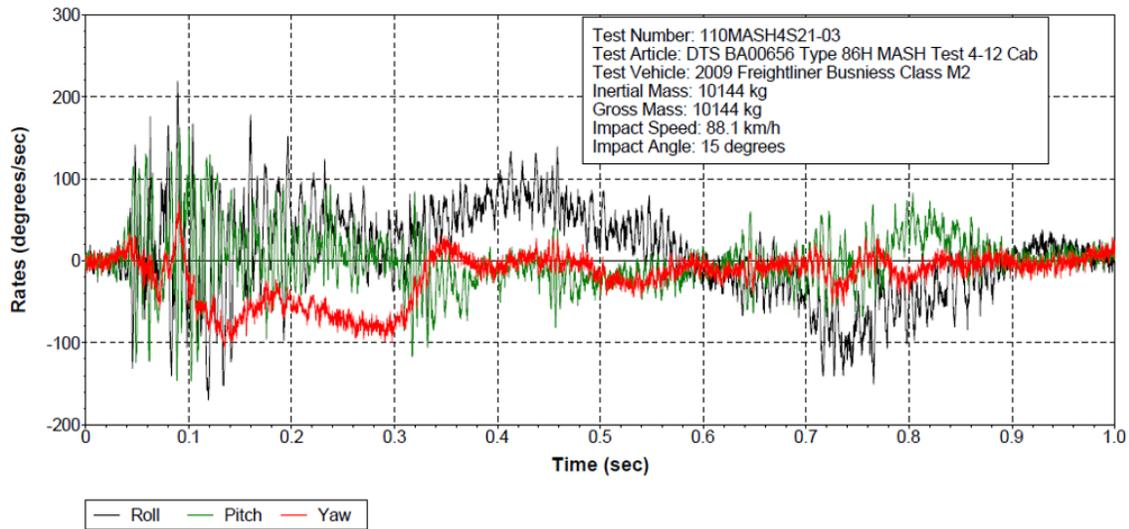
Figure 10-55 Test 4-12 Roll, Pitch, and Yaw Rates (DTS SLICE Micro TRAP BA00656)
