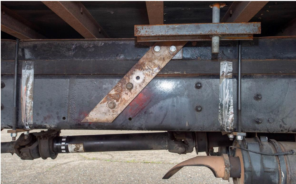
**Figure 4-23 MASH 4-12 Test Vehicle Front Shear Plate and Ballast Mounting Plate**
