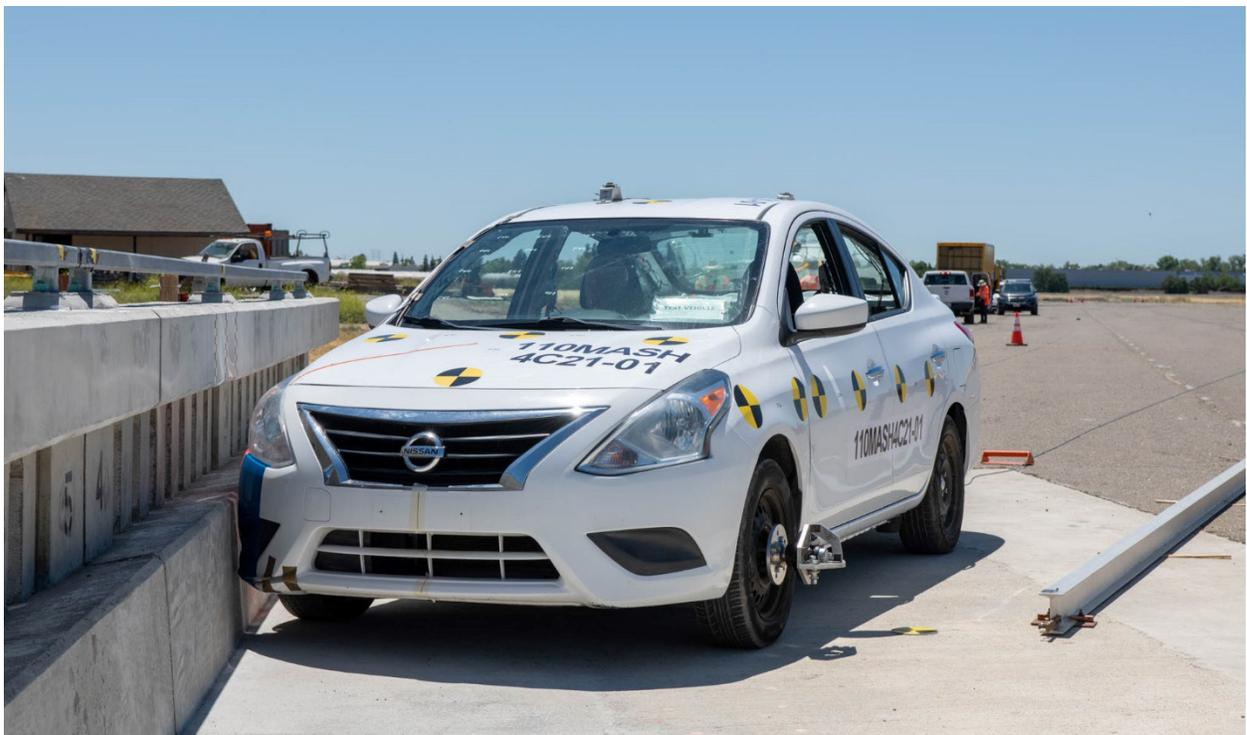
Figure 4-6 MASH 4-10 Test Vehicle at Impact Point
