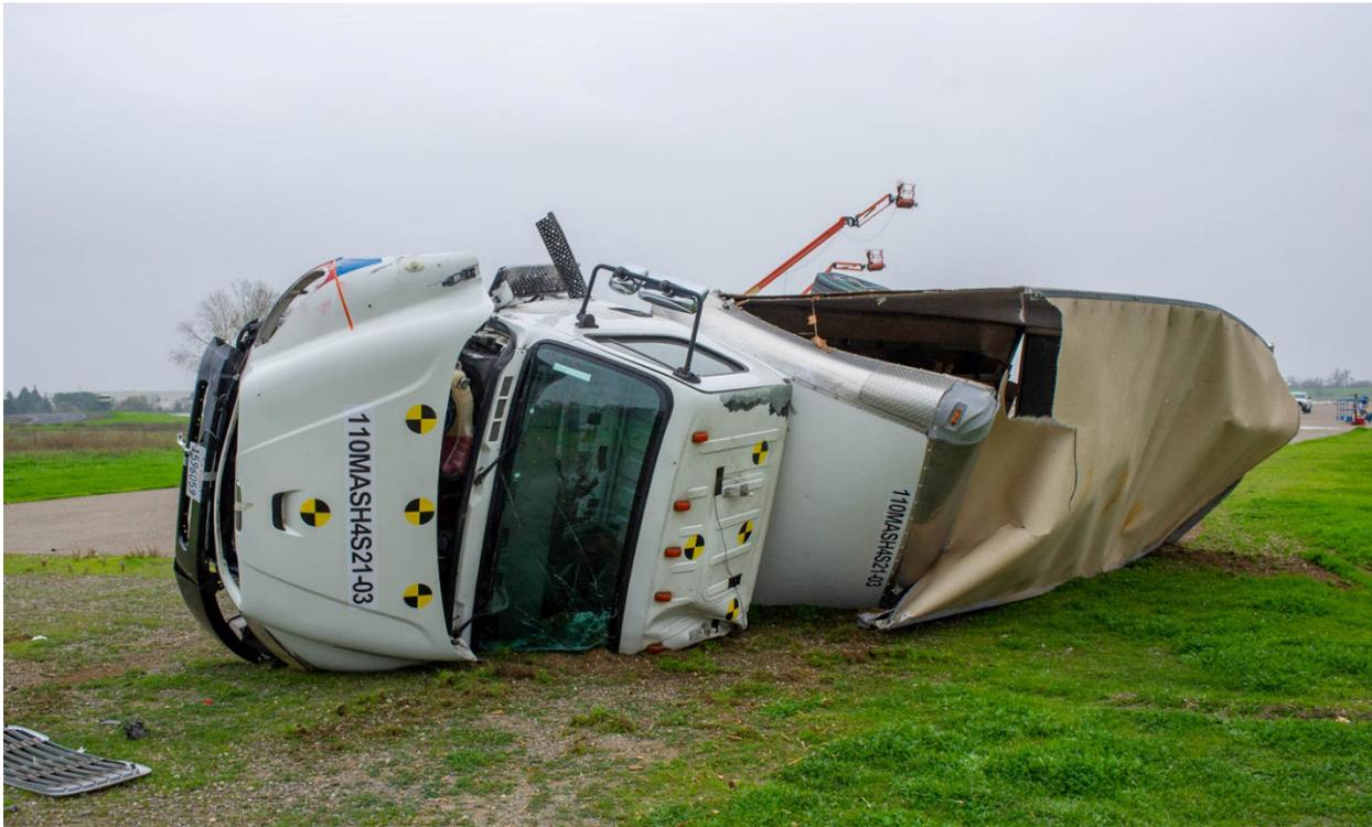
Figure 7-20 Test 4-12 Test Vehicle After Impact (front right)
