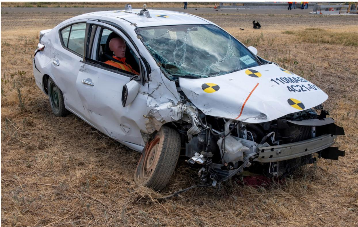
Figure 5-11 Test Vehicle Damage (front right)
