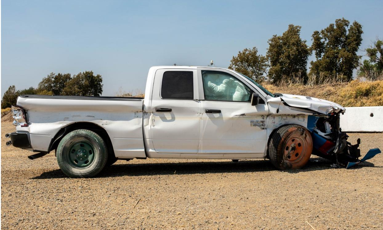
Figure 6-12 Test 4-11 Test Vehicle Damage (right)
