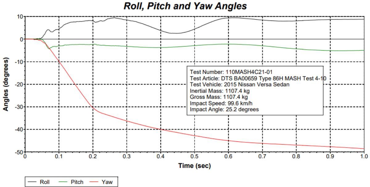
Figure 10-28 Test 4-10 Roll, Pitch, and Yaw Angles (DTS SLICE Micro TRAP BA00659)
