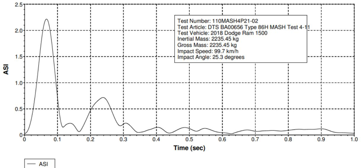
Figure 10-50 Test 4-11 Acceleration Severity Index (DTS SLICE Micro TRAP BA00656)
