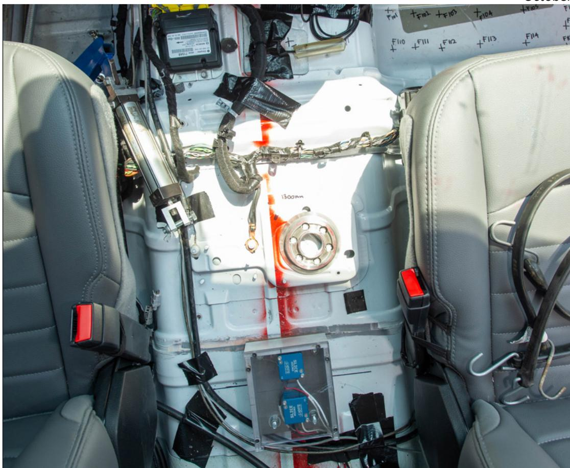
**Figure 10-4 Test 4-11 DTS SLICE Micro Mount Position in the Vehicle**
