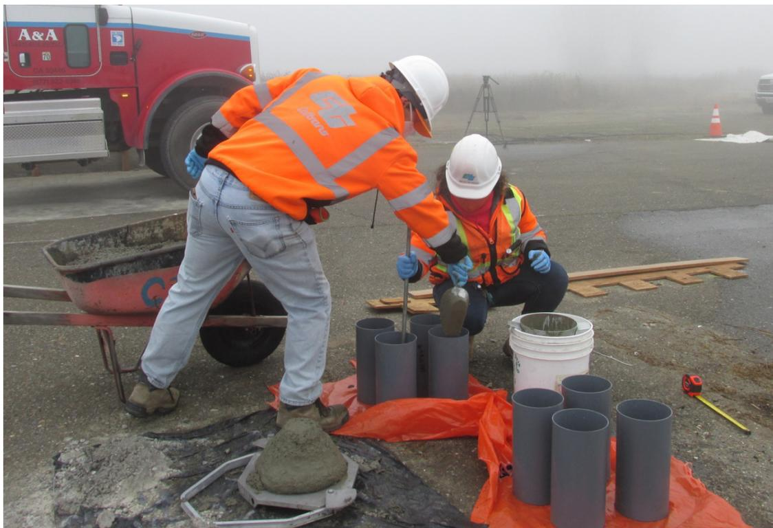
Figure 2-47 Concrete Sampling and Slump Test During the Post and Beam Pour by Caltrans Staff
