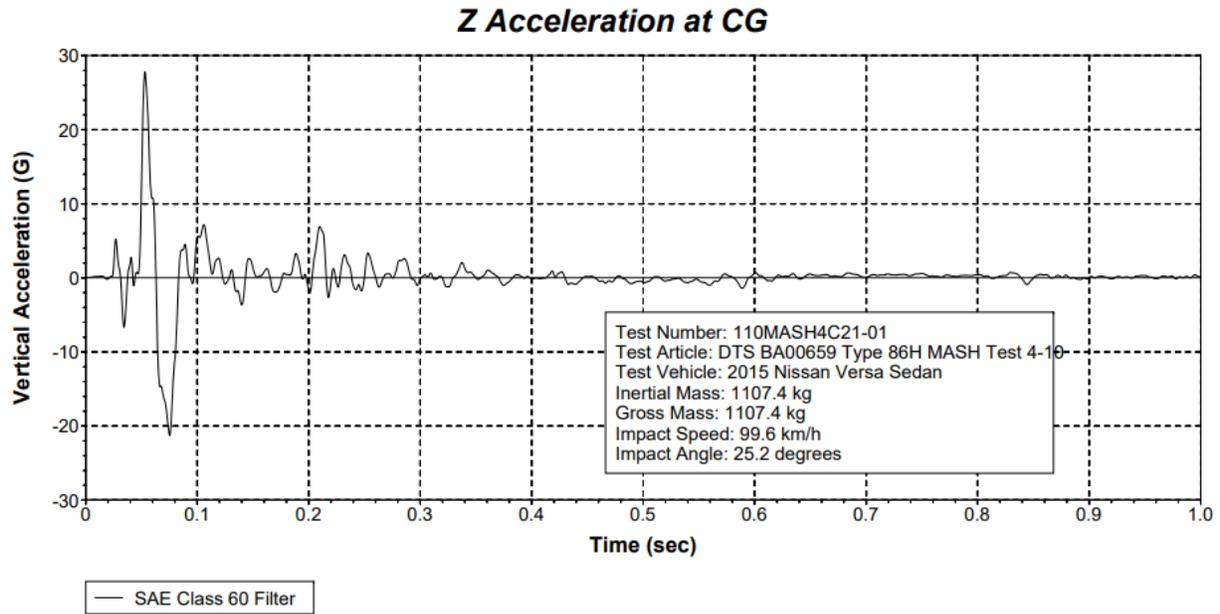
Figure 10-26 Test 4-10 Vertical Acceleration (DTS SLICE Micro TRAP BA00659)
