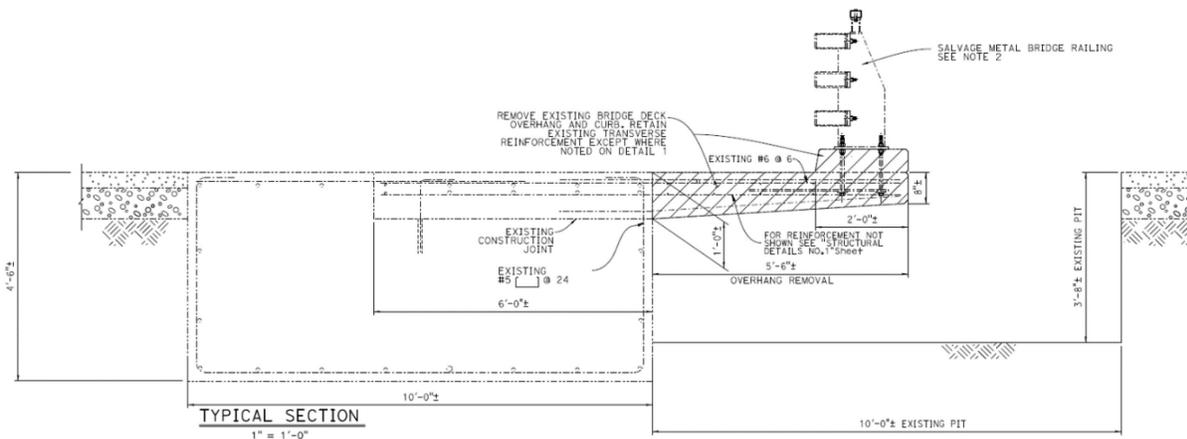
Figure 2-2 Cross Section of Existing Concrete Block and Overhang Removal
