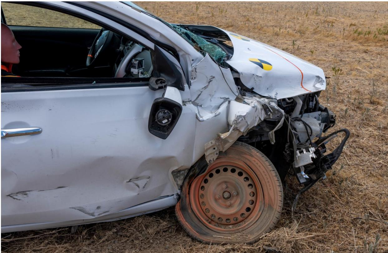
Figure 5-13 Test 4-10 Test Vehicle Damage (front right)
