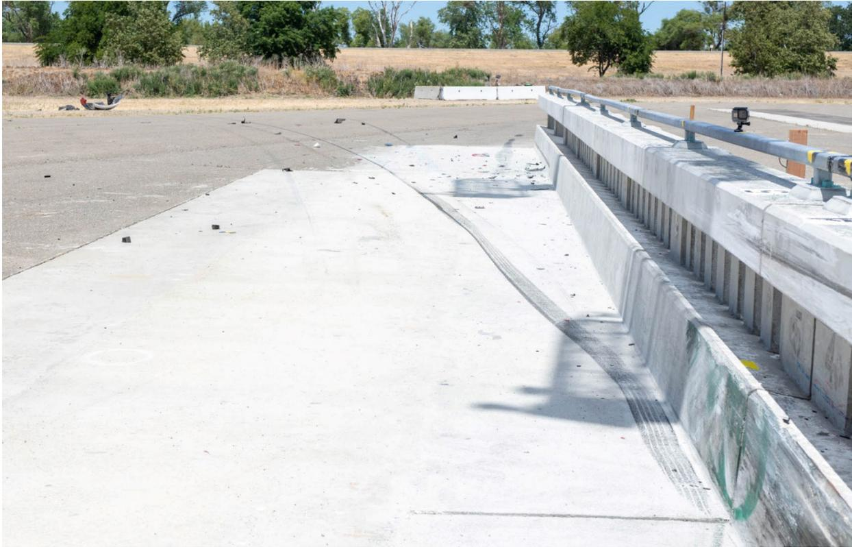
**Figure 5-9 Test 4-10 Tire Marks Post-Test (view from downstream)**
