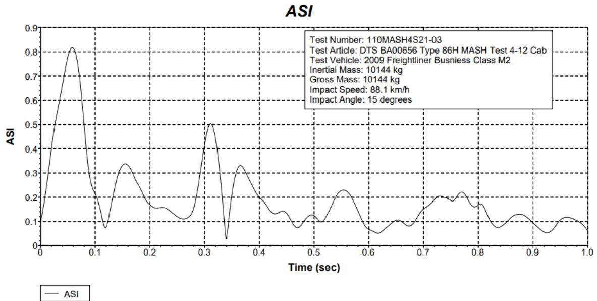
Figure 10-57 Test 4-12 Acceleration Severity Index (DTS SLICE Micro TRAP BA00656)
