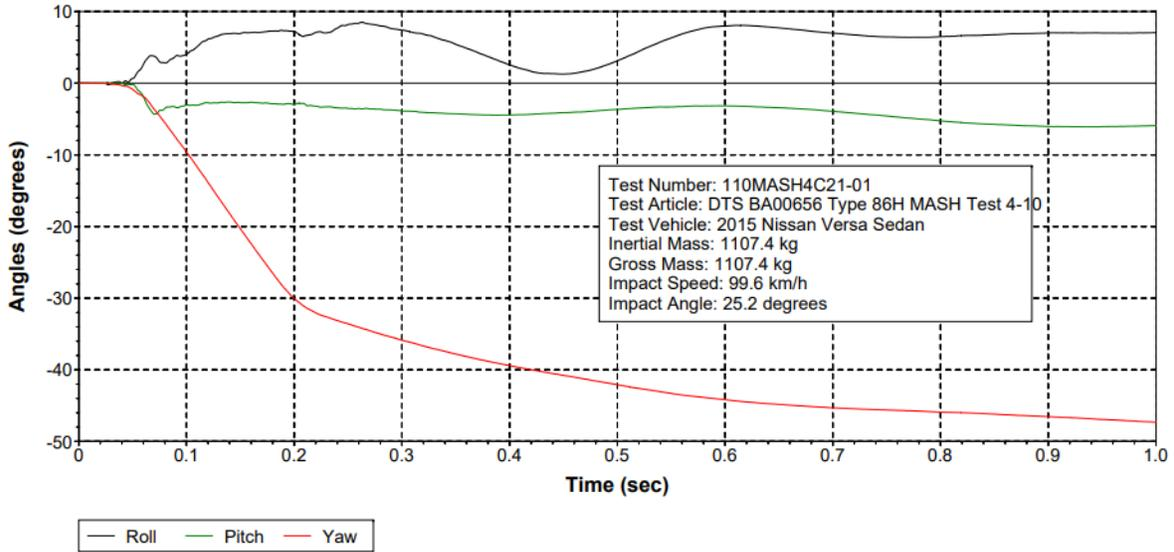
Figure 10-35 Test 4-10 Roll, Pitch, and Yaw Angles (DTS SLICE Micro TRAP BA00656)
