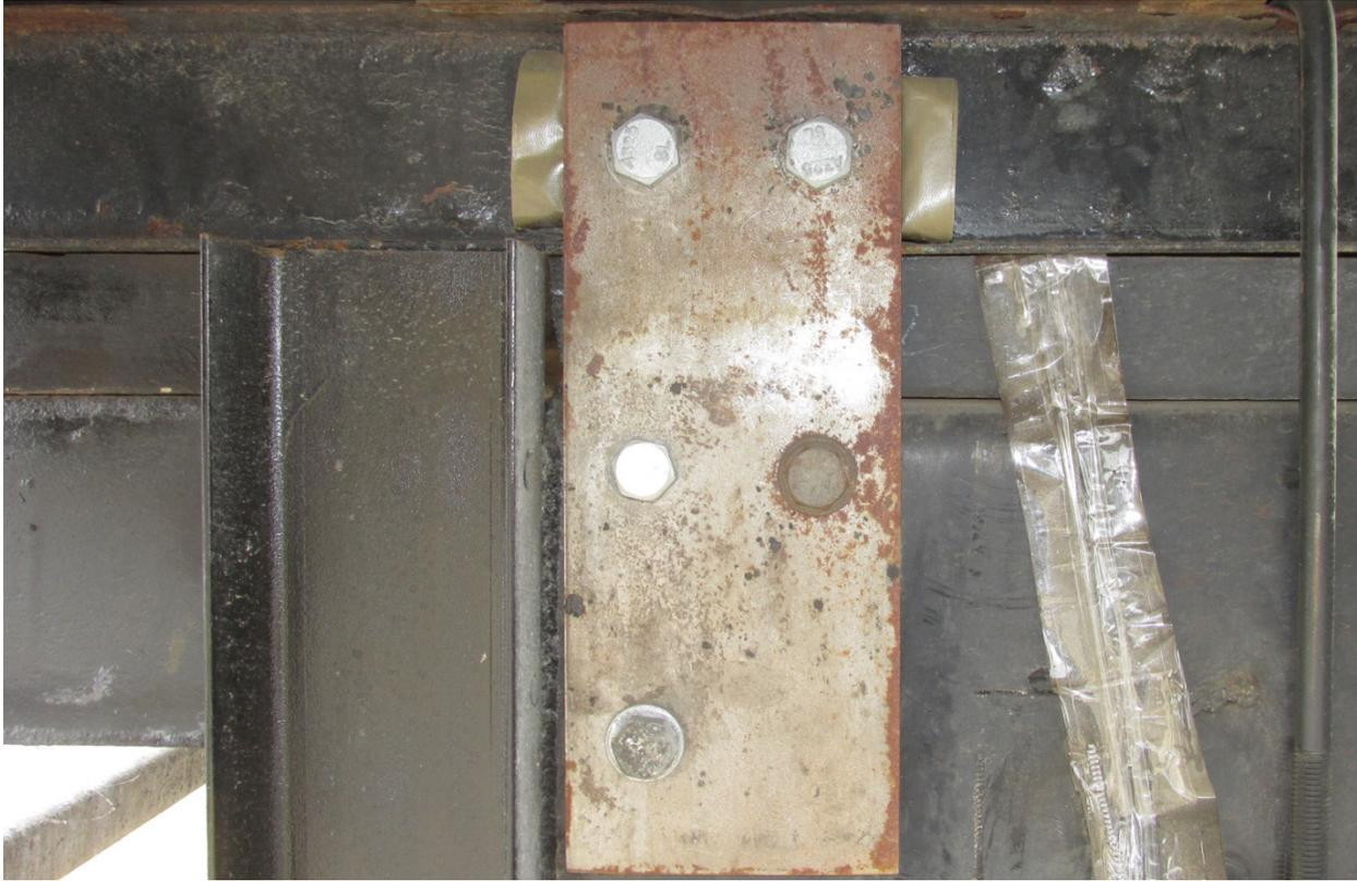
**Figure 7-24 Test 4-12 Rear Right Shear Plate After Impact**
