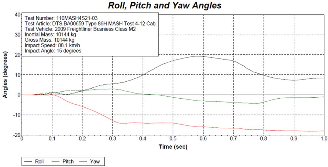
Figure 10-63 Test 4-12 Roll, Pitch, and Yaw Angles (DTS SLICE Micro TRAP BA00659)
