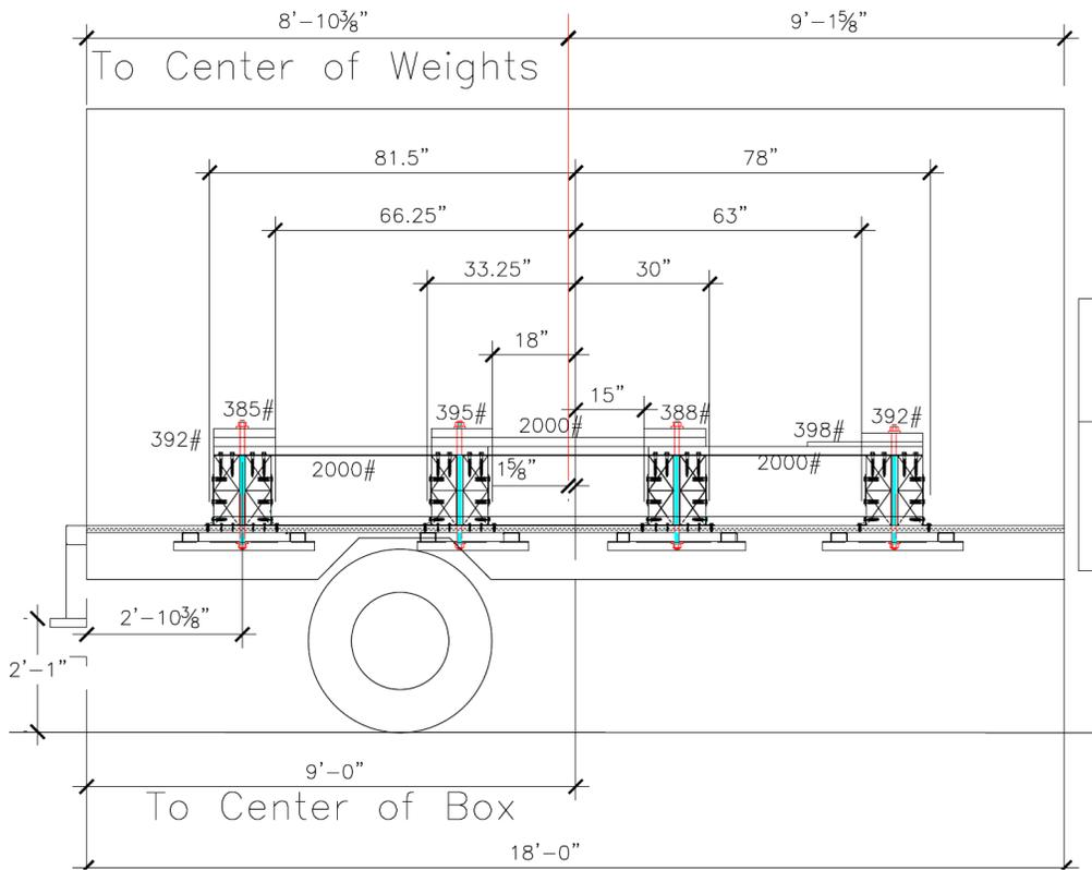
Figure 4-21 MASH 4-12 Side View Diagram of Test Vehicle Ballast in Cargo Box
