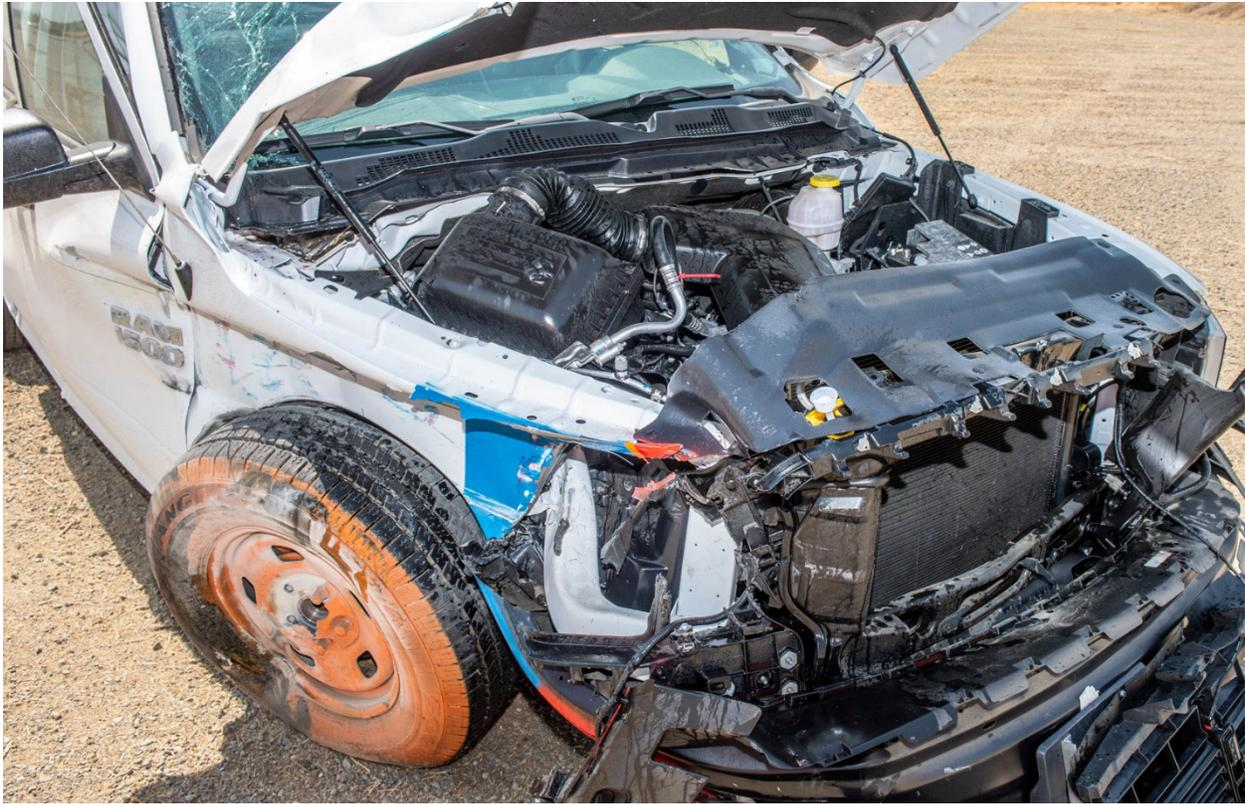
Figure 6-18 Test 4-11 Test Vehicle Damage front right with hood opened
