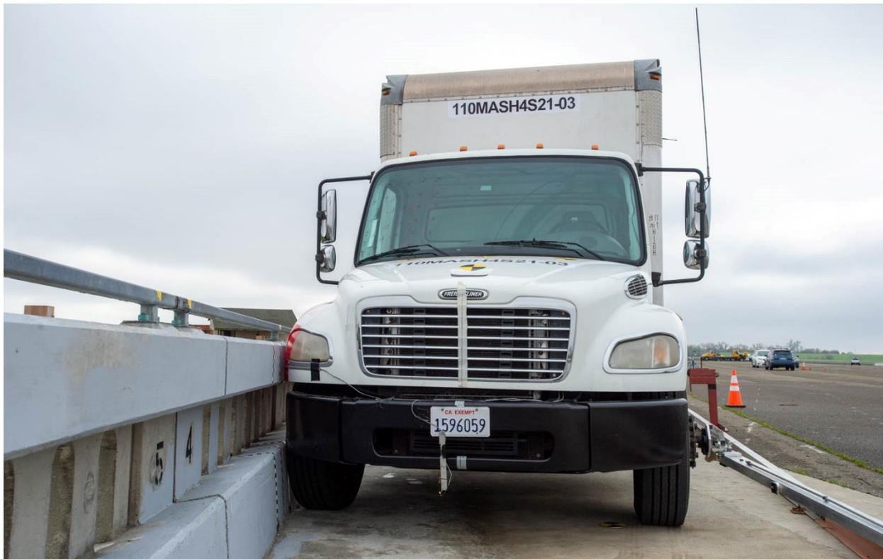
Figure 4-19 MASH 4-12 Test Vehicle at Impact Point
