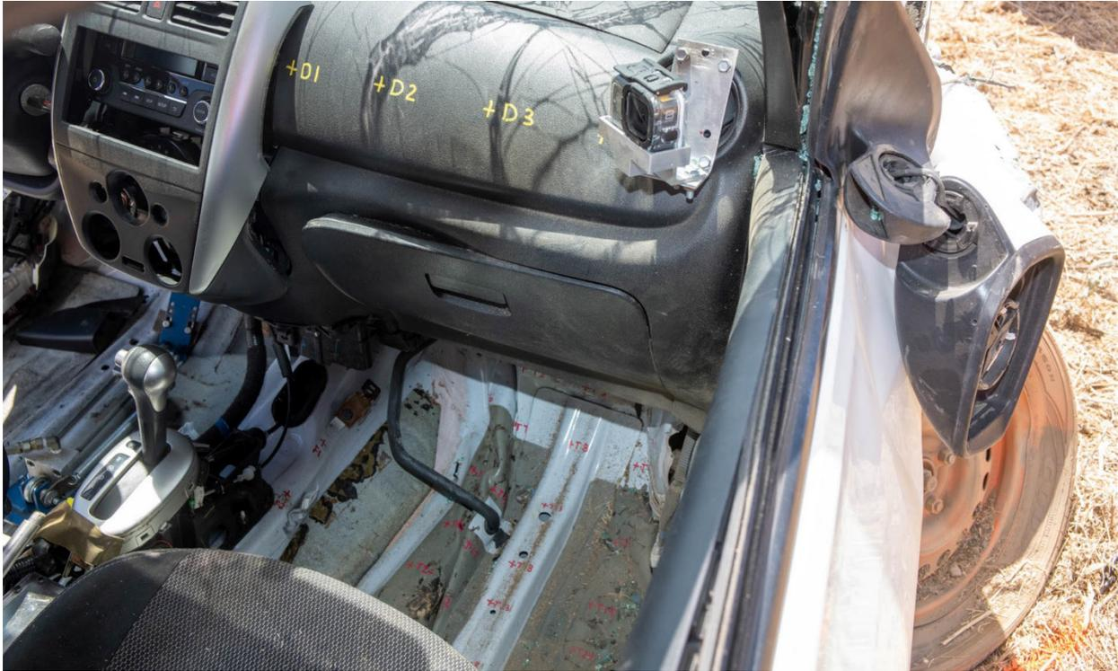
Figure 5-22 Test 4-10 Floorboard Deformation
