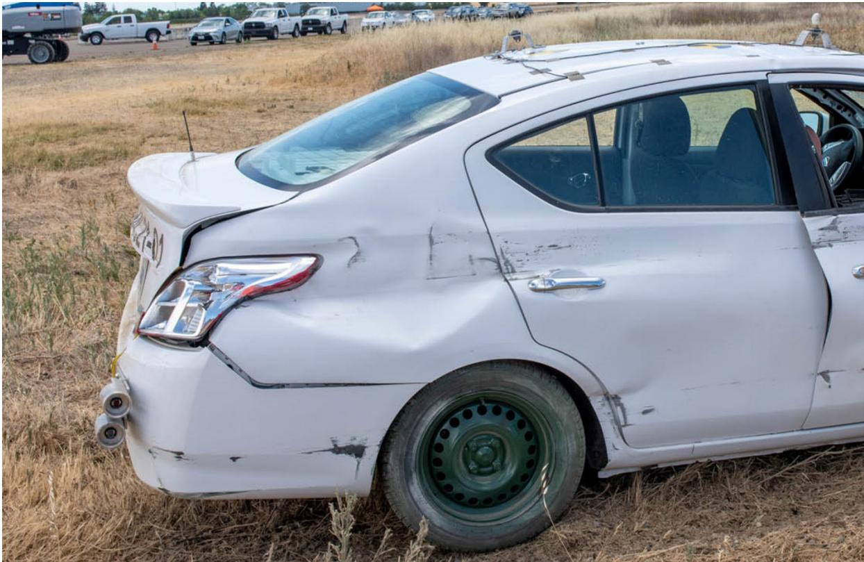
Figure 5-15 Test 4-10 Test Vehicle Damage (right rear)
