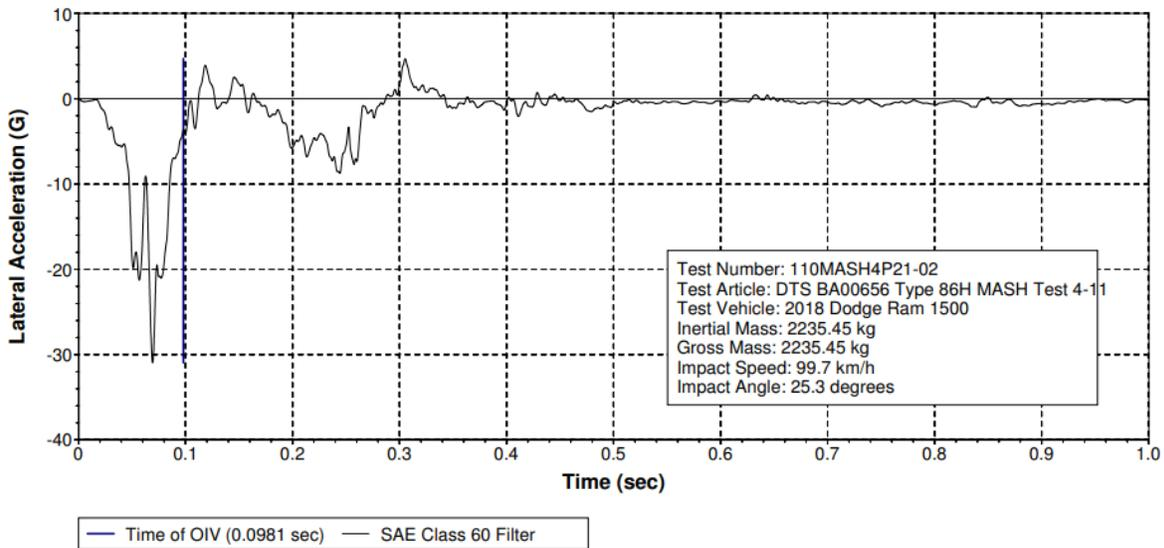
Figure 10-46 Test 4-11 Lateral Acceleration (DTS SLICE Micro TRAP BA00656)
