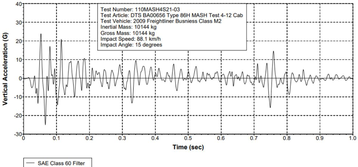
Figure 10-54 Test 4-12 Vertical Acceleration (DTS SLICE Micro TRAP BA00656)
