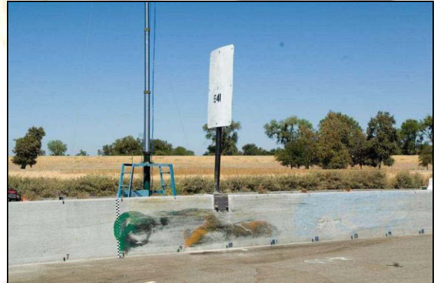
Figure 4 – Impact Area After Test
