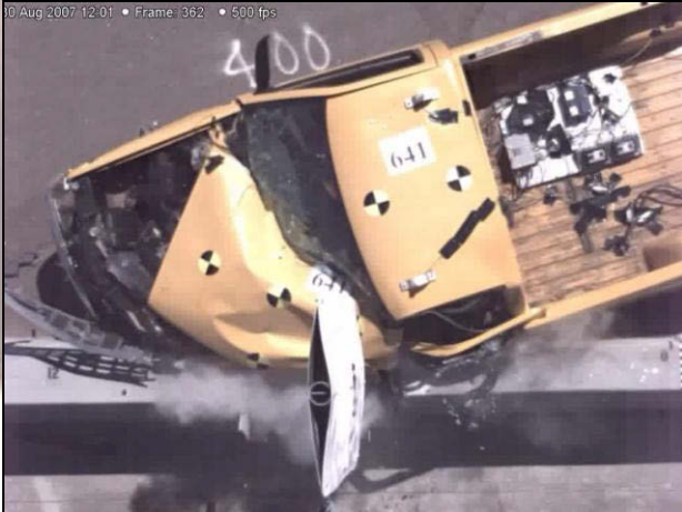
Figure 2 – Vehicle Impacting Barrier and Signpost
