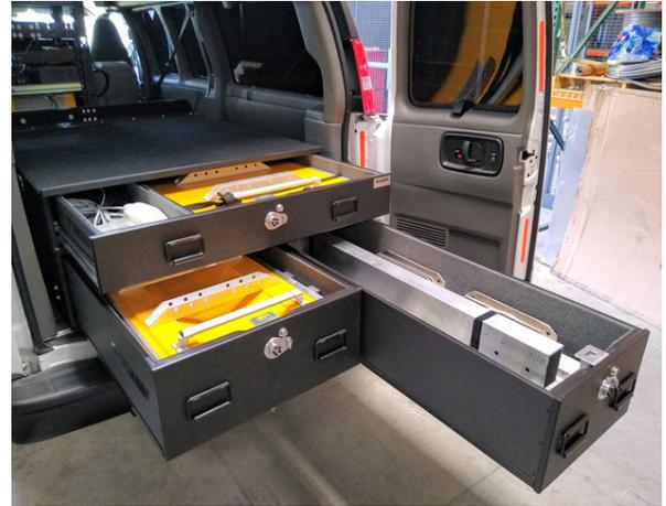
Figure 4: A lockable storage system mounted at the rear of the 3D vehicle. It provides secure storage and transportation for the 3D GPR antennas and sensor mount.
