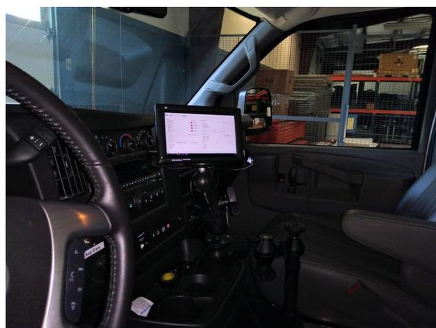
Figure 2: The driver's guidance display. It guides the driver to the proper location within the lane for complete and accurate data collection.
