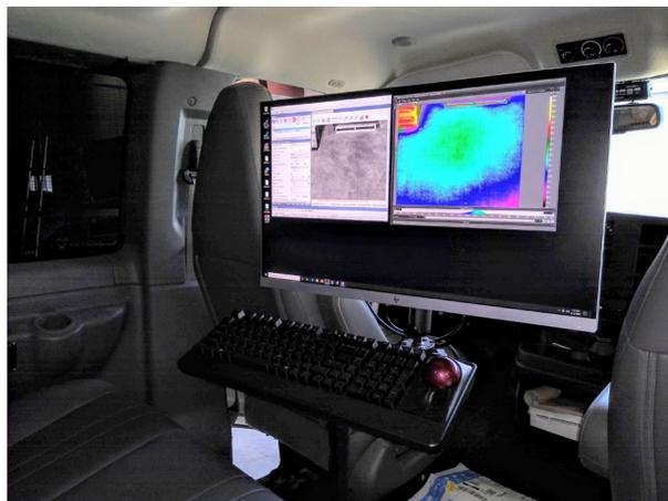
Figure 8: The 3D GPR operator's user interface. The interface enables the operator to monitor the proper functioning of sensors, cameras, and data collection.
