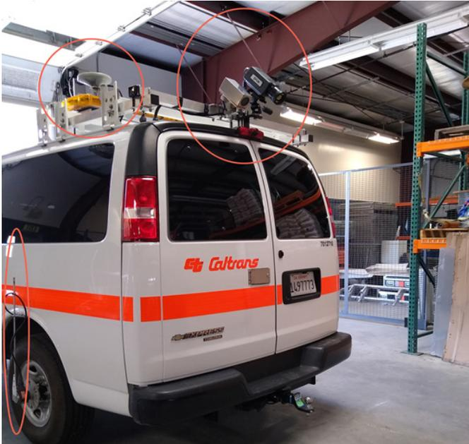
Figure 3: A rear view of Caltrans' 3D Radar vehicle. The dual GNSS antennas that provide accurate positioning are mounted near the center of the roof of the vehicle (a). Above the rear doors are the B/W camera (enclosed inside a stainless steel waterproof housing) and the FLIR IR Camera, both pointing towards the pavement (b). Mounted on the left rear wheel is the Distance Measurement Unit (DMI), which is connected to the Applanix GNSS/IMU system and GeoScope (c).
