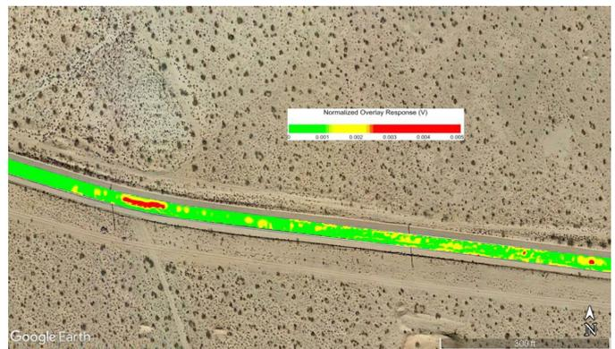
Image 5: A sample graphic of the Pavement Intralayer GPR Response. Intralayer GPR Response provides an indicator for overlay stripping or delamination.
