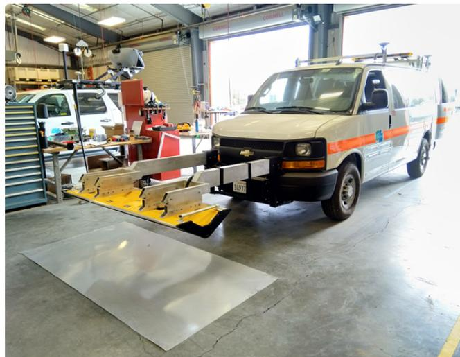
Figure 1: A frontal view of Caltrans' 3D Radar vehicle. The 3D-GPR antenna array (with a yellow top) is mounted on two racks at the front of the vehicle.
