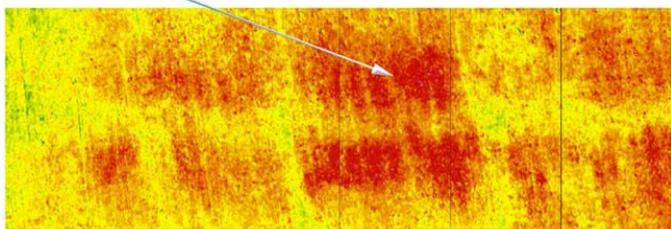
Image 7: A sample of a processed thermal image of a bridge deck where the color difference (red shade) can indicate delamination.
