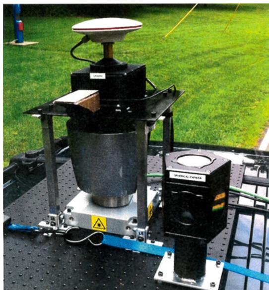
Image 1: Mapping Unit with GPS and LIDAR unit
