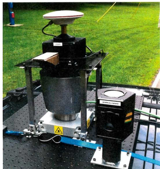
Image 1: Mapping Unit with GPS and LIDAR unit
