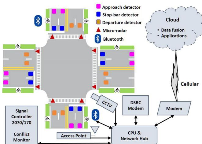
FIGURE 1: Schematic of reference intersection instrumentation
