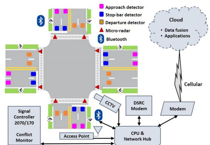
FIGURE 1: Schematic of reference intersection instrumentation
