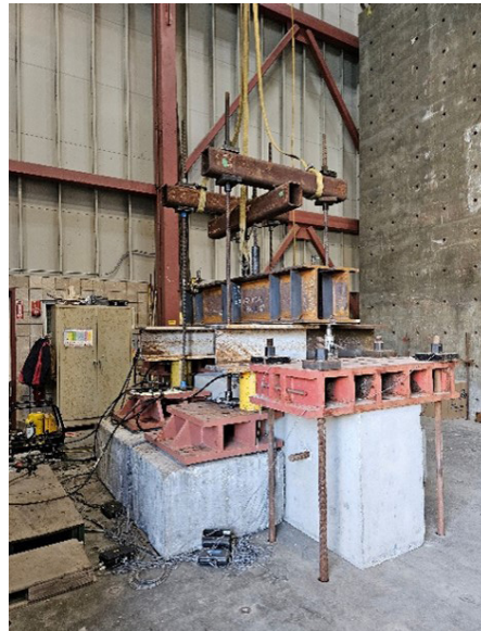
Image 1: Setup for a bar anchorage test
