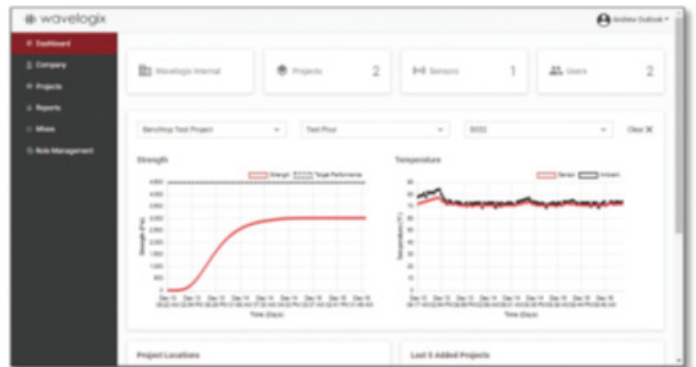
Image 2: Dashboard of REBEL concrete strength monitoring system.
