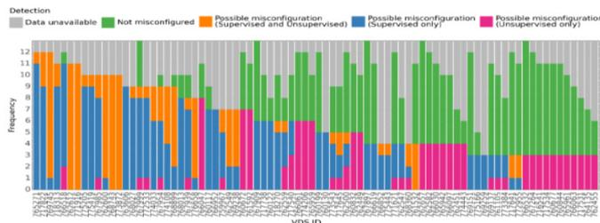
Image 2: Sorted frequency distribution of misconfigured sensor detections for quarterly analyses from 2018-Q1 to 2021-Q1, truncated to only sensors with at least two detections
