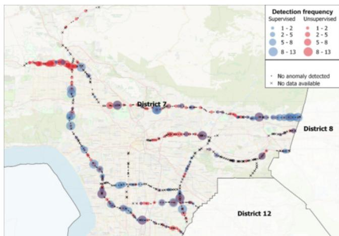
Image 1: Map of misconfiguration detection frequency in District 7 by unsupervised learning (red dots) and supervised learning (blue dots) where larger dots indicate more detections per sensor
