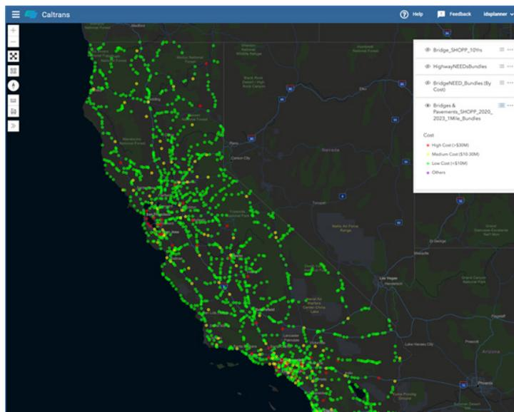
Image 3: Example of cross-asset treatment bundles for bridge and pavement treatments recommended by the SHOPP 10-year planning scenario
