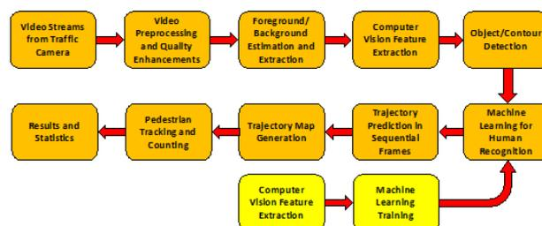
Image 1: End-to-end system architecture
