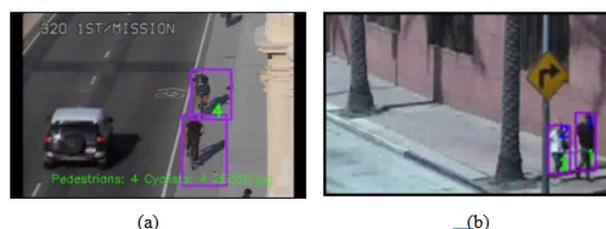
Image 2: System results on real-time traffic video streams: (a) Bicyclist tracking and counting, (b) Pedestrian tracking and counting
