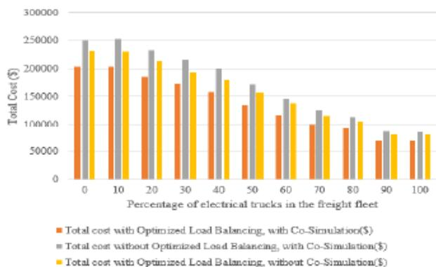
Image 2: Comparison with cases without optimized load balancing or co-simulation
