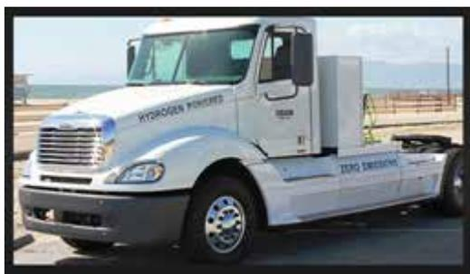
Image 2: A Fuel-cell Powered Heavy-duty Truck
