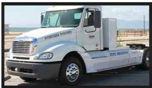
Image 2: A Fuel-cell Powered Heavy-duty Truck
