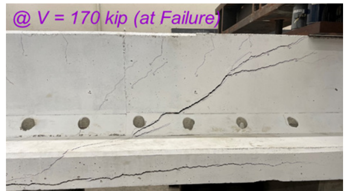
Image 2: Failure of control specimen (Phase I).
