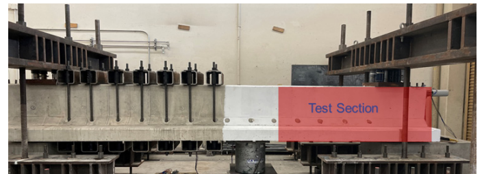
Image 1: Test setup enabling two tests per specimen.
