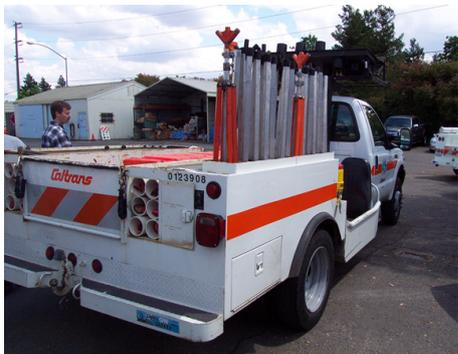
Image 1: Typical Caltrans cone body truck with 80 cones
