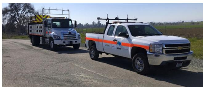
Image 4: The Caltrans ATMA performance testing system
