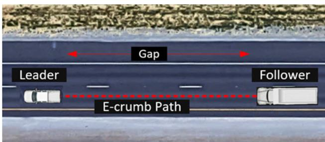
Image 2: Autonomous E-crumb path guidance
