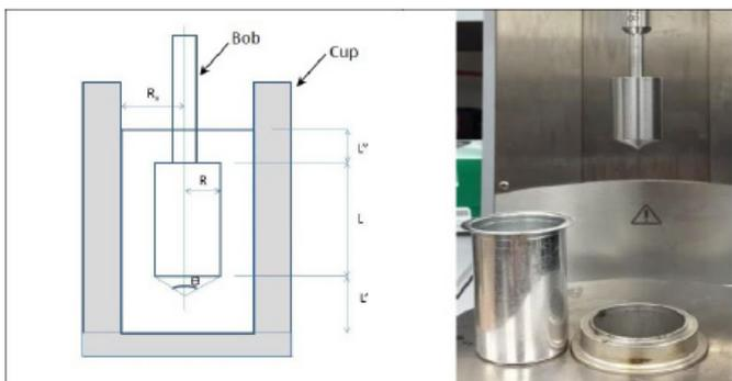
Image 1: Concentric cylinder geometry
