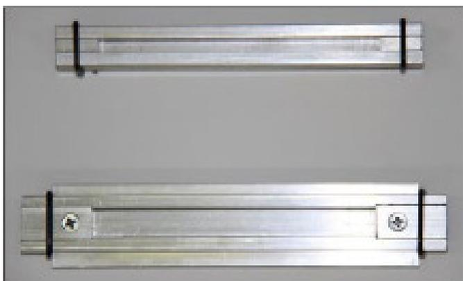
Image 2: Standard (top) and modified (bottom) BBR specimen mold configurations
