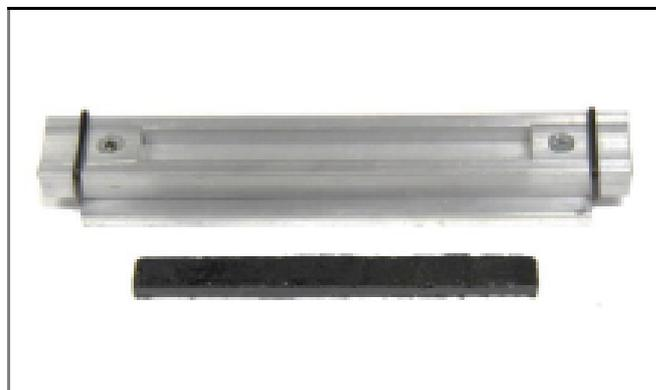
Image 3: Modified mold configuration and beam specimen
