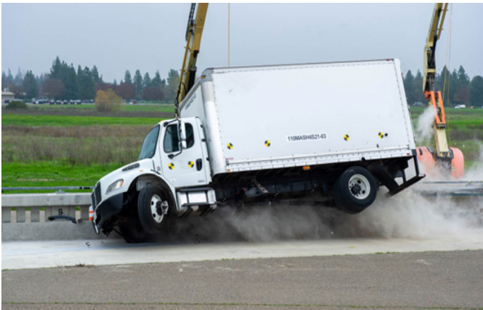
Image 5: A 22,000 pound single-unit truck impacting at 56 mph and 15°.
