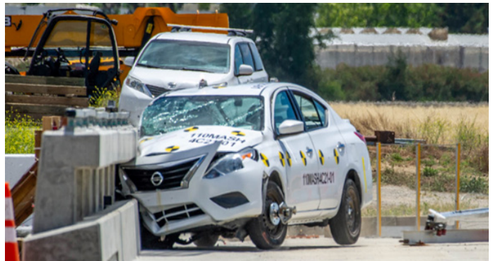
Image 3: A 2,420 pound small car impacting at 62 miles per hour (mph) and 25°.
