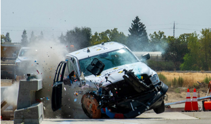
Image 4: A 5,000 pound pickup truck impacting at 62 mph and 25°.
