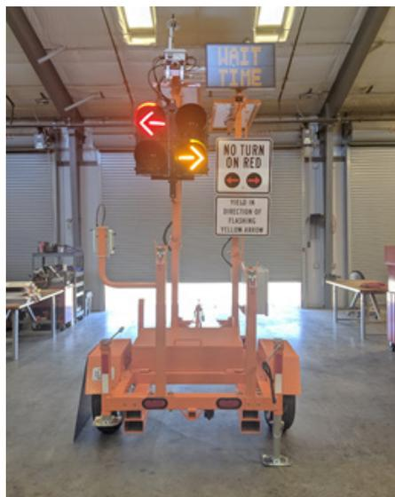
Figure: Picture of Driveway Management Unit from Superior Traffic Services.
