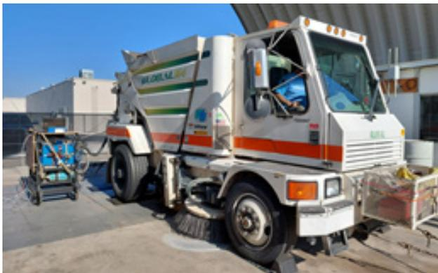
Image 2: Chassis dynamometer emission testing of Caltrans diesel street sweeper.
