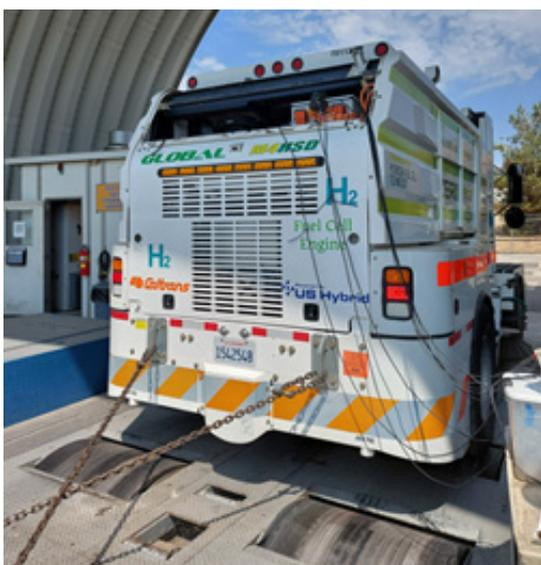
Image 3: Chassis dynamometer emission testing of Caltrans HFC street sweeper.
