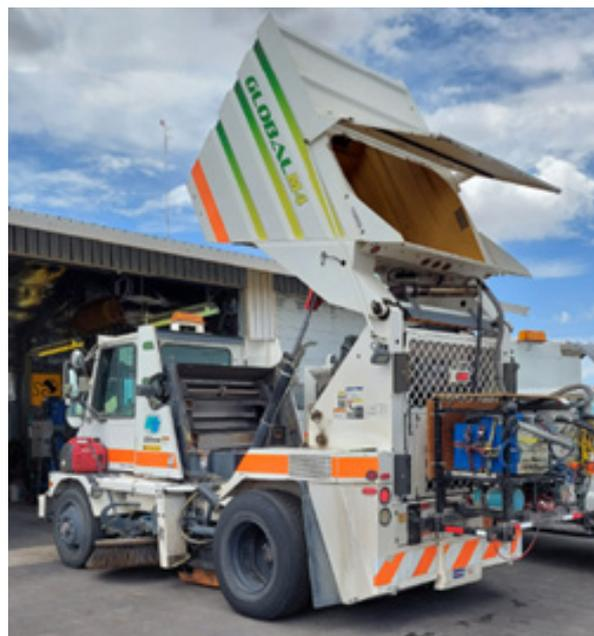
Image 1: PEMS instrumentation installed on Caltrans diesel street sweeper.
