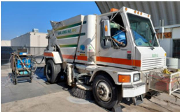
Image 2: Chassis dynamometer emission testing of Caltrans diesel street sweeper.
